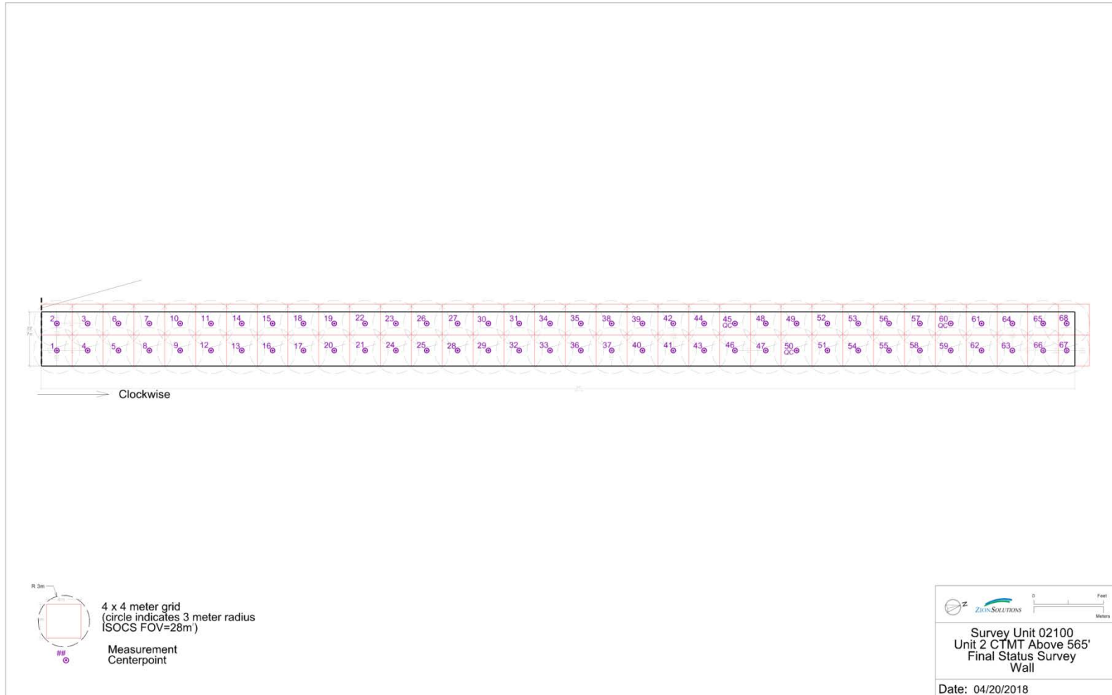
Figure 13 - Unit 2 Containment Above 565 foot Elevation FSS Wall Measurement Locations
