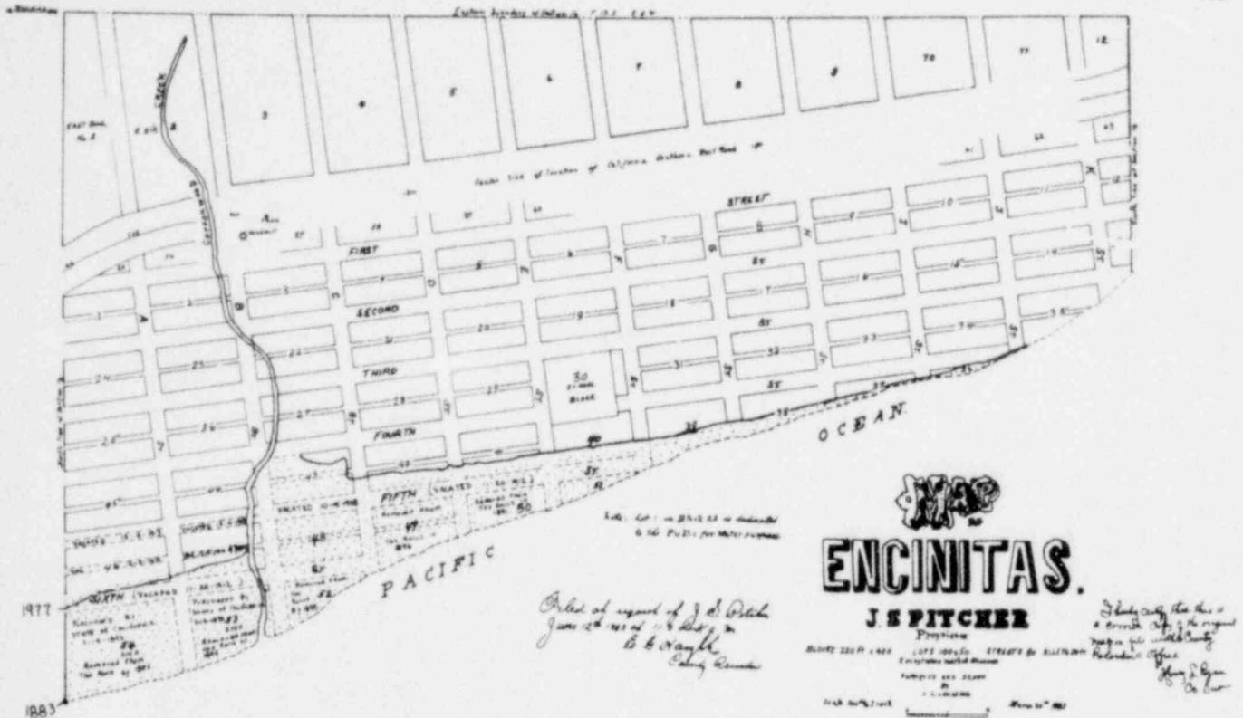
Figure 2. Town plat map of Encinitas, 1883. Apparent land loss is stippled. Solid line is the approximate present-day bluff top; dashed line (1883) may be either the former bluff top or shoreline. Several blocks of real estate were removed from county tax rolls before 1900. Map is an enhanced copy of San Diego County Recorders Subdivision Map #148, filed on June 12, 1883.
