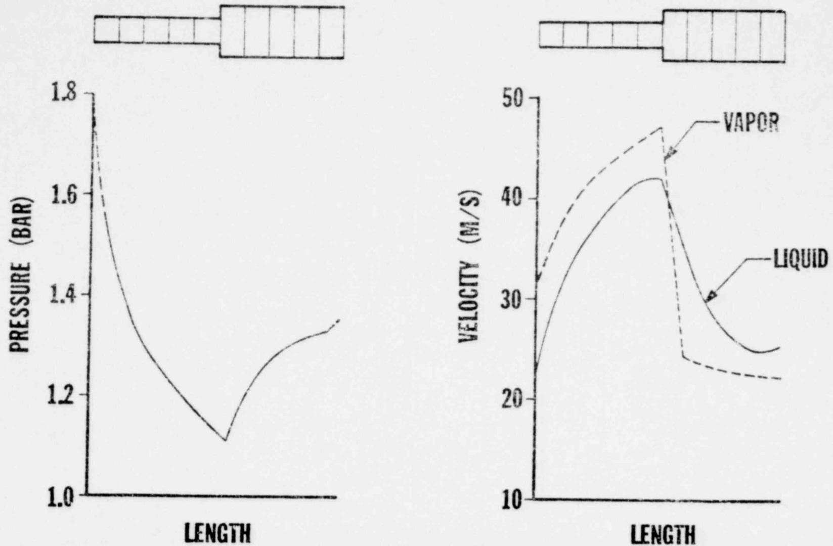
Fig. 16 Pressure and velocity variation in coupled one-dimensional regions showing pressure decrease due to flow velocities and corresponding separated flow effects.
