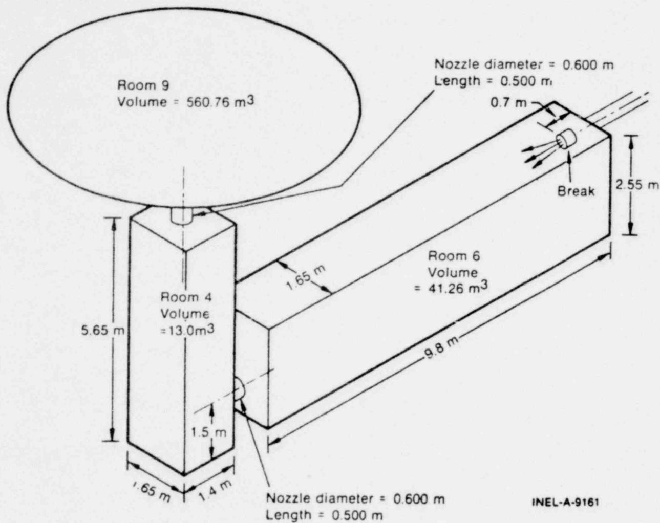
Fig. 26 Configuration for Sample Problem 7 which simulates a primary coolant pipe break into the first in a series of interconnected rooms.
