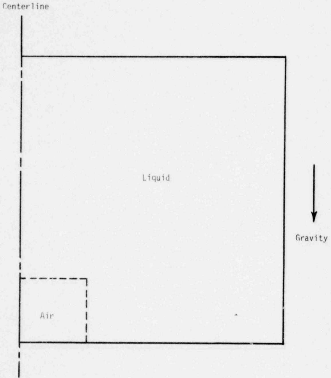
Fig. 1 Initial configuration for Sample Problem 1 before the air bubble has risen to the top of the liquid.
