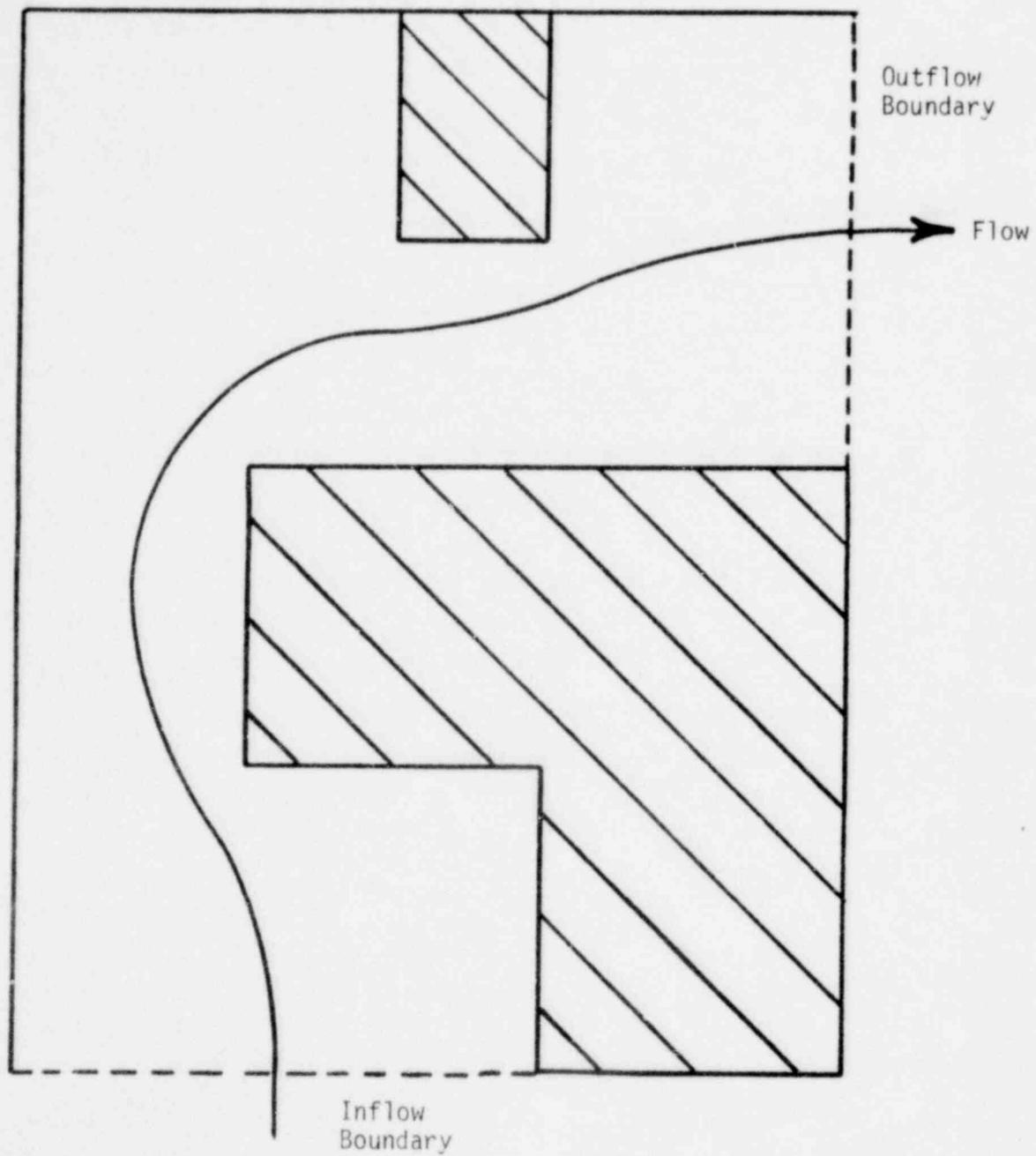
Fig. 7 Configuration for Sample Problem 2 a typical containment subcompartment problem, modeled with obstacle cells and inflow and outflow boundaries.
