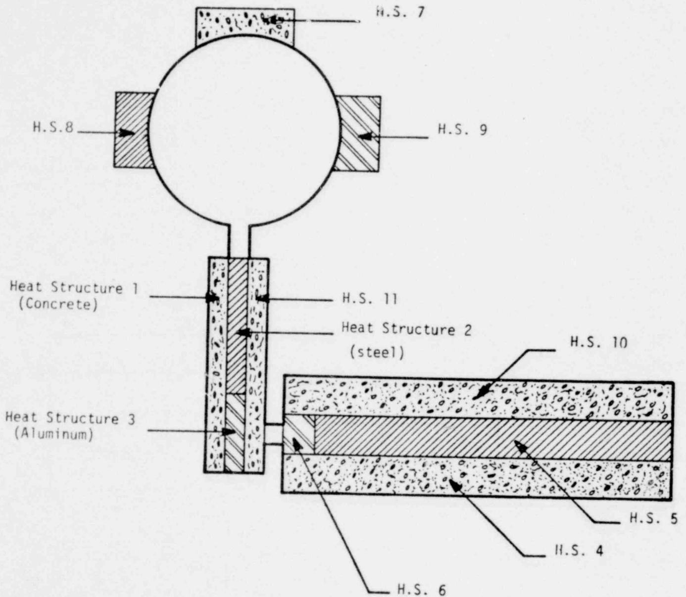
Fig. 28 Heat structure arrangement for Sample Problem 7 showing location of each material present.
