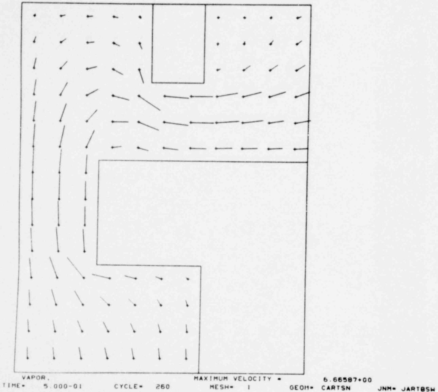
Fig. 9 Vapor velocity vector plot for Sample Problem 2 showing the flow diversion caused by the obstacles and the increase in velocities through the constricted areas.
