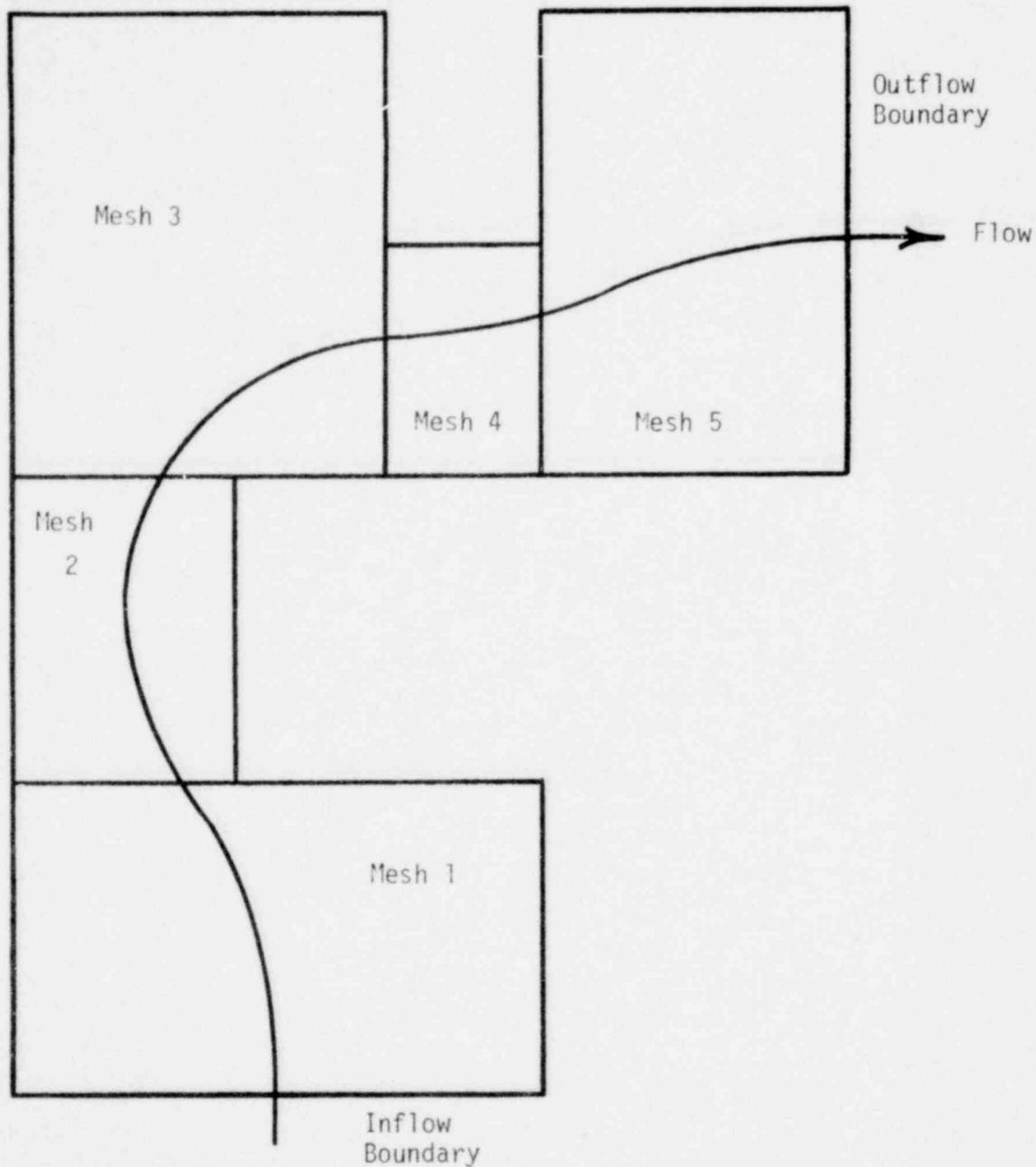
Fig. 11 Configuration for Sample Problem 3, a typical containment subcompartment problem, modeled by coupling a series of Eulerian regions.
