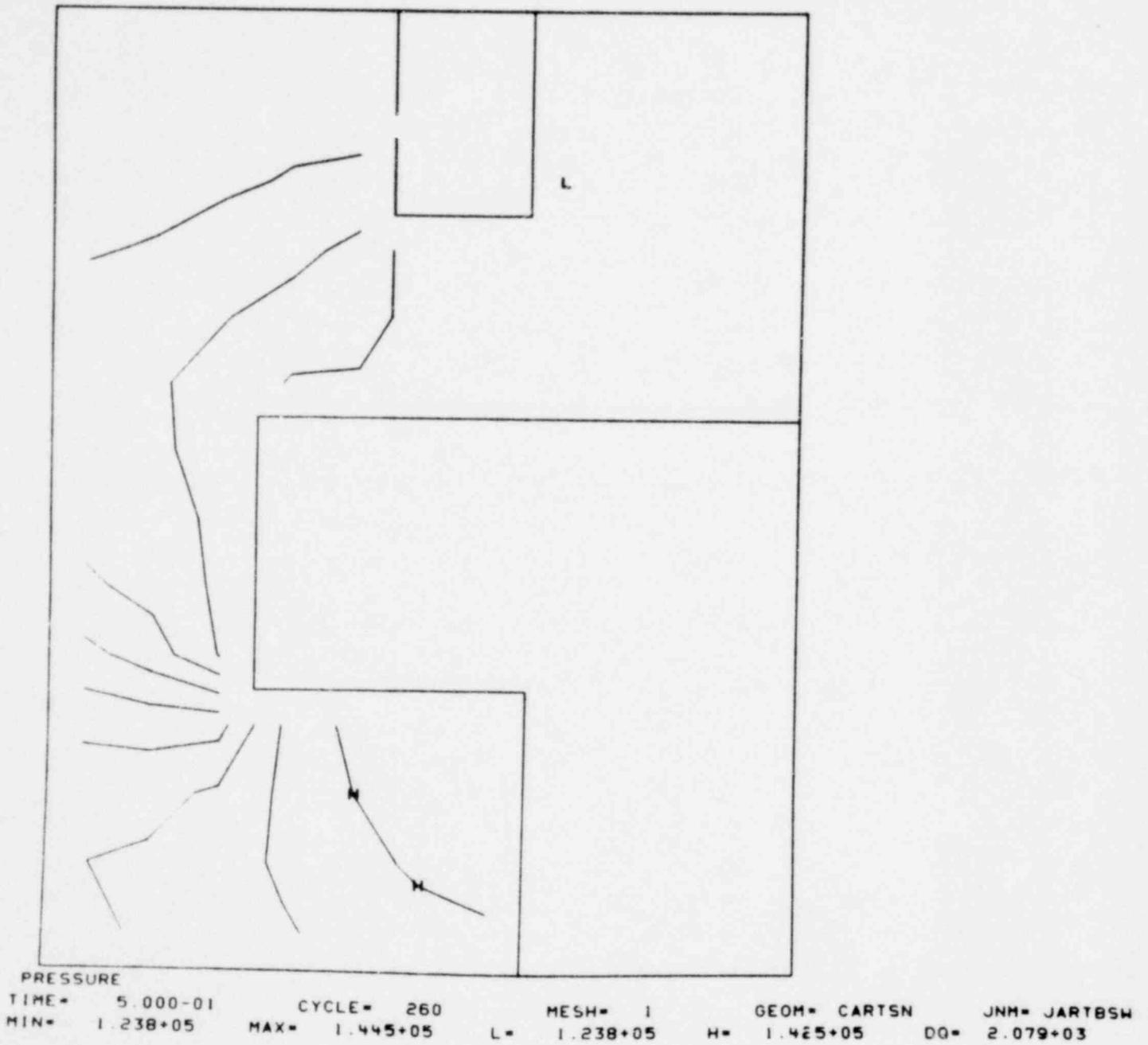
Fig. 10 Contour plot for Sample Problem 2 showing variations in the pressures resulting from velocity changes.
