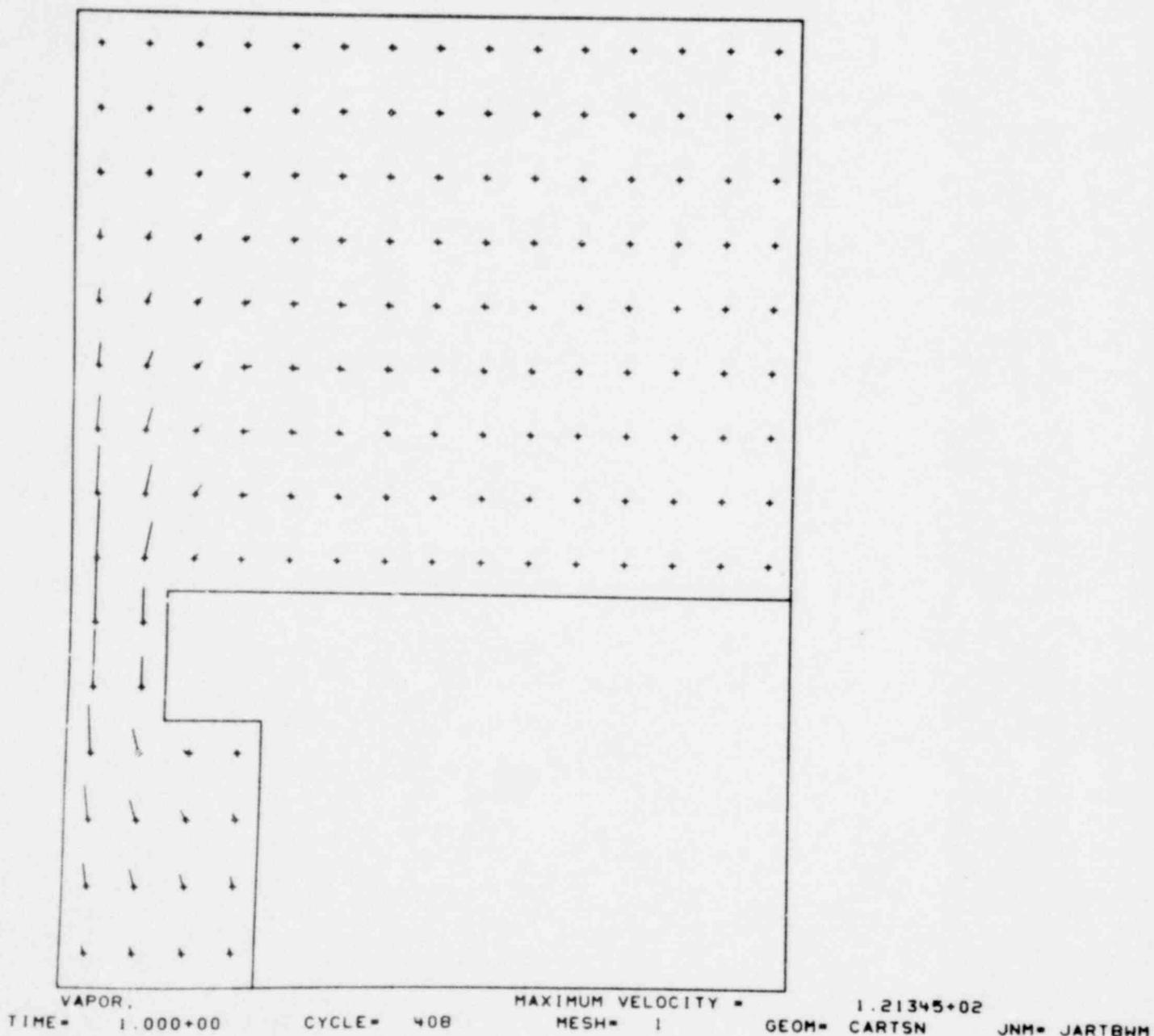
Fig. 19 Vapor velocities for Sample Problem 5 increase in the constricted area and stagnate in the large upper compartment.
