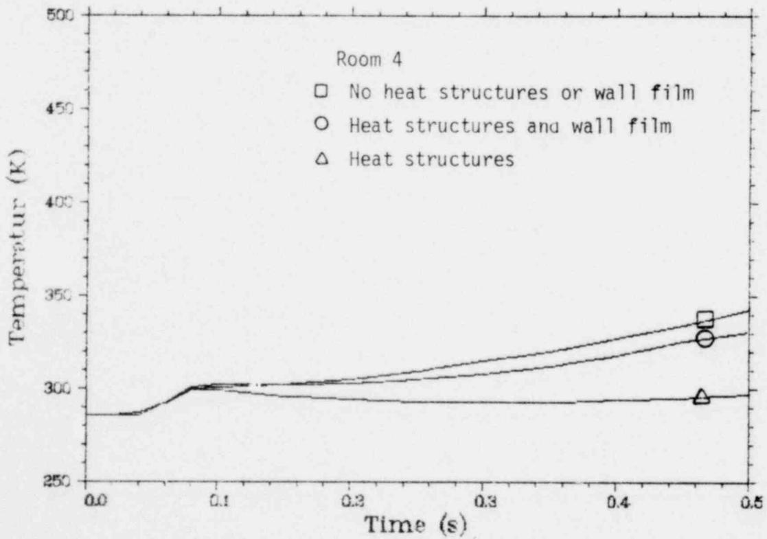
Fig. 31 Effects of wall film and heat structure modeling on temperatures calculated near the centers of Rooms 6 and 4.
