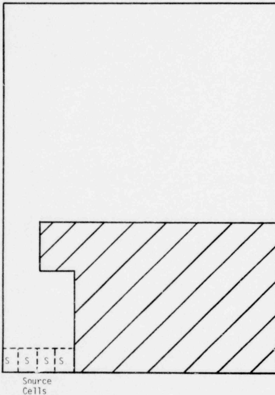
Fig. 17 Configuration for Sample Problem 5 demonstrating the use of source cells to introduce a steam flow into a two-compartment containment.
