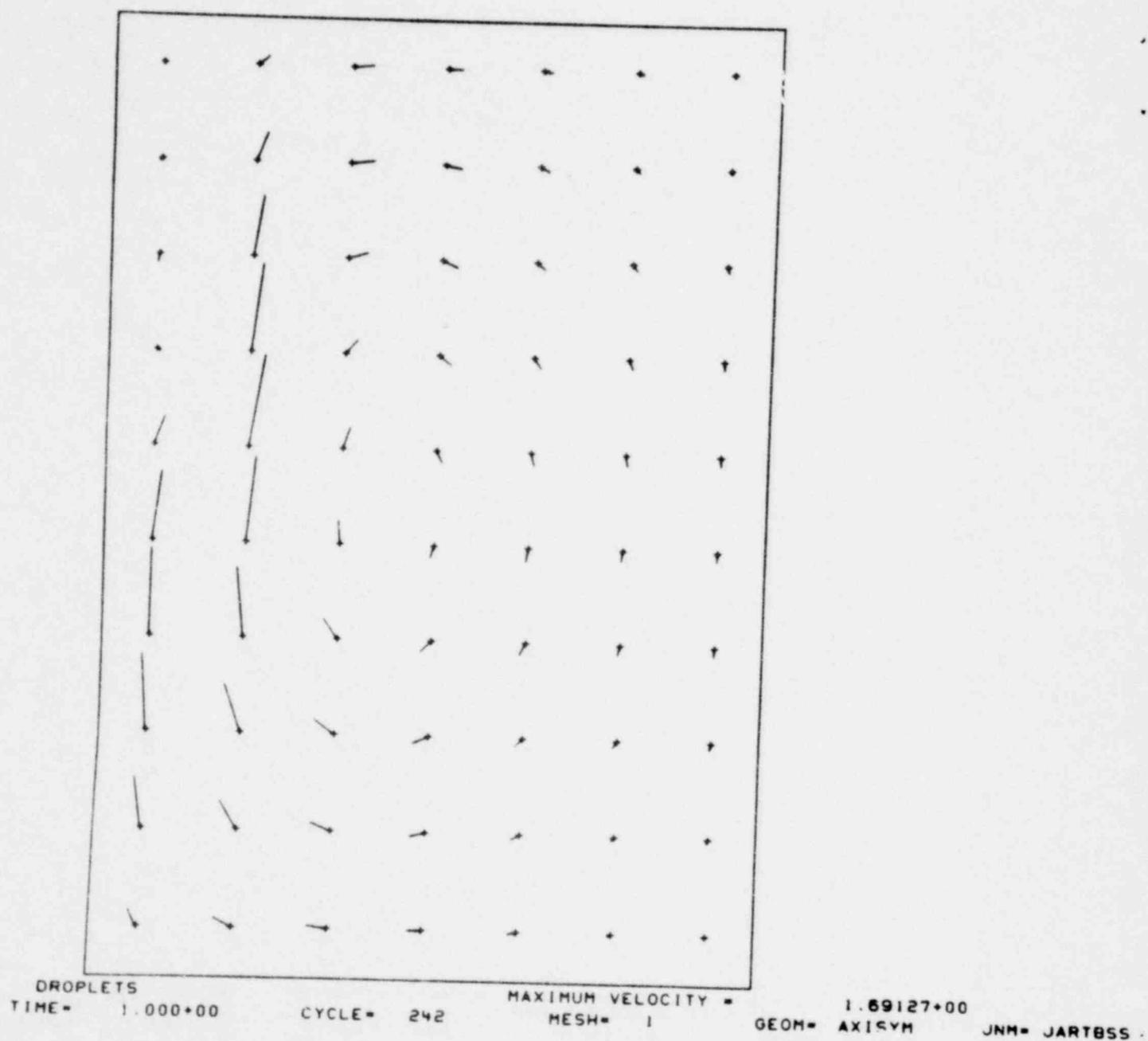
Fig. 4 Velocity vector plot for Sample Problem 1 illustrating how convection currents are produced in the liquid by the rising air bubble.
