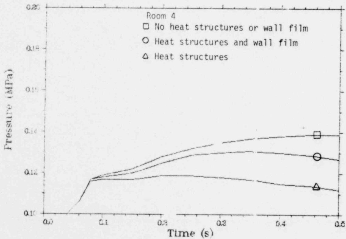
Fig. 30 Effects of wall film and heat structure modeling on pressures calculated near the centers of Rooms 6 and 4.
