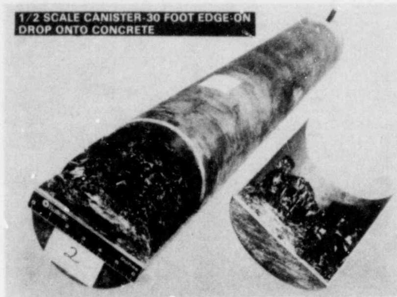
FIGURE 21. Half-Scale Canister After Impact
