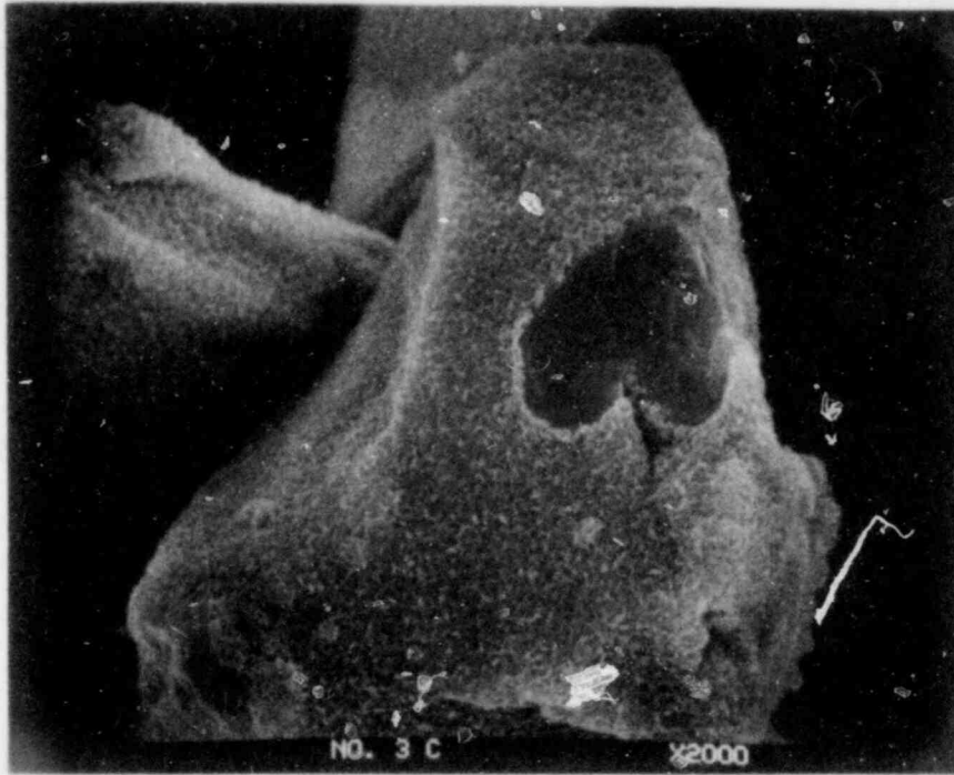
Figure 9. Silt-sized grains of basaltic glass with overgrowth of clay minerals.
