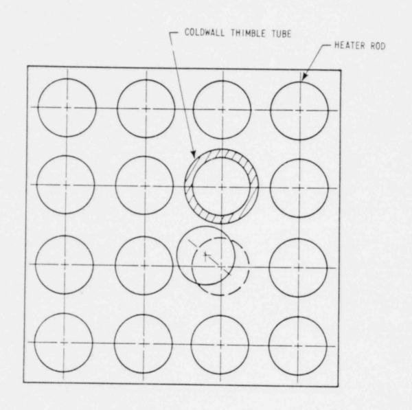
Figure 1 Partial Rod Bow Test Section, 85 Percent Closure
