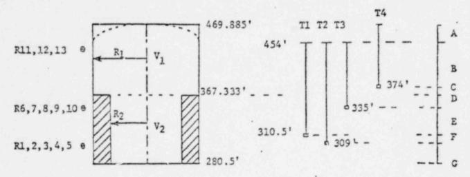
$$V = V_1 + V_2 = 2.1 \times 10^6 \text{ cu.ft.}, R_1 = 65'$$
