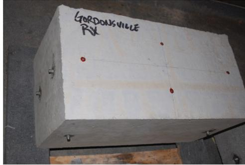
Figure 2.23: Concrete expansion block tested by Prof. E. Giannini
