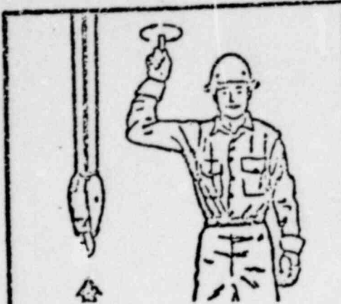
HOIST. With forearm vertical, forefinger point up, move hand in small horizontal circle.
