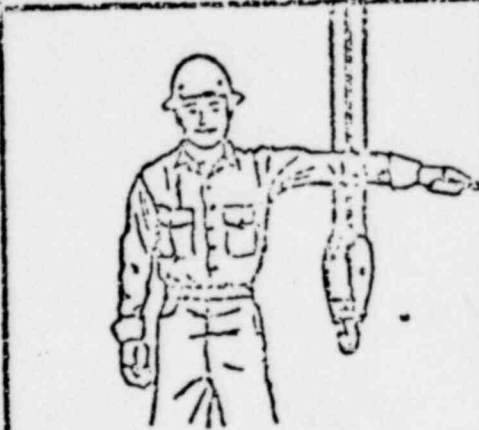
STOP. Arm extended, palm down, hold position rigidly.
