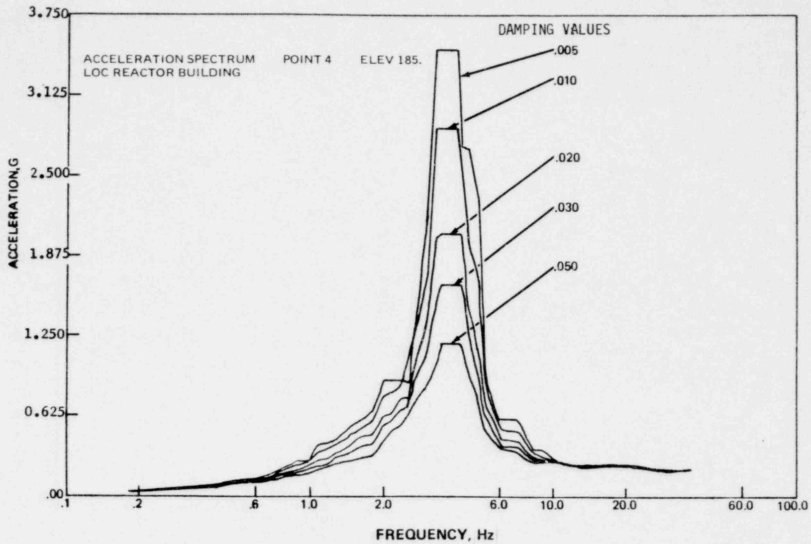
Figure 4-3 Reactor Building East-West OBE CE 921 Analysis
