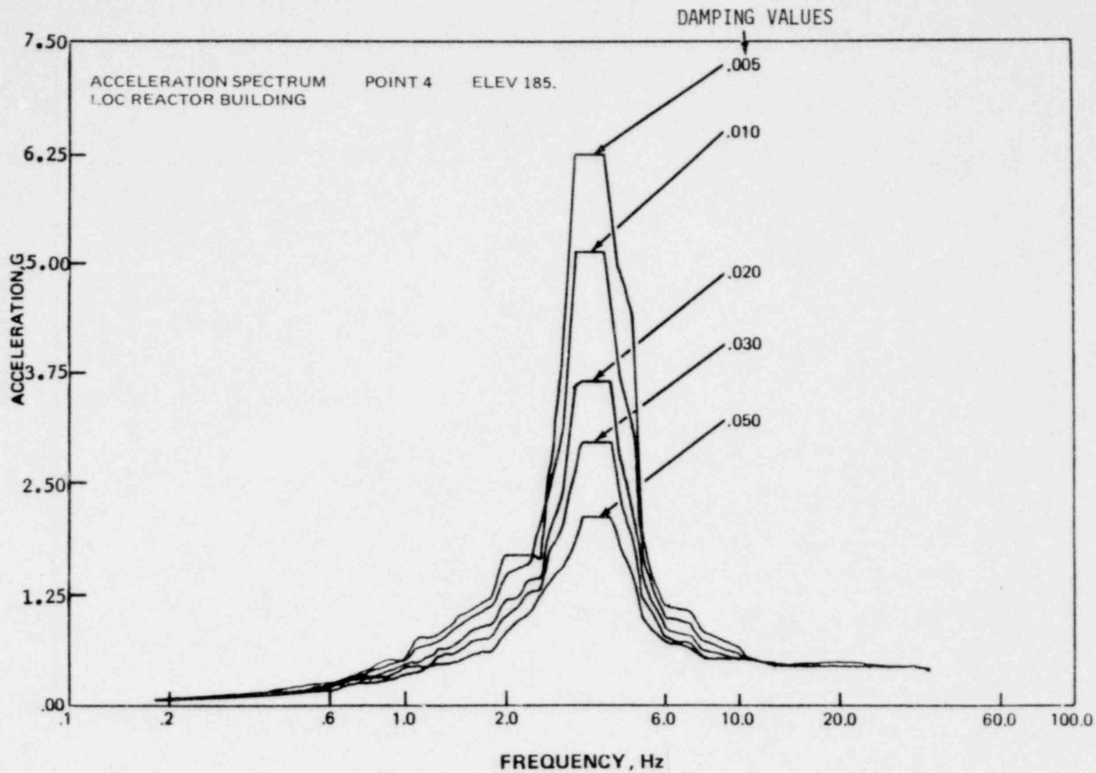
Figure 4-4 Reactor Building East-West SSE CE 921 Analysis
