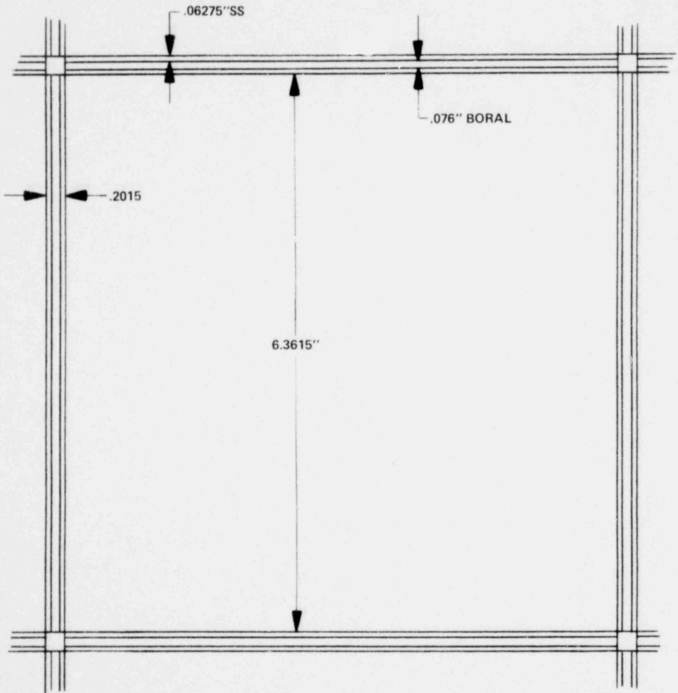
Figure 7-7 Simplified Cell Model
