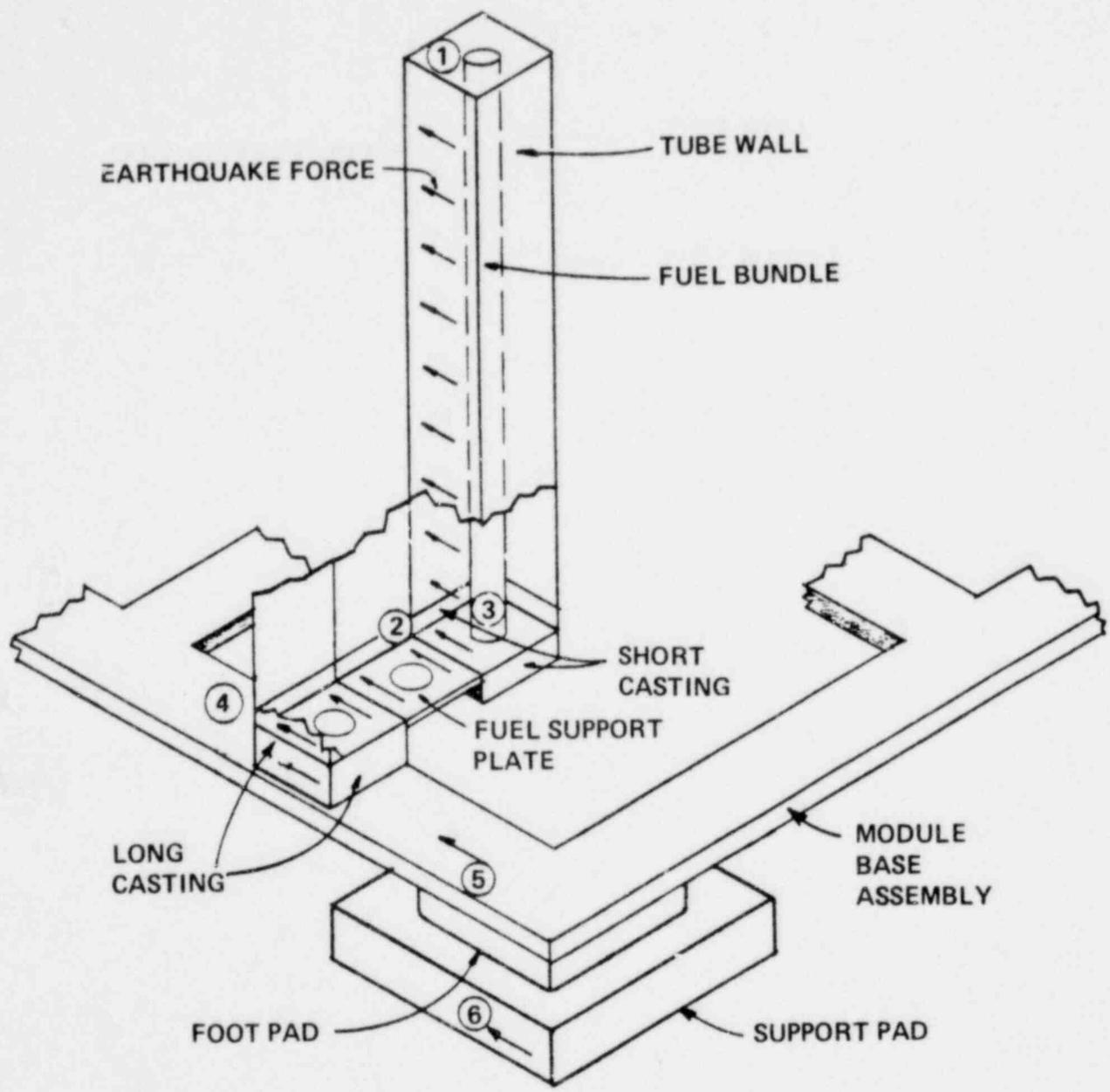
Figure 4-10 Path of Earthquake Horizontal Forces in Module
