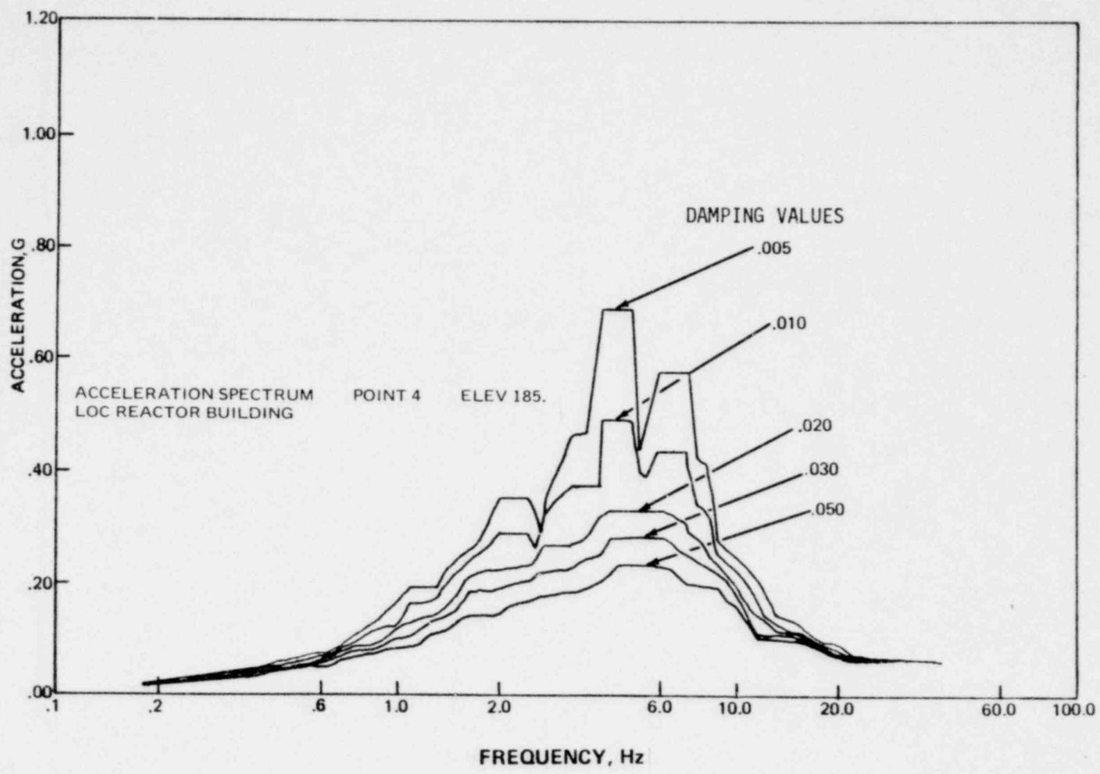
Figure 4-5 Reactor Building Vertical OBE CE 921 Analysis
