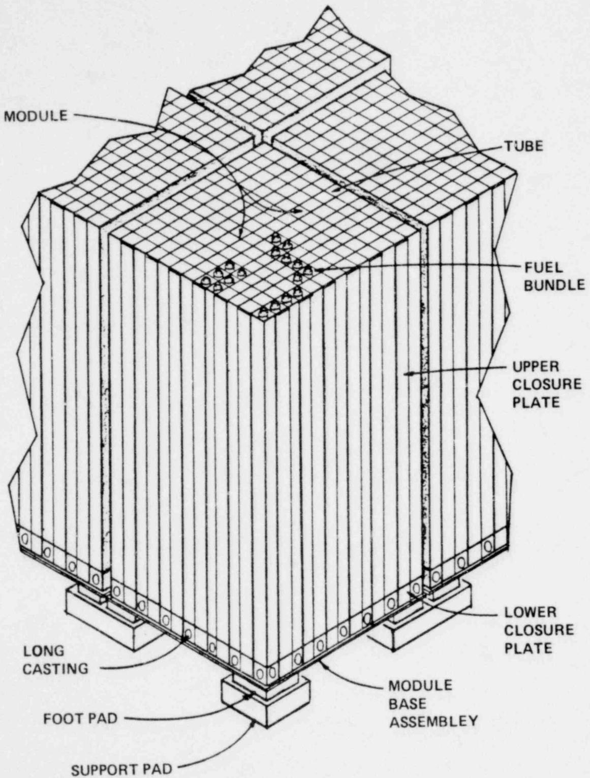
Figure 2-13 Isometric View of Modules
