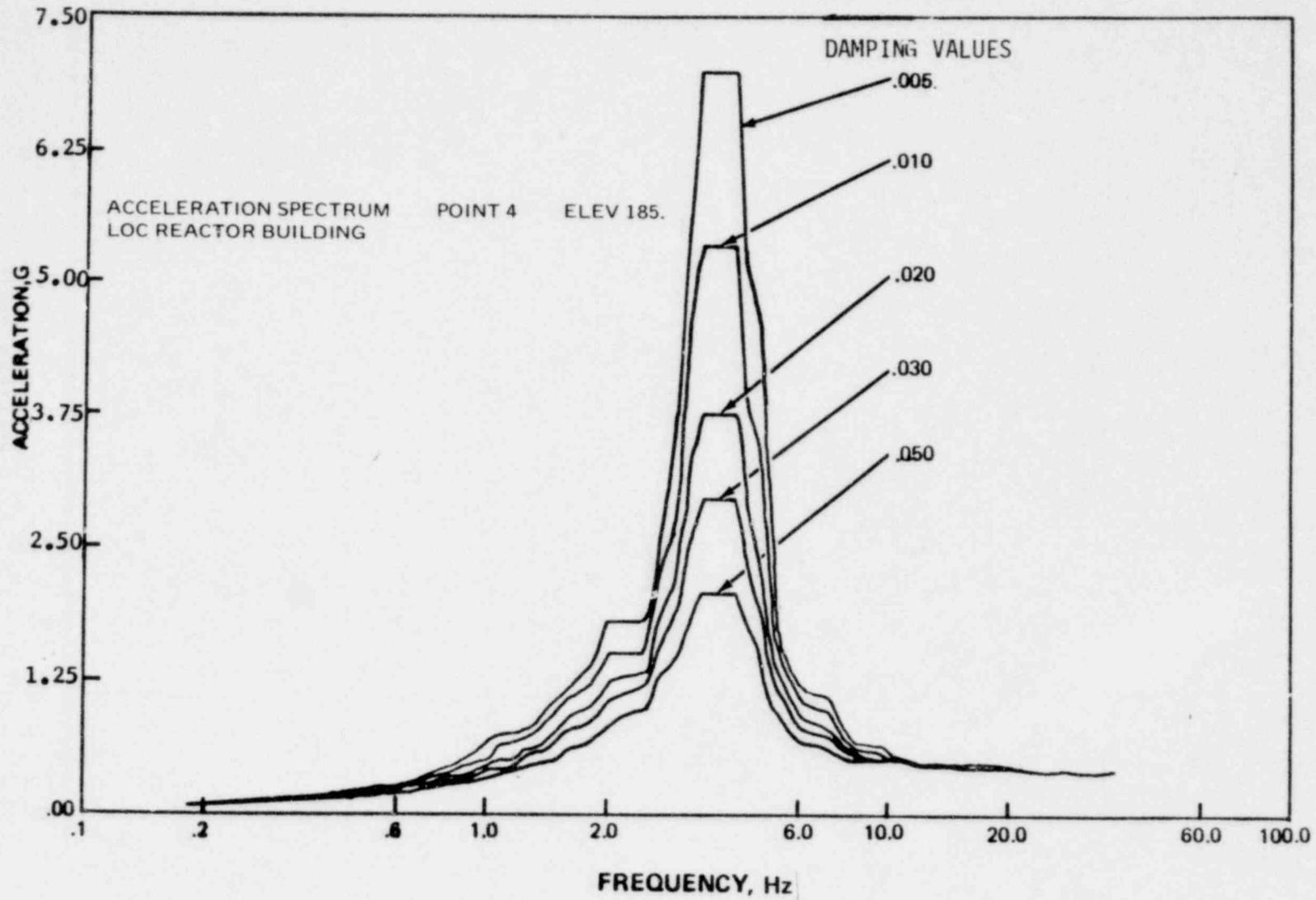
Figure 4-2 Reactor Building North-South SSE CE 921 Analysis
