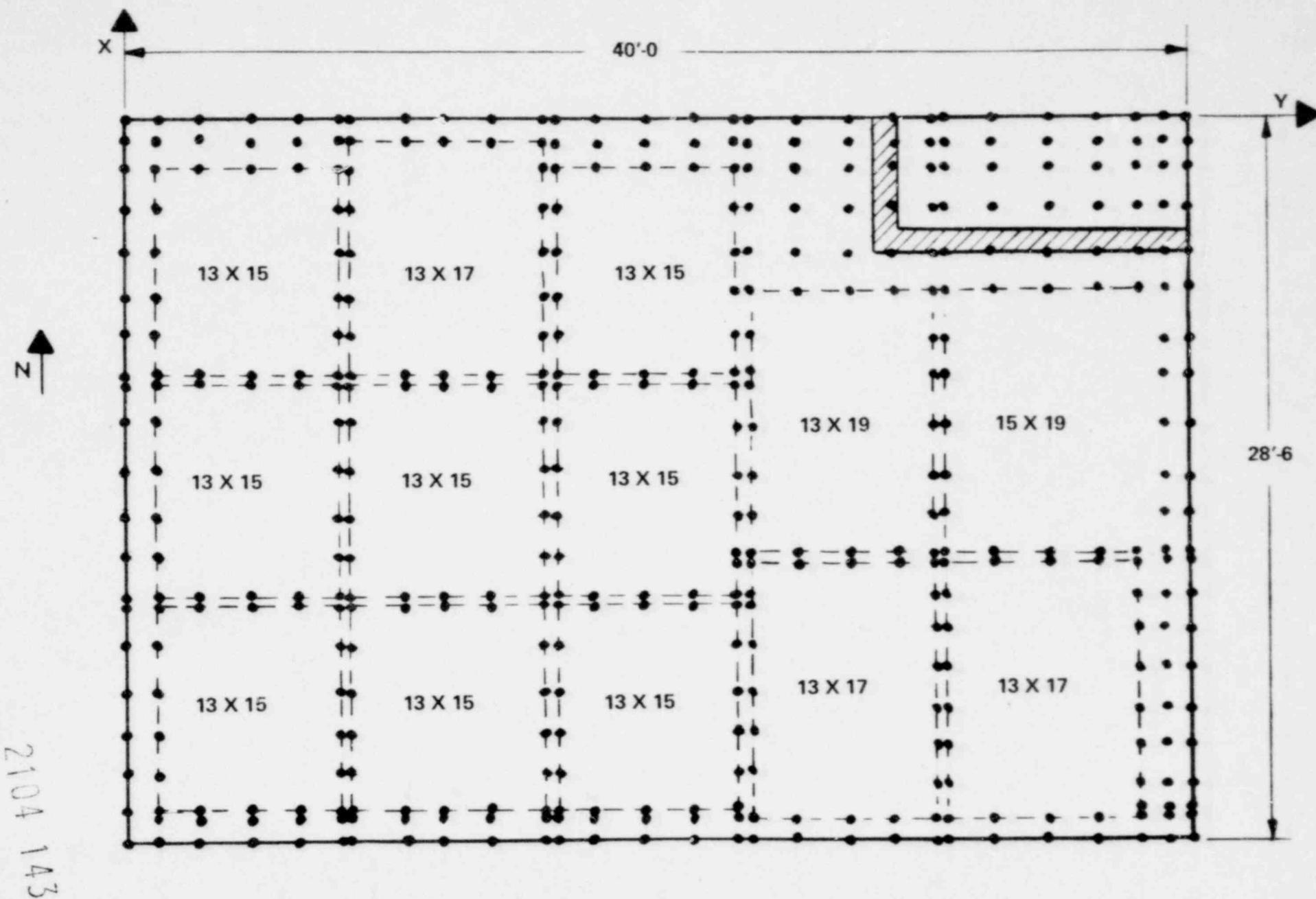
Figure 4-8 Modules and Pool Model for Hydrodynamic Virtual Mass Analysis Hatch 2
