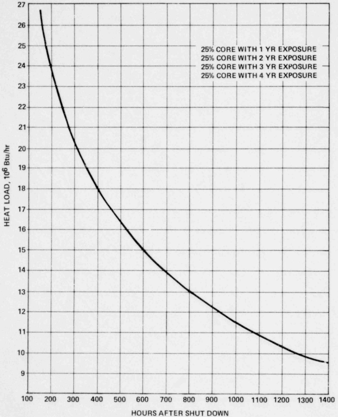
Figure 8-3 Full Core Heat Load As a Function of Time After Shutdown
