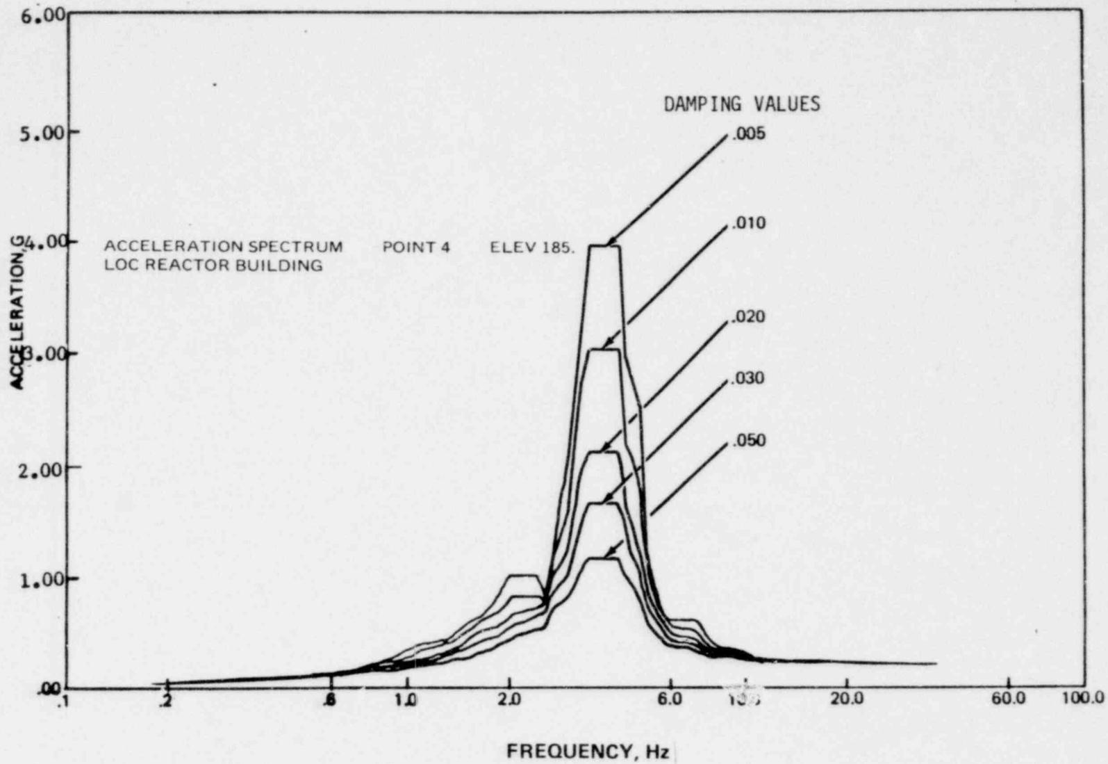
Figure 4-1 Reactor Building North-South OBE CE 921 Analysis
