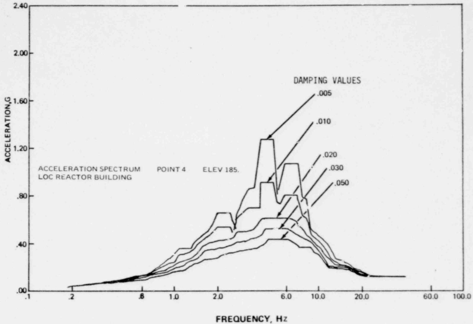
Figure 4-6 Reactor Building Vertical SSE CE 921 Analysis
