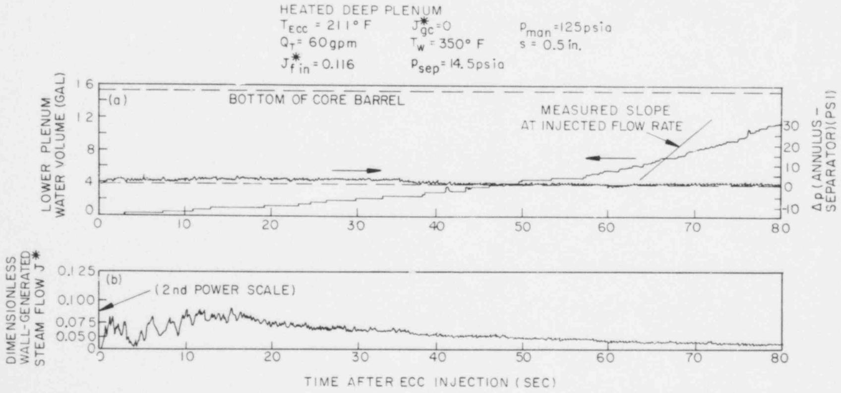
Figure 5. MEASUREMENT OF SEPARATOR VESSEL STEAM OUTFLOW WITH HEATED PLENUM ( $T_{ECC} = 210^{\circ}F$ )
