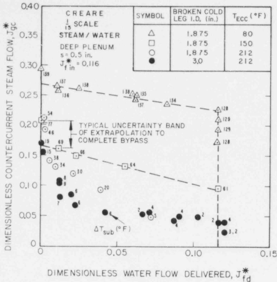
Figure 9. ILLUSTRATION OF THE DIFFICULTY OF SUBCOOLED WATER DATA EXTRAPOLATION TO SATURATION
