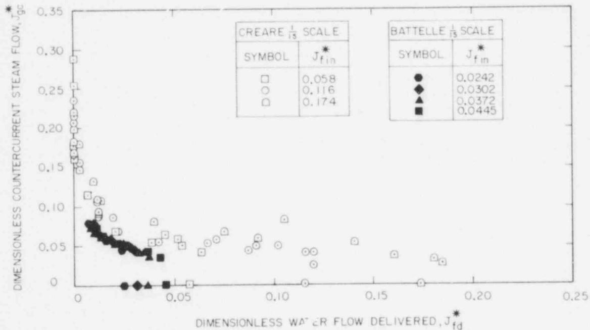
Figure 17. COMPARISON OF BATTELLE 1/15 SCALE AIR/WATER DATA WITH CREARE 1/15 SCALE DATA
