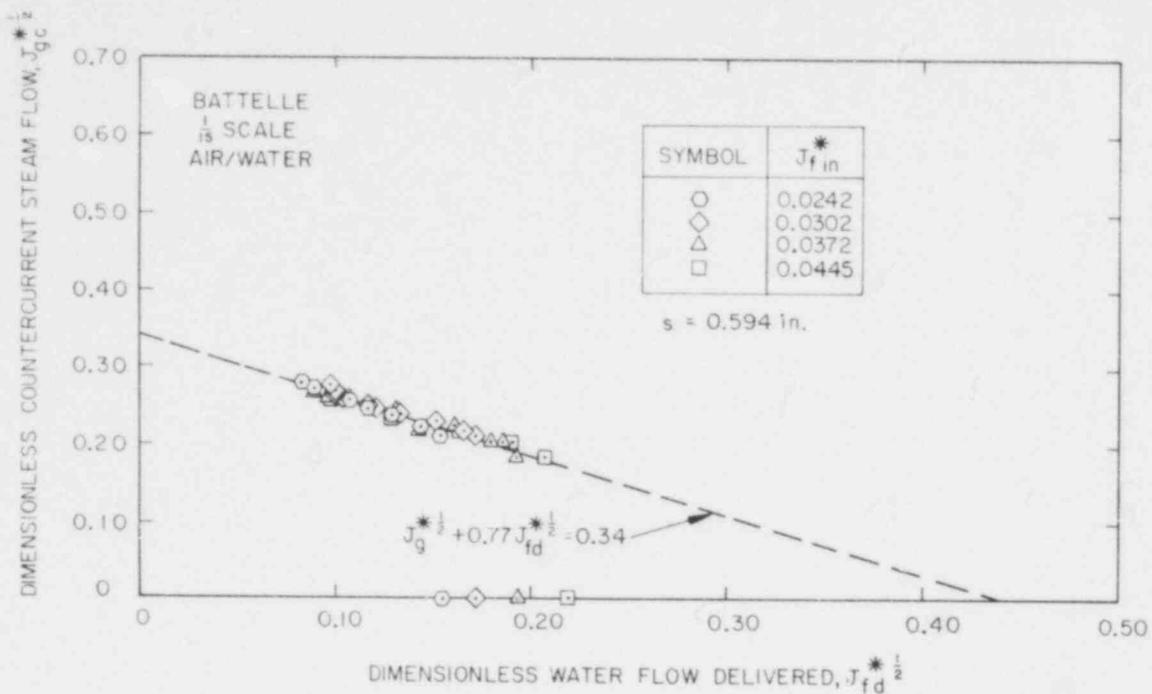
Figure 18. BATTELLE 1/15 SCALE AIR/WATER DATA [30]
