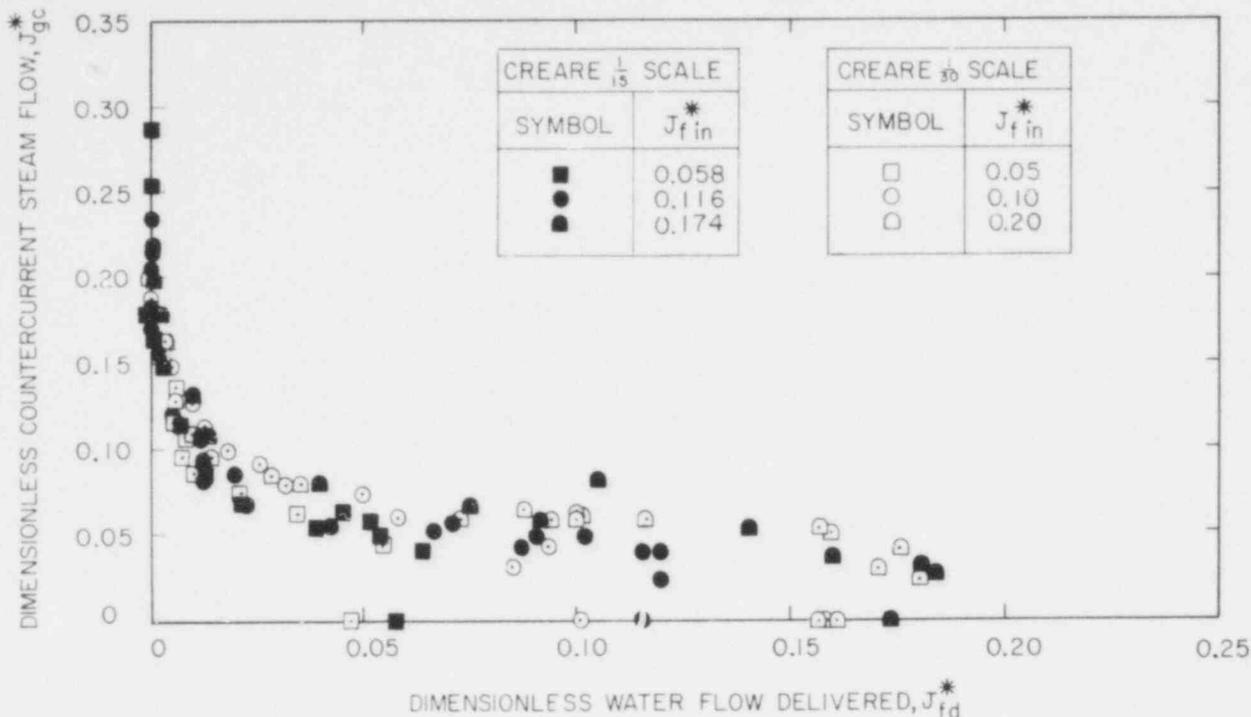
Figure 12. COMPARISON OF CREARE 1/30 AND 1/15 SCALE FACILITY WATER DATA
