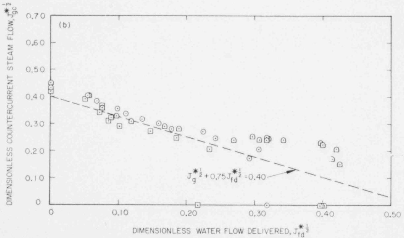
Figure 10. CREARE 1/30 SCALE SATURATED WATER DATA [27]
