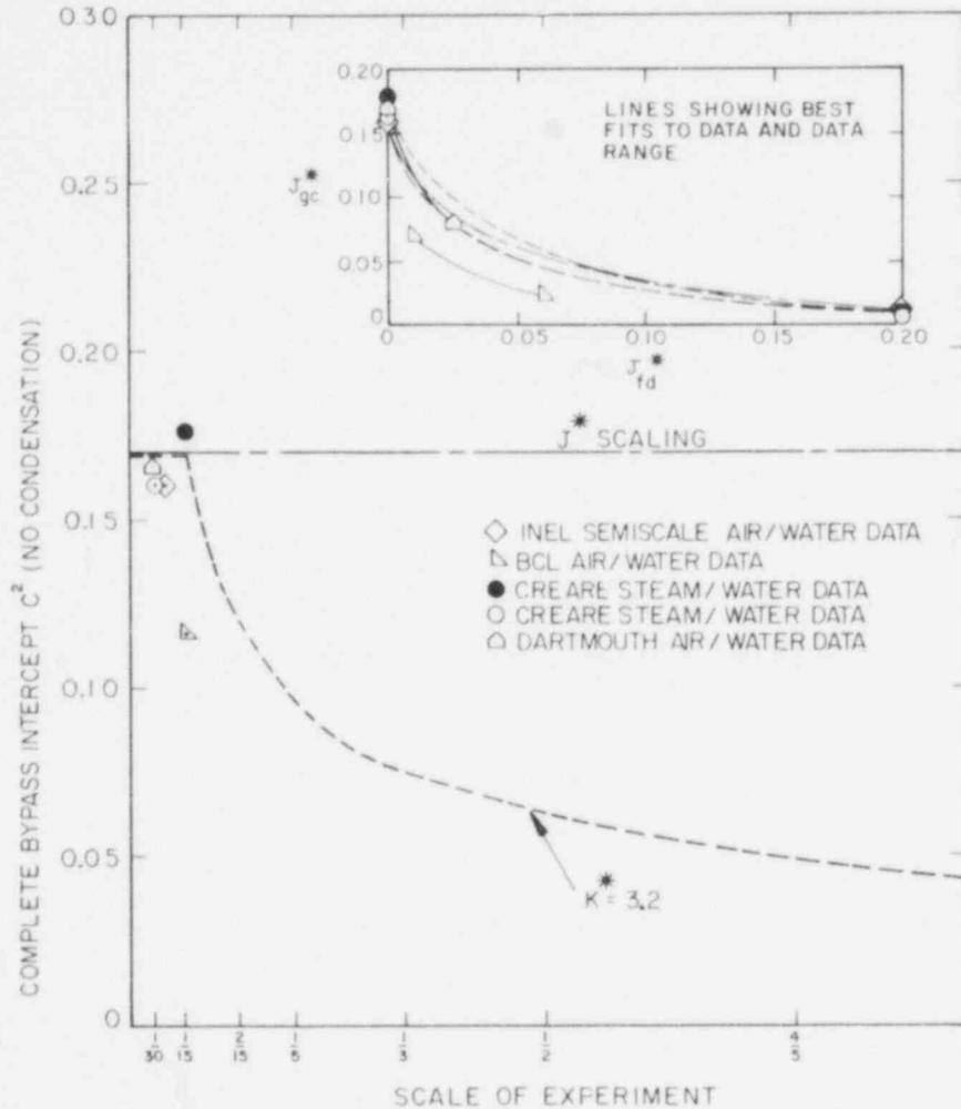
Figure 7. SUMMARY OF EXPERIMENTAL RESULTS FOR COMPLETE BYPASS OF SATURATED WATER AT SEVERAL SCALES
