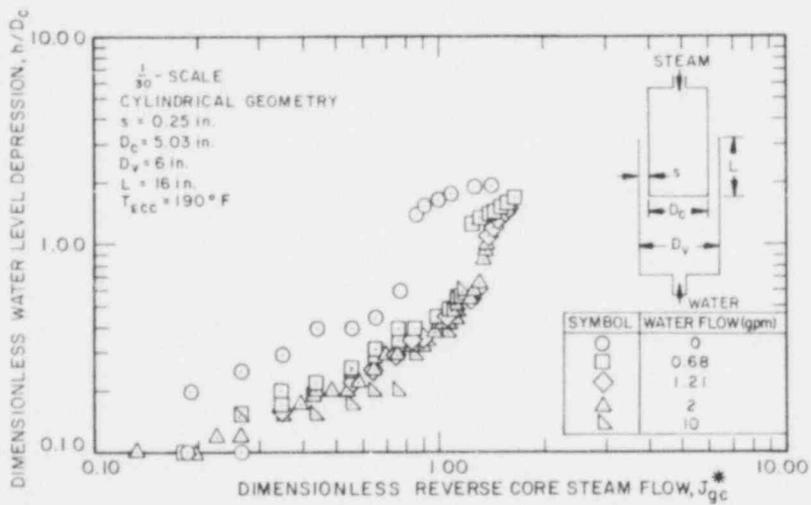
Figure 3. SAMPLE LOWER PLENUM VOIDING DATA FROM 6" ID TRANSPARENT VESSEL
