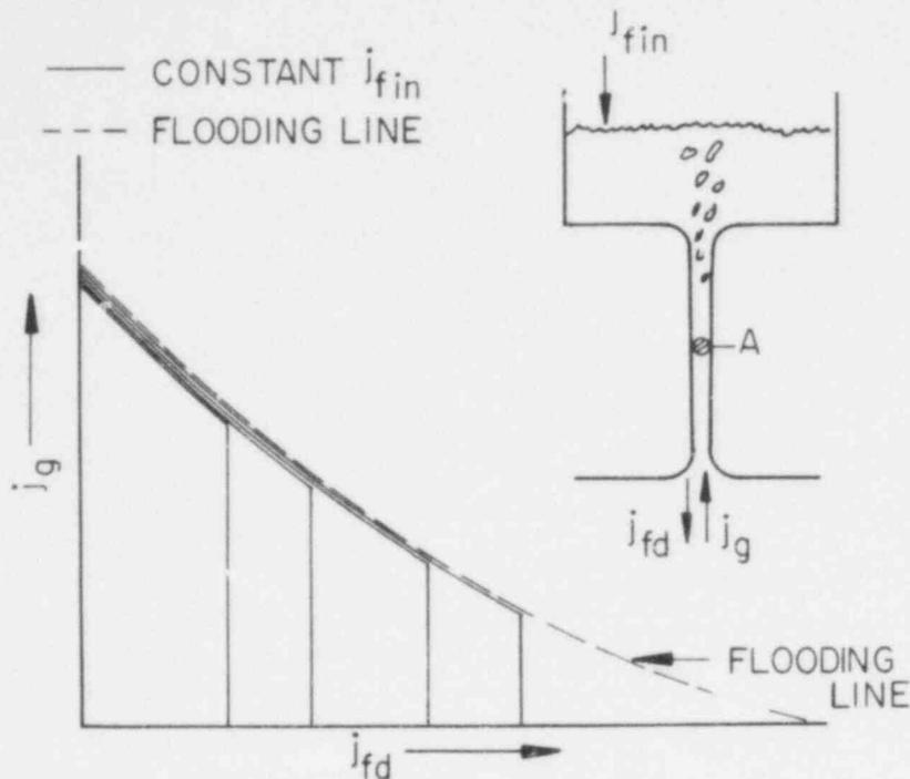
Figure 6. TYPICAL COUNTERCURRENT FLOW CHARACTERISTICS FOR A VERTICAL TUBE
