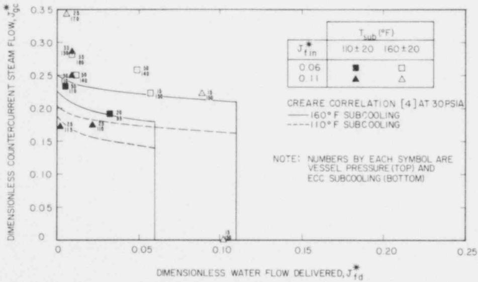
Figure 20. COMBUSTION ENGINEERING 1/5 SCALE DATA WITH HIGHLY SUBCOOLED WATER [31]
