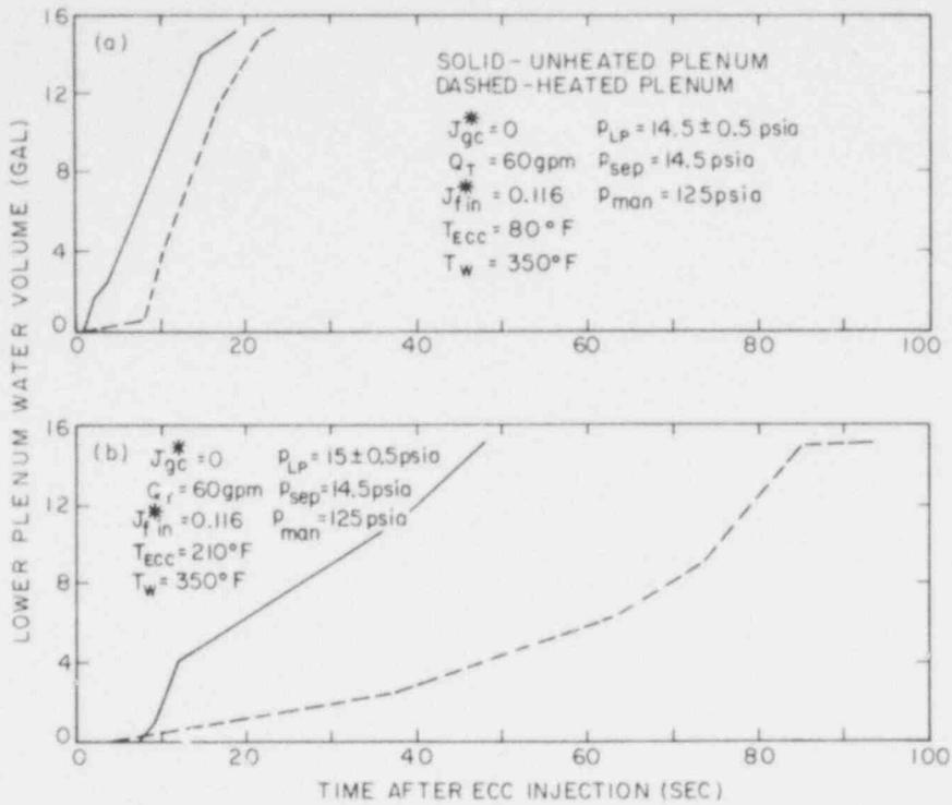
Figure 2. EFFECT OF HEATED PLENUM ON PLENUM FILLING WITH  $T_{ECC} = 80^\circ$  F AND  $212^\circ$  F
