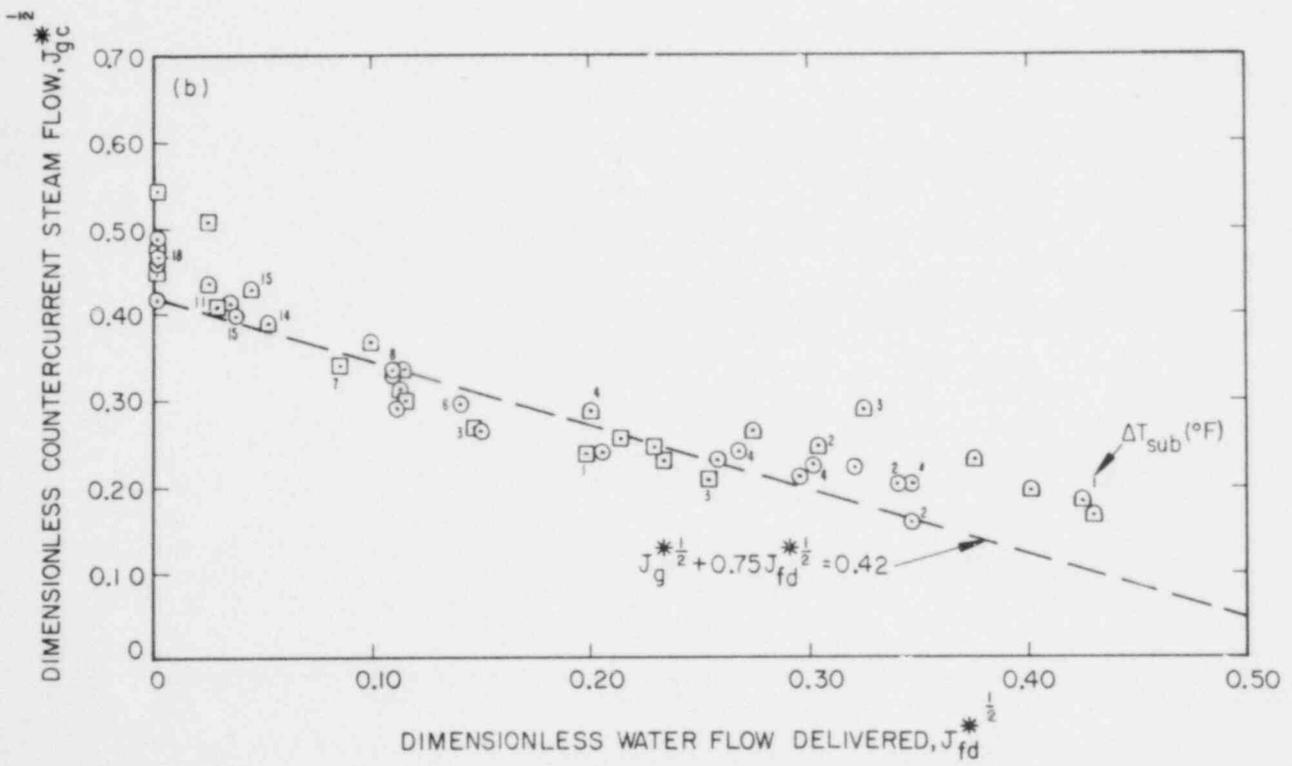
Figure 11. CREARE 1/15 SCALE SATURATED WATER DATA
