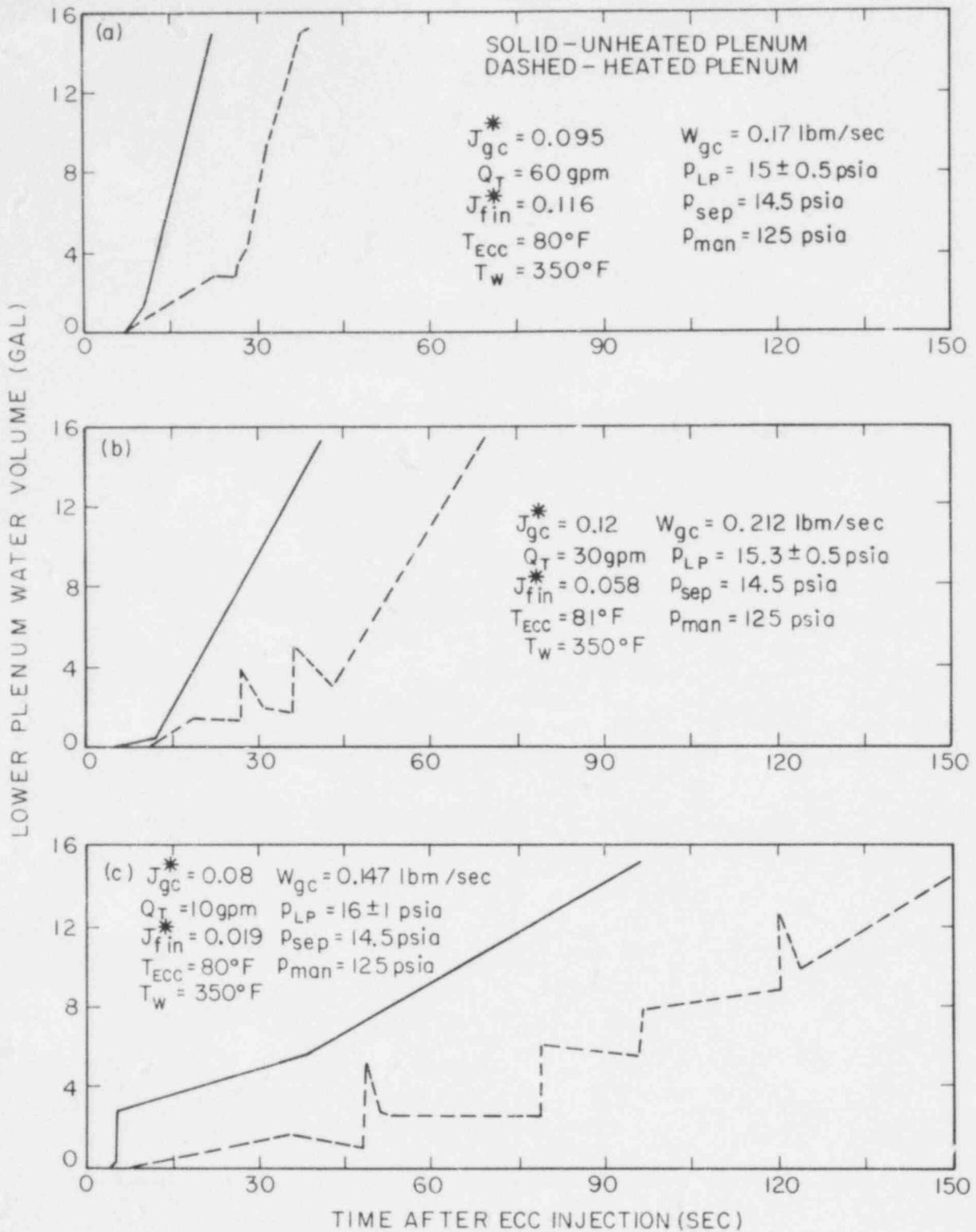
Figure 1. EFFECT OF HEATED PLENUM ON PLENUM FILLING AT VARIOUS ECC FLOW RATES
