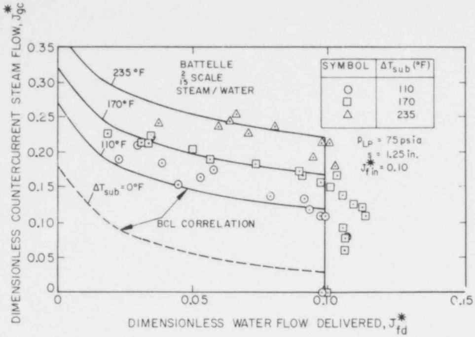
Figure 19. BATTELLE 2/15 SCALE DATA WITH HIGHLY SUBCOOLED WATER [26]
