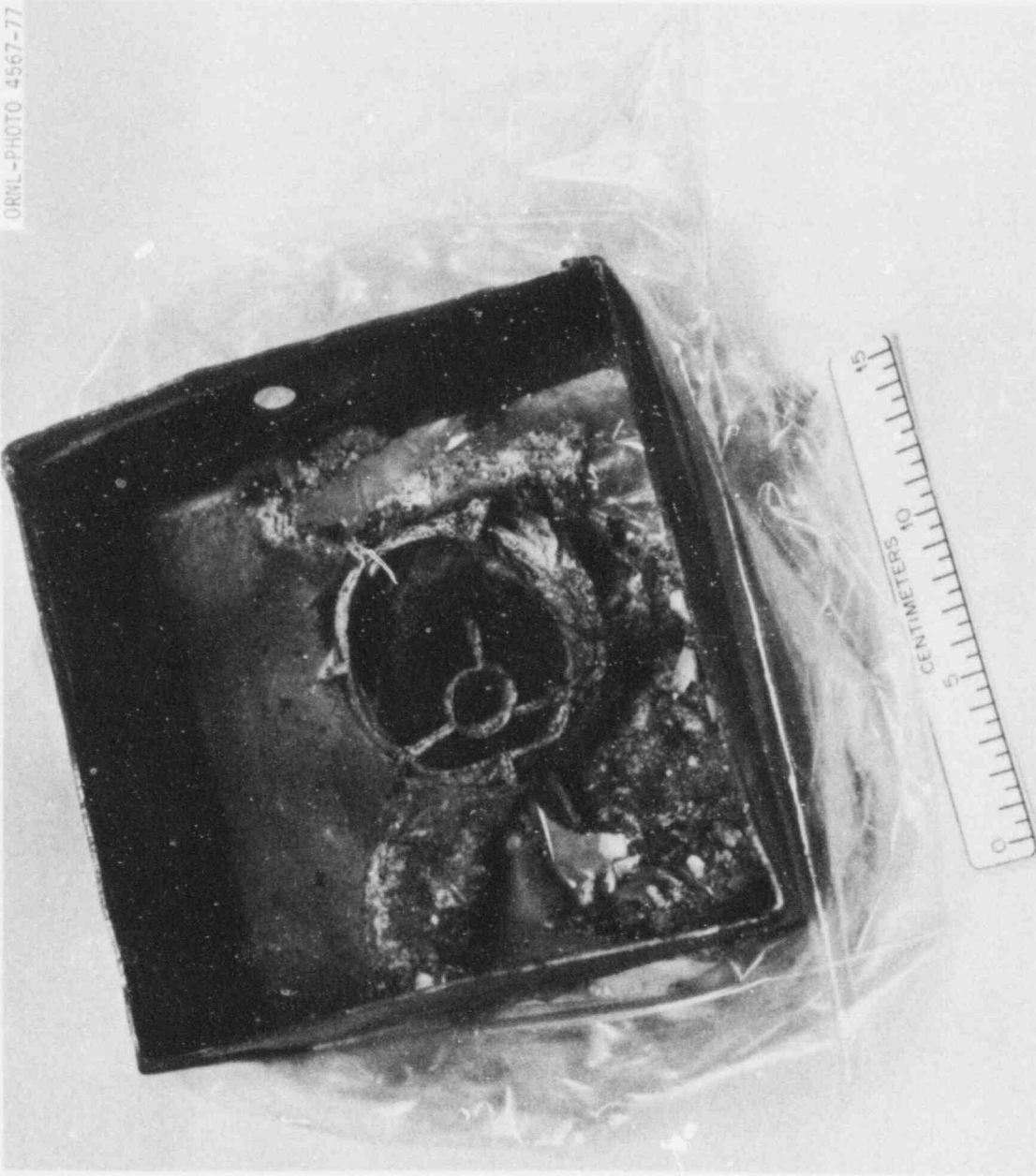
Fig. 16. Type 3 Whole Smoke Detector After Heating to 1200°C
