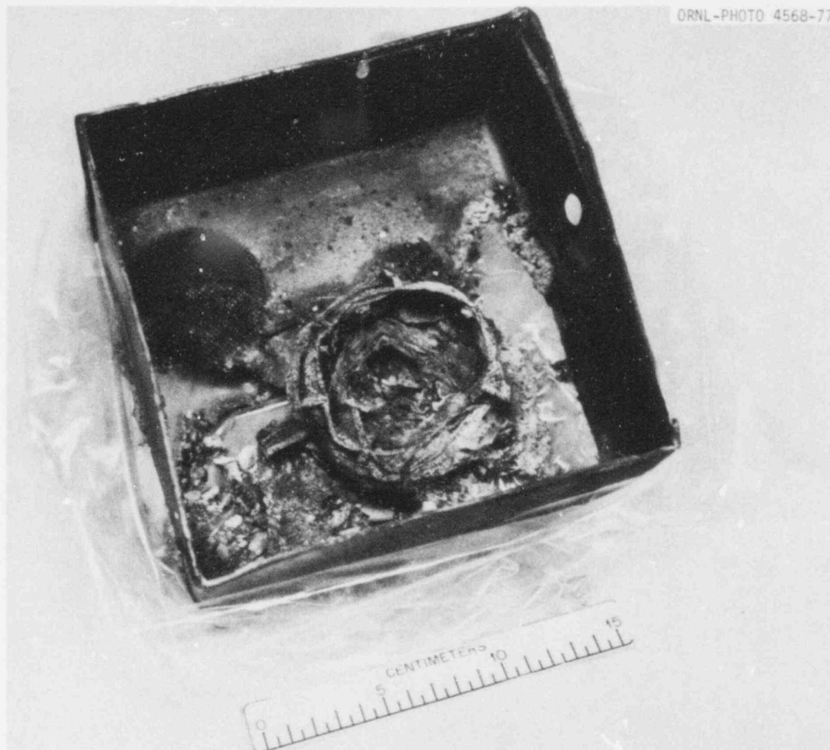
Fig. 17. Whole Smoke Detector After Heating to 1200°C (wire screen displaced in order to show inner damage)
