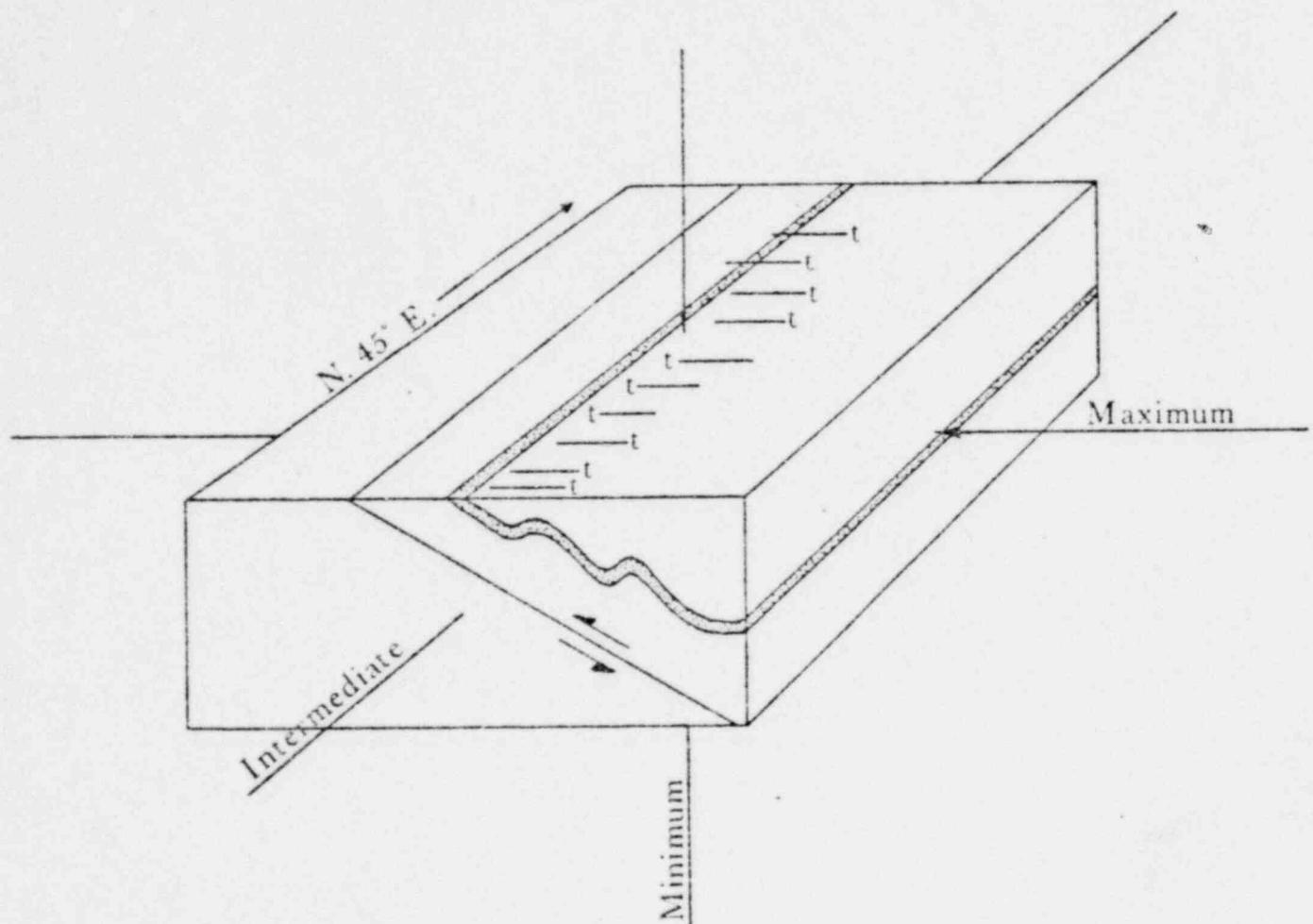
Figure 1. Orientation of stress axes compatible with structural features present in the Phipps Bend, Tennessee, area. Faults and folds are shown diagrammatically. Symbols: t = tensional fractures, arrows show relative motion of fault blocks, and axes are labelled. Modified isometric base distorts right-angle relations.
