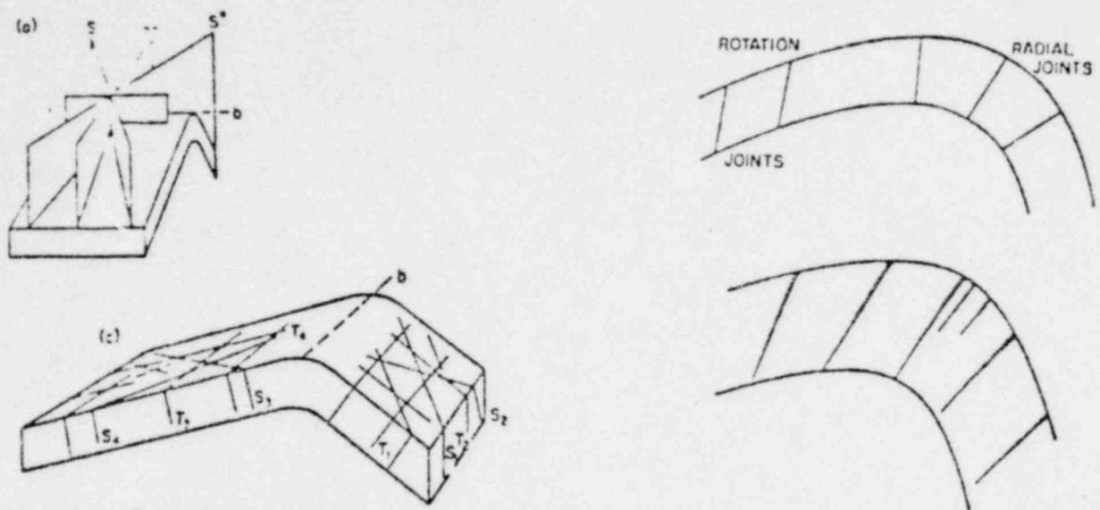
Figure 4. Relation of joint patterns to bedding in folded rocks (Price, 1966). Diagrams at left show 3-D view of shear joints (labelled  $S_1$ ,  $S'$ , etc.) and tension joints (labelled  $T_1$ ,  $T_2$ , etc.). The diagrams at the right show radial joints and rotation joints (labelled at top), and axial plane joints filled by mineral deposits (lower diagram).
