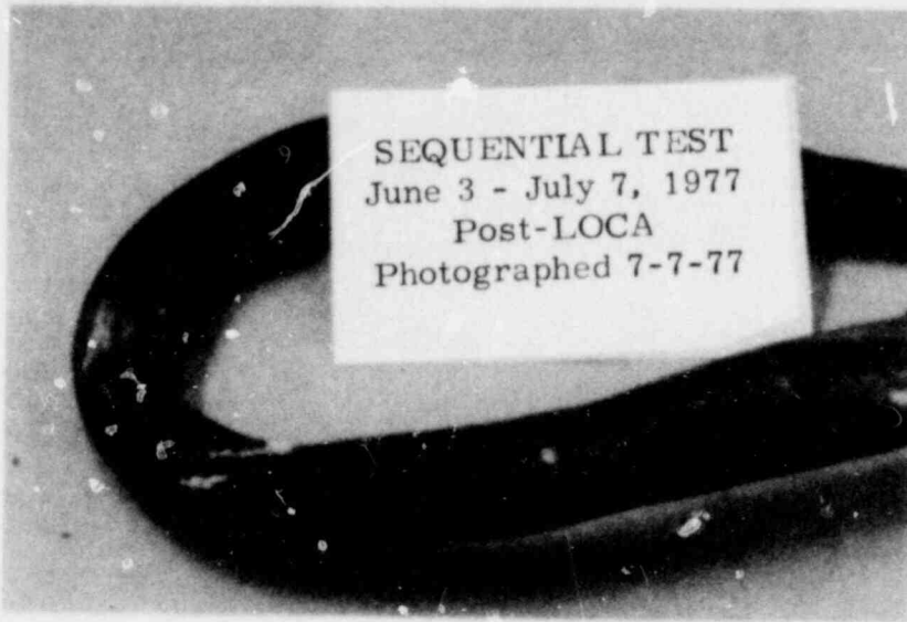
Figure 5. The type A/bend splice after a sequential test and approximately 360 megarads dose. Some minor surface roughness is visible in the bend area.
