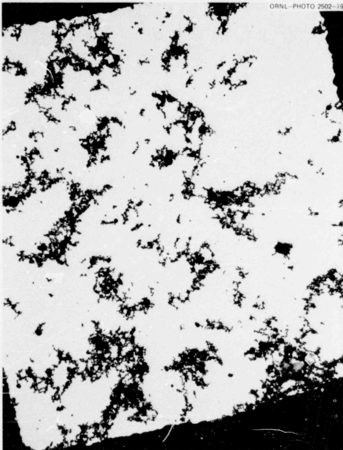
Fig. 18. Agglomerated U_3O_8 particles from run PT-17 initial fall-out sample.
