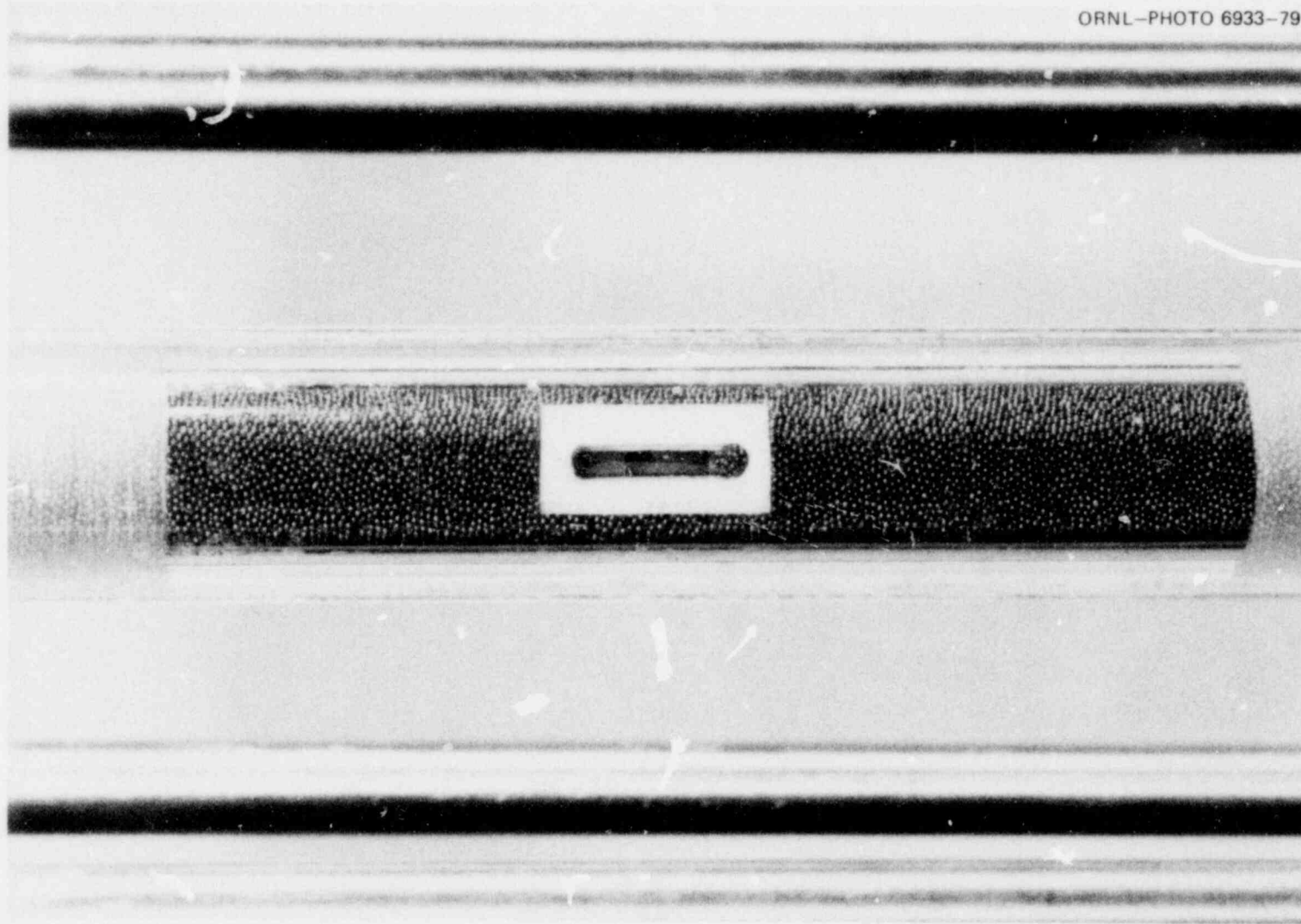
Fig. 9. Close-up view of sample assembly used in CDV 76 showing \text{Al}_2\text{O}_3 window glued to ID of tube, exposed side of \text{UO}_2 pellet with a 1/16-in.-diam hole, and \text{UO}_2 microspheres surrounding rest of pellet stack.
