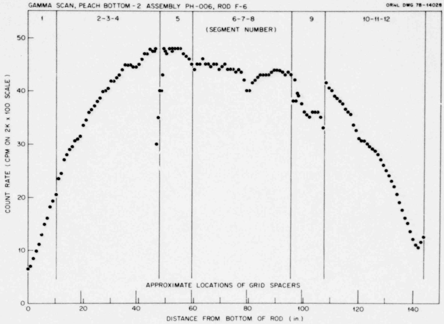
Fig. 3. Gamma scan of rod F-6 from bundle PH-006, Peach Bottom-2 Reactor.
