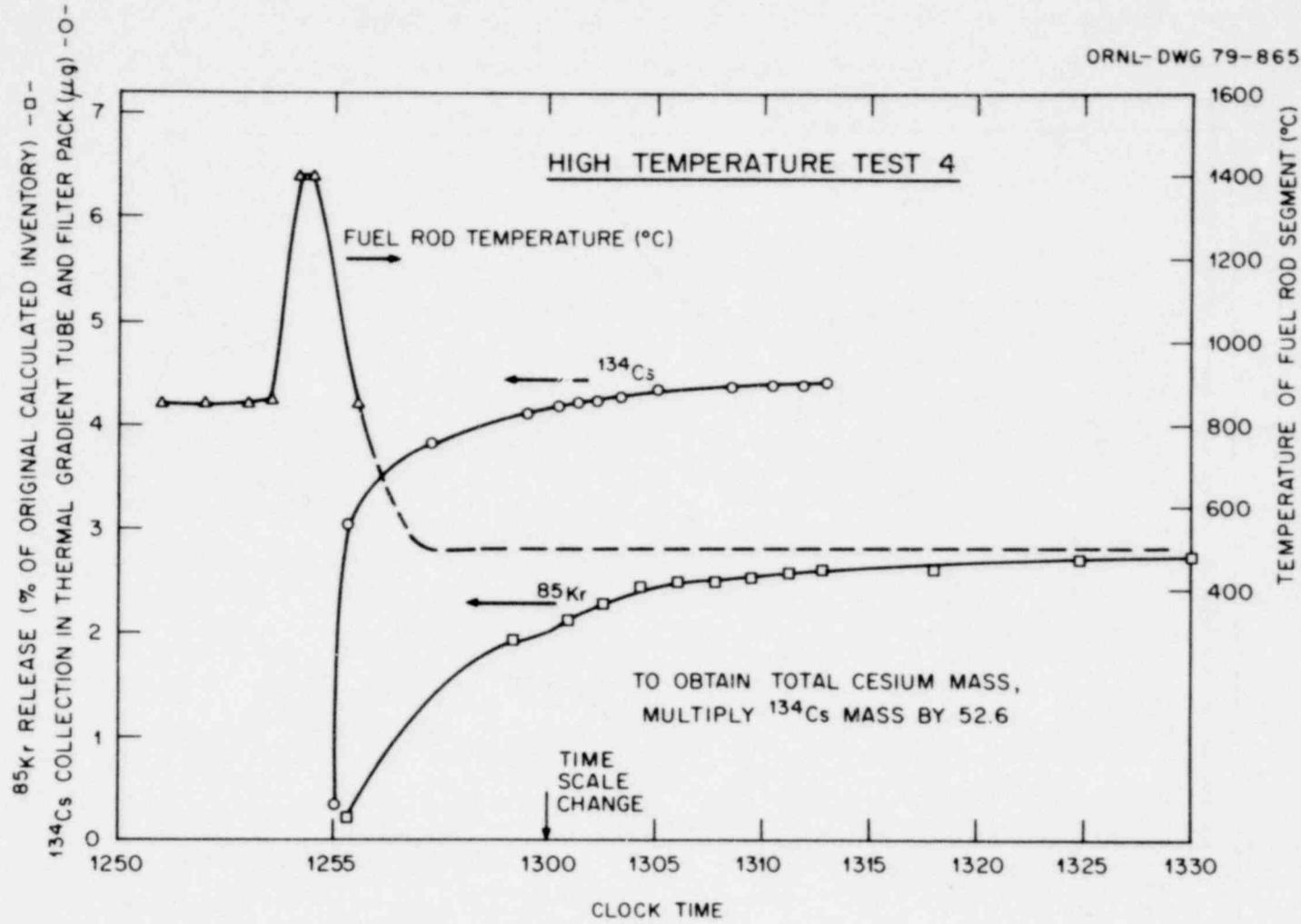
Fig. 2. Collection of <sup>134</sup>Cs in the thermal gradient tube and filter pack and of <sup>85</sup>Kr in the charcoal traps during test HT-4.
