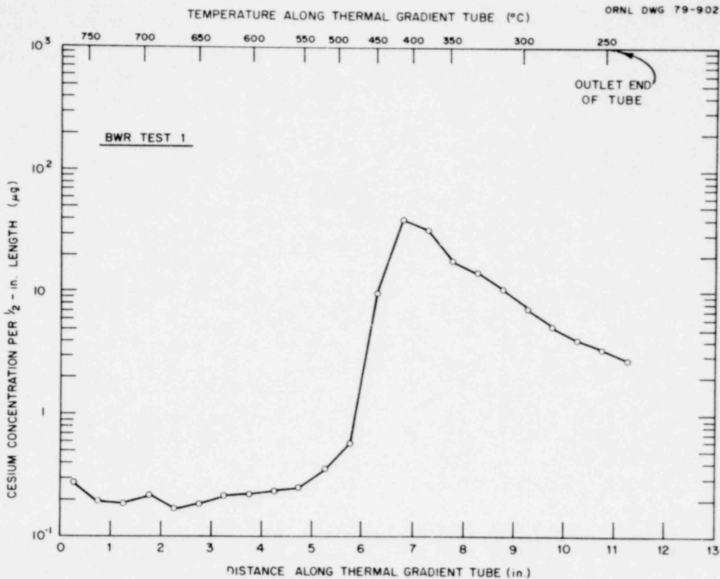
Fig. 5. Distribution of cesium collected in the thermal gradient tube during test BWR-1.
