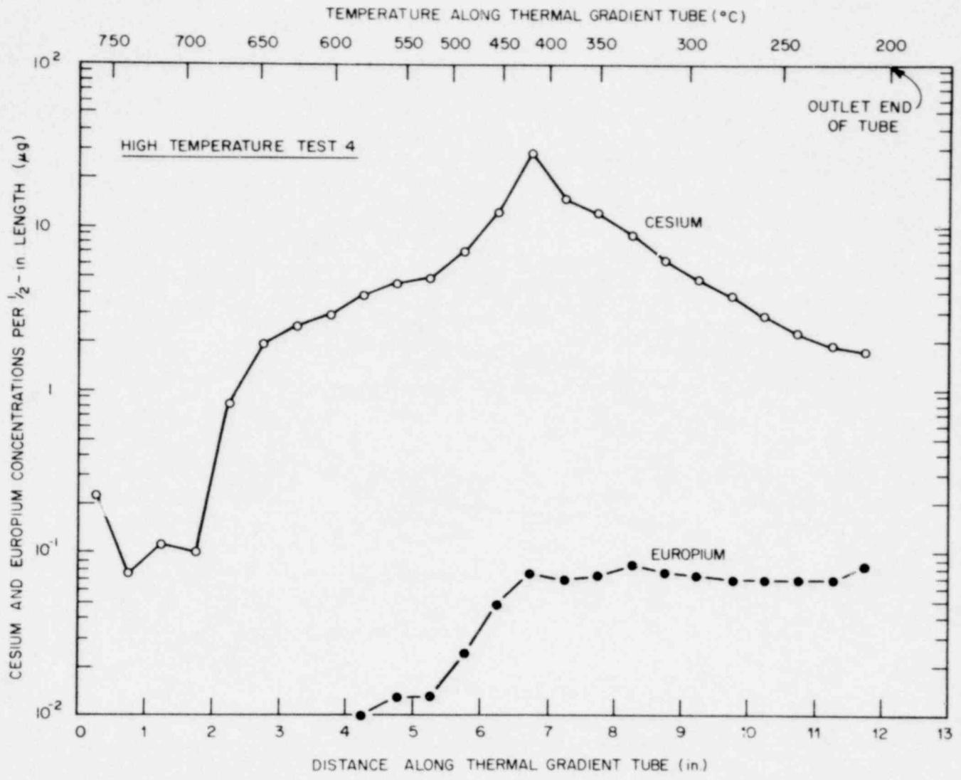
Fig. 1. Distribution of cesium and europium collected in the thermal gradient tube during test HT-4.
