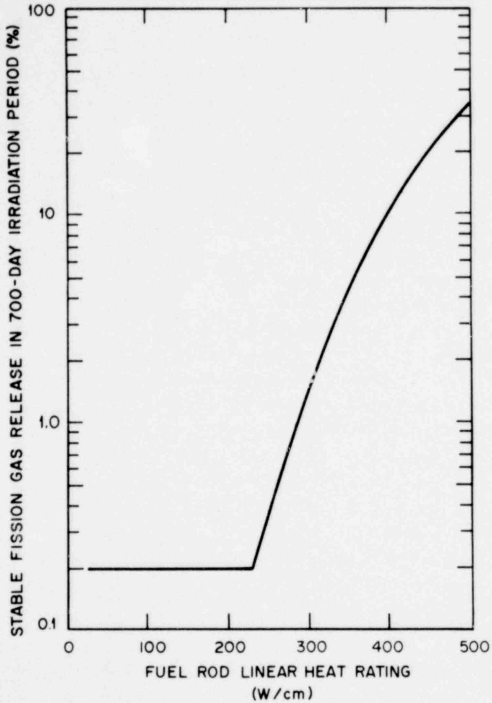
Fig. 4. Stable fission gas release estimated as a function of linear heat rating.
