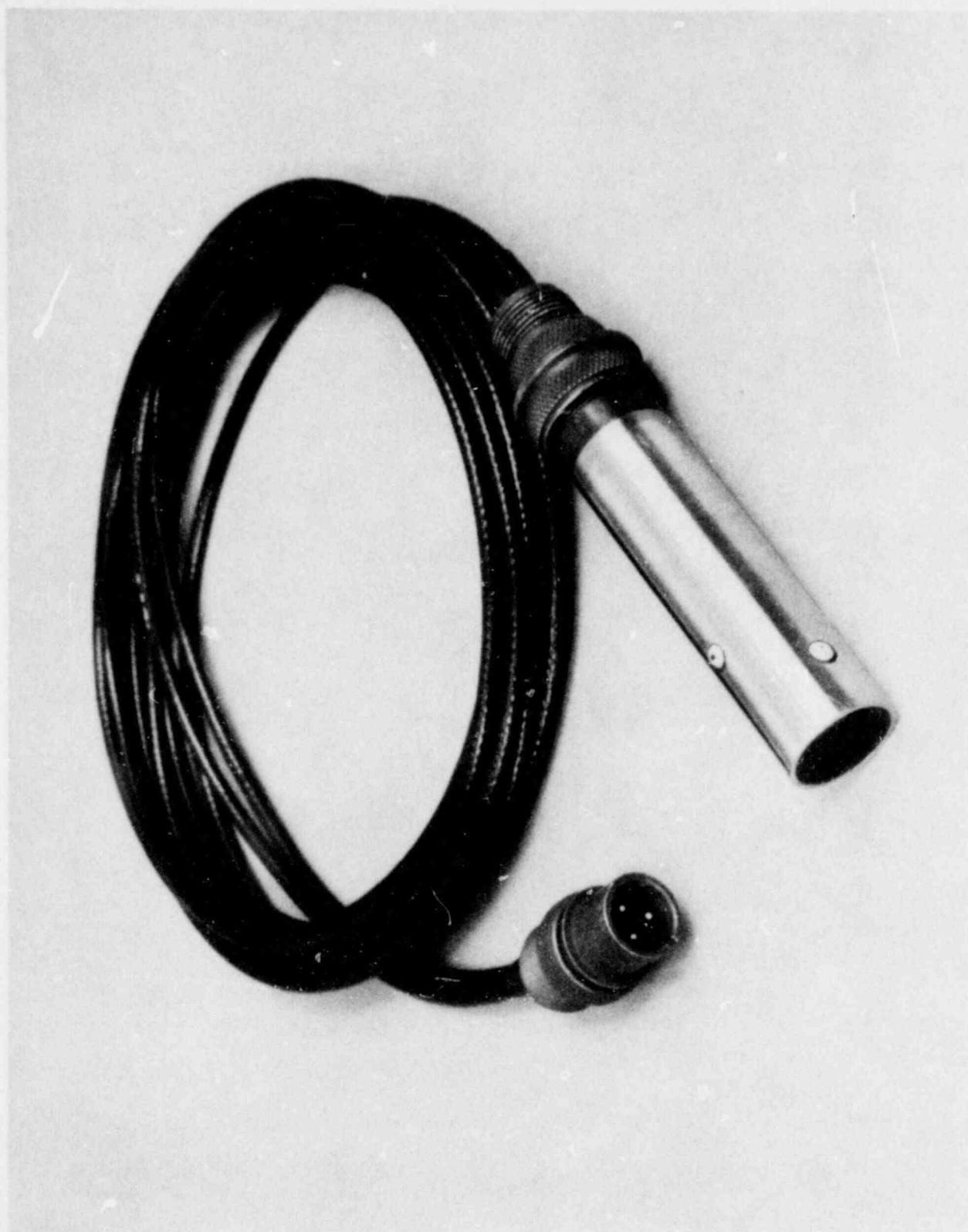
Figure 3. Inspection Probe showing entry holes to eddy current coils.
