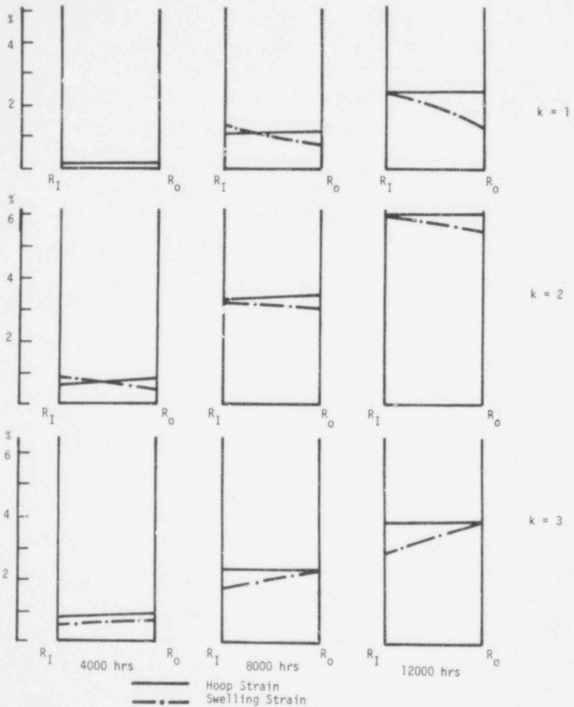
Figure H0 - 9. The Distribution of the Hoop Strain and the Swelling Strain Across the Clad Wall (Case H0)
