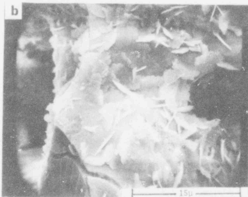
FIGURE 10. Magnified Photograph Illustrating the Porous Structure of a Particle in the Size Range 2,362 \mu to 833 \mu Shown in Figure 9(a).
