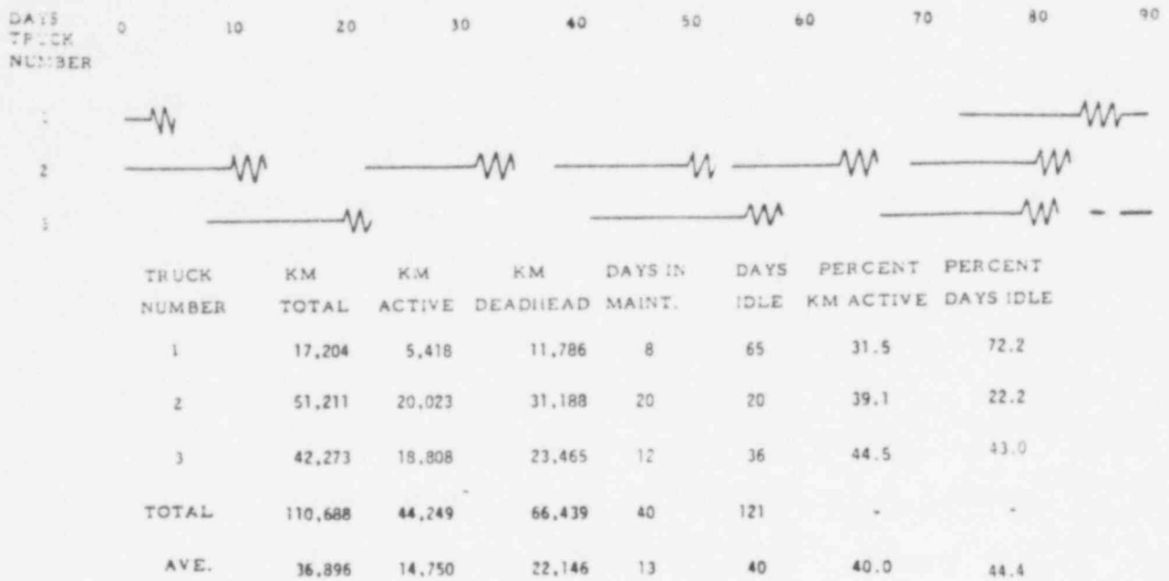
Figure 3.6 Schedule 1 trailer/tractor itineraries with linking value penalty coefficients idle 2, deadhead 2, flexibility loss 0.1, and total time 0.
