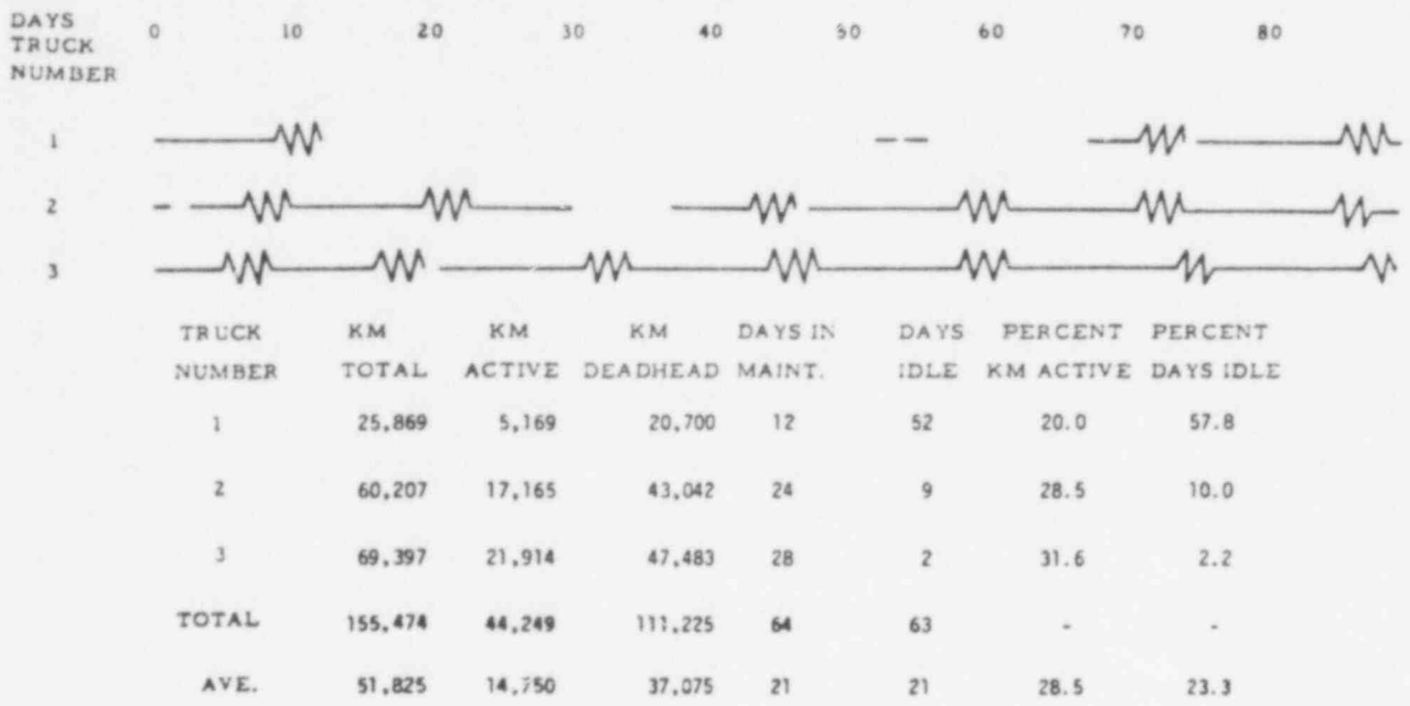
Figure 3.8. Schedule 1 trailer/tractor itineraries with linking value penalty coefficients idle 2, deadhead 1, flexibility loss 1 and total time 0.
