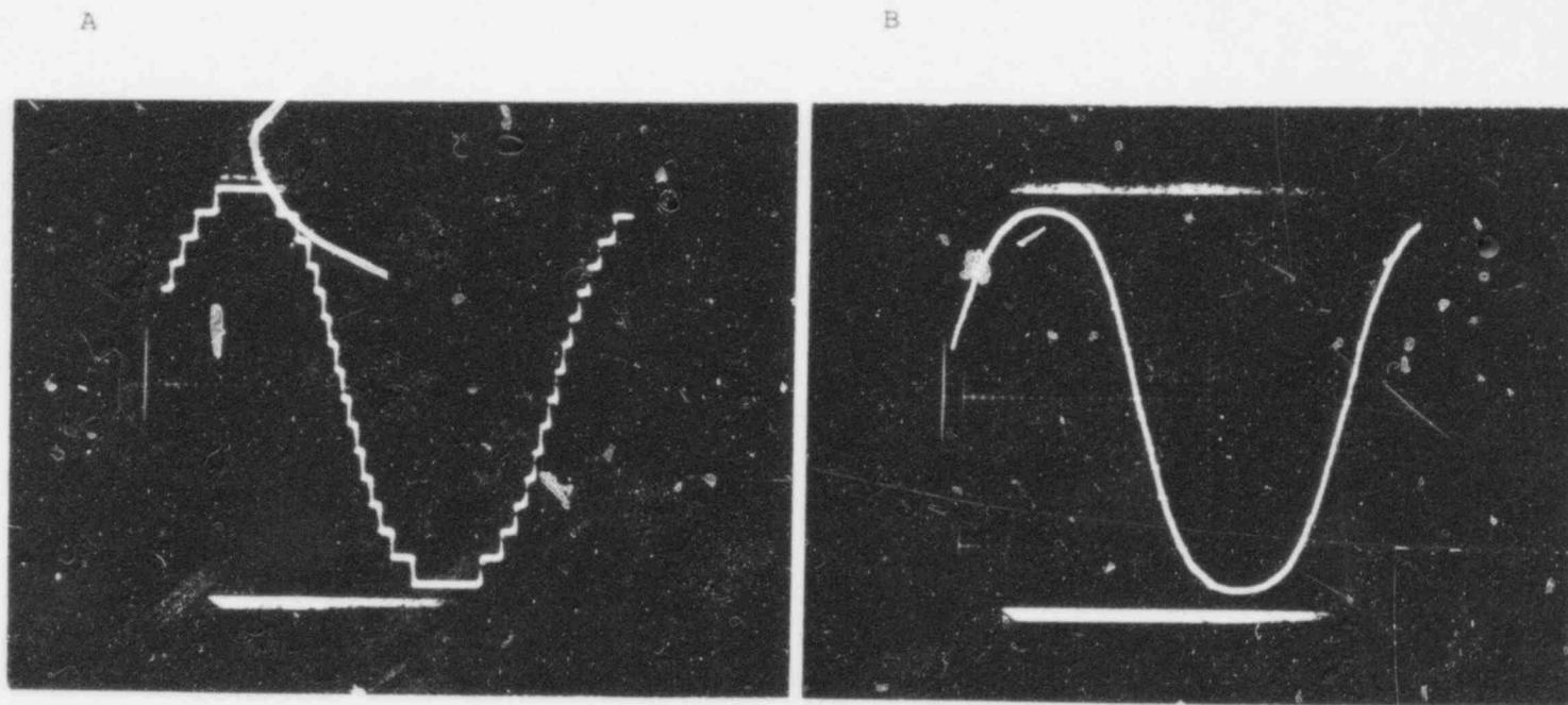
Figure 1. Demonstration of averaging capability of NBS system. Input sinusoid is quantized by 16-level analog-to-digital converter and averaged 256 times. Horizontal axis consists of 4,000 samples at 40 ns/sample. A) Signal without additive noise. B) Signal after noise equal to one-sixteenth of full scale is added. Averaging smooths out the coarse quantization steps produced by the analog-to-digital converter.
