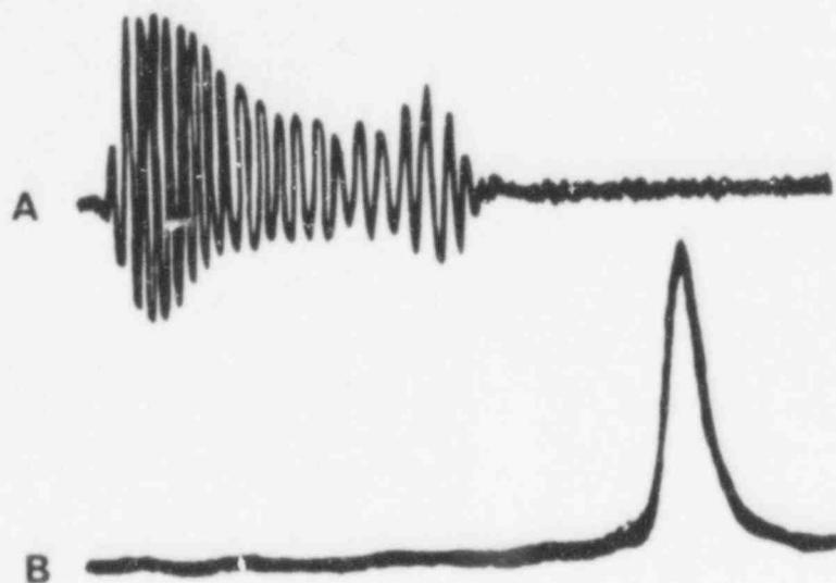
Figure 4. (A) Preamplified normal echo from the rear of an aluminum block. (B) The same signal following compression and detection. A 4.8  $\mu$ s pulse is compressed to a halfwidth of 0.6  $\mu$ s.
