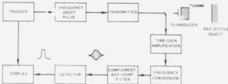
Figure 3. Block diagram of pulse compression ultrasound system.
