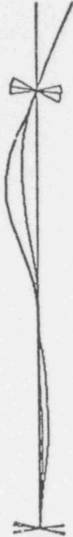
Figure 5-10. Second Fundamental Mode Shape of SSHT and Capsules (Radial Motion  $F = 219$  Hz)
