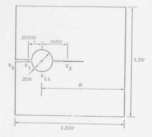
FIGURE 2. LOCATIONS WHERE CRACK-LINE DISPLACEMENTS WERE CALCULATED FOR CLWL SPECIMEN
