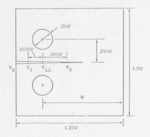
FIGURE 1. LOCATIONS WHERE CRACK-LINE DISPLACEMENTS WERE CALCULATED FOR COMPACT SPECIMEN
