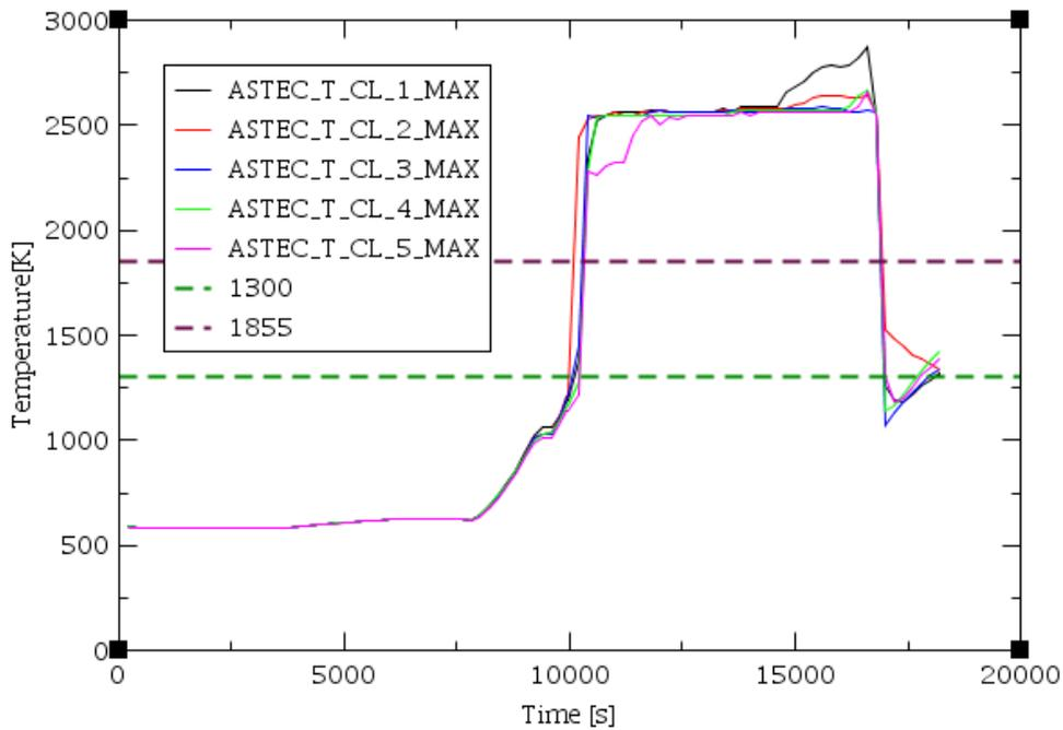
**Figure 5-25 Max Intact Cladding Temperature at the Different 5 Rings Predicted by ASTEC (maximum value achieved from the beginning of the transient)**
