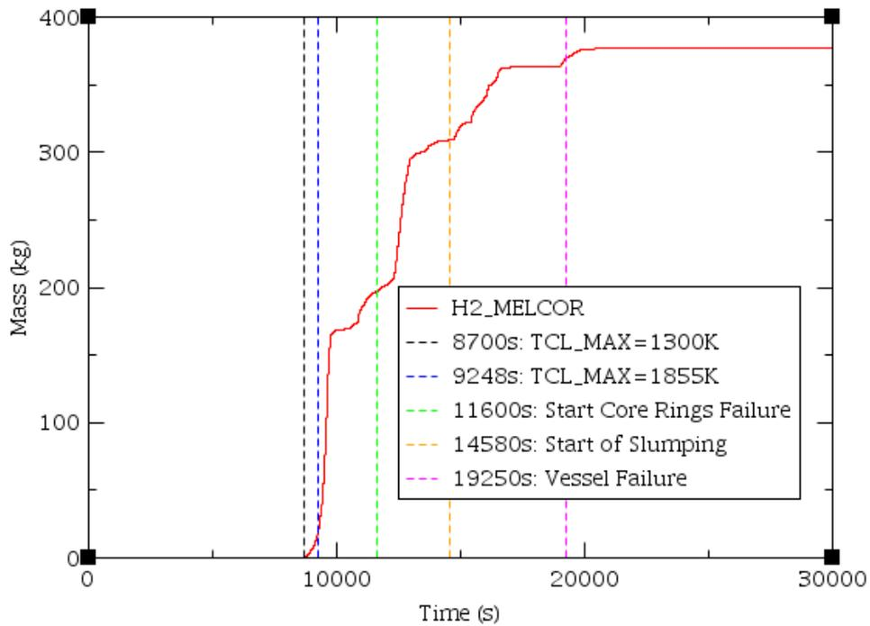
**Figure 5-36 Hydrogen Production versus Time Predicted by MELCOR**
