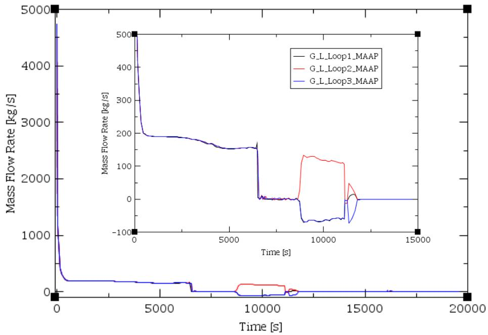
**Figure 5-23 MAAP Loop1/2/3 Mass Flow Rate Versus Time**
