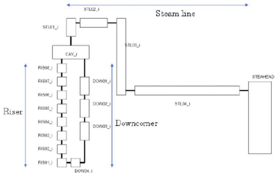
**Figure 4-3 ASTEC Nodalization of the Secondary Circuit of the Generic PWR 900 MWe Reference Reactor [33]**
