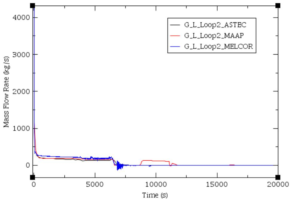
**Figure 5-20 HL Loop2 Mass Flow Rate Versus Time Predicted by ASTEC, MAAP and MELCOR**
