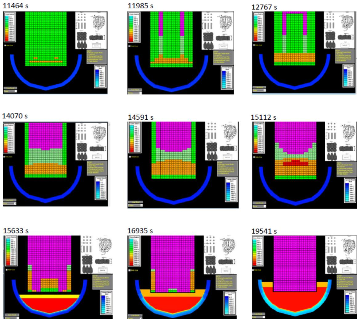
**Figure 5-40 MAAP Core Degradation Representation (number 0,1,2,3,4,5 represent the type of degradation that take place in each node; in particular : 0= Nearly Empty Node; 1=Fuel Pin; 2= Collapsed Fuel Pin; 3=Thickened Fuel Pin; 4= Impenetrable Crust; 5= Fully Molten)**
