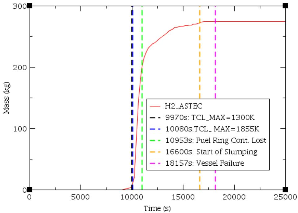
**Figure 5-34 Hydrogen Production versus Time Predicted by ASTEC**
