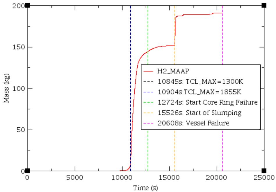
**Figure 5-35 Hydrogen Production versus Time Predicted by MAAP**
