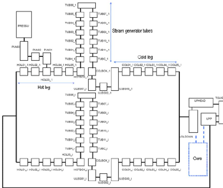
**Figure 4-2 ASTEC Nodalization of the Primary Circuit of the Generic PWR 900 MWe Reference Reactor [33]**
