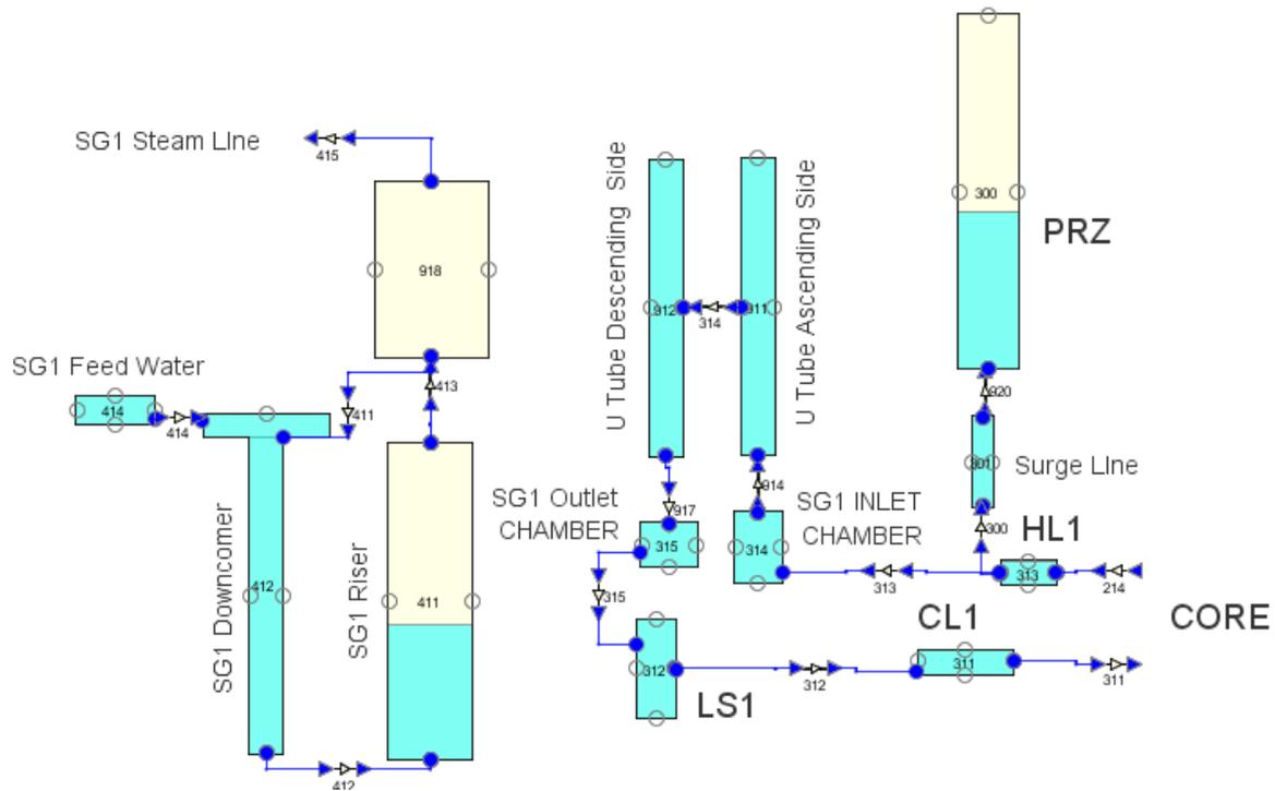
**Figure 4-7 MELCOR Loop 1 Nodalization of the Generic PWR 900 MWe Reference Reactor, Developed by Using SNAP**
