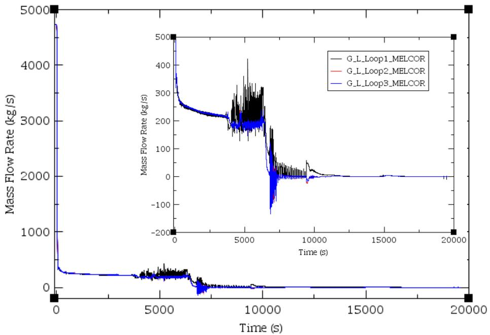
**Figure 5-24 MELCOR Loop1/2/3 Mass Flow Rate Versus Time**
