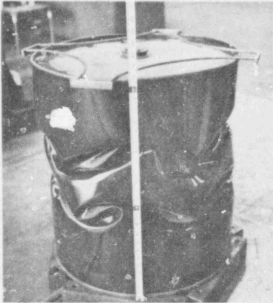
Figure 2 - 17C 16 Gage Fixed Head Drum After Maximum Load of 19,560 lbs.
