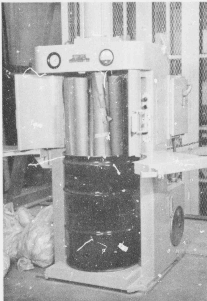
Figure 7 - S-E-Co. hydraulic compactor, drum loaded with rolled paper. Drum extension and split loading table open.
