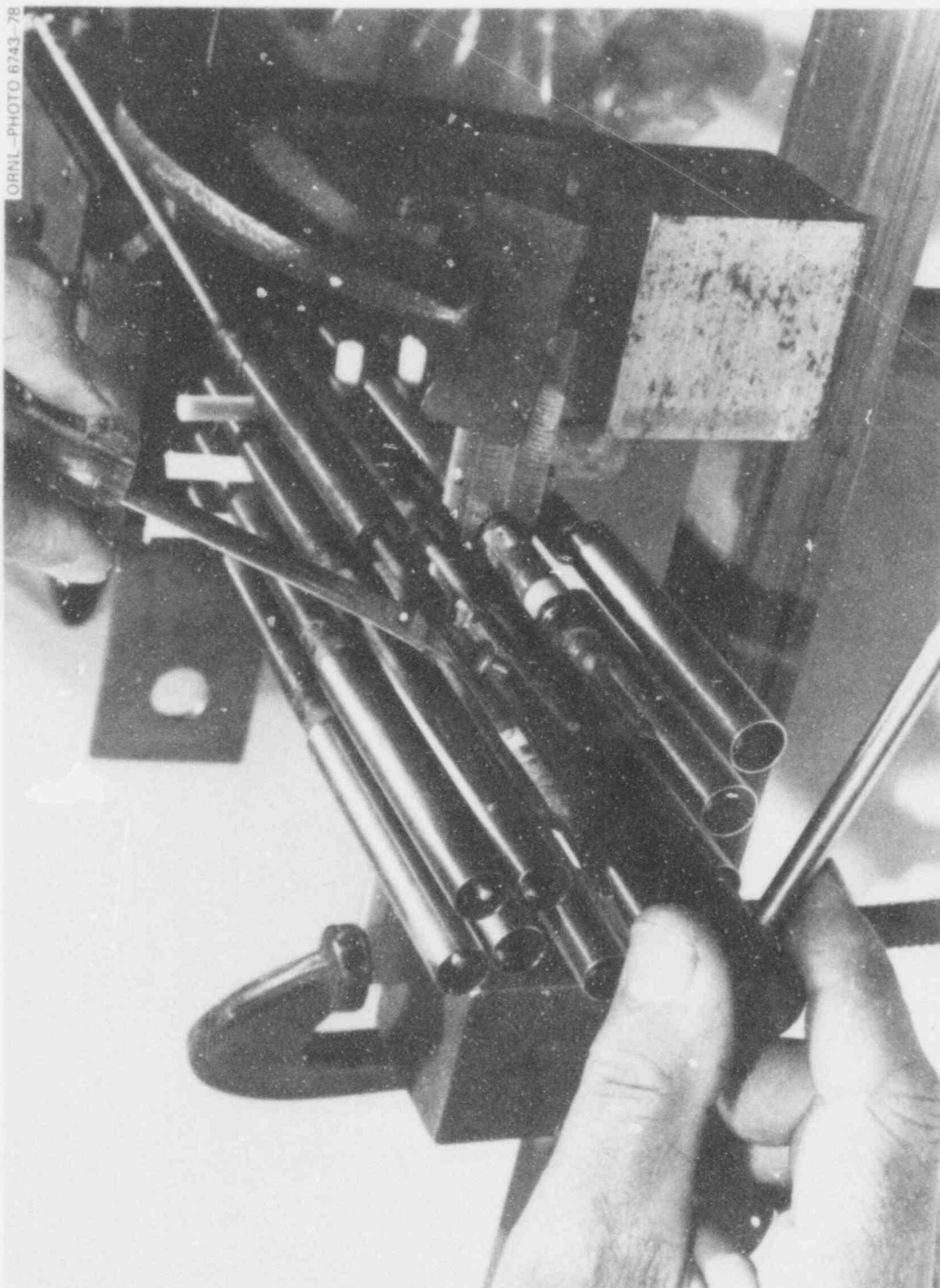
Fig. 4.2. Fracturing of ceramic insulator for removal of B-3 lower gland. Protective shields cover exposed ends to reduce possibility of thermocouple damage.
