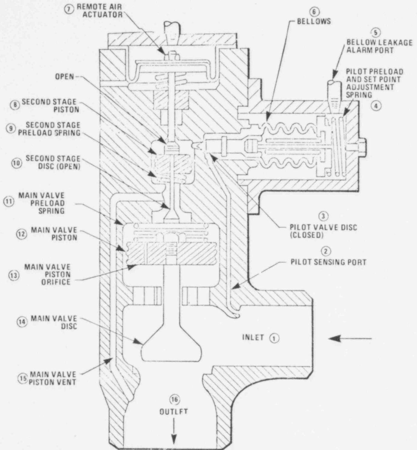
FIGURE 7 Safety-Relief Valve (External Actuation)
