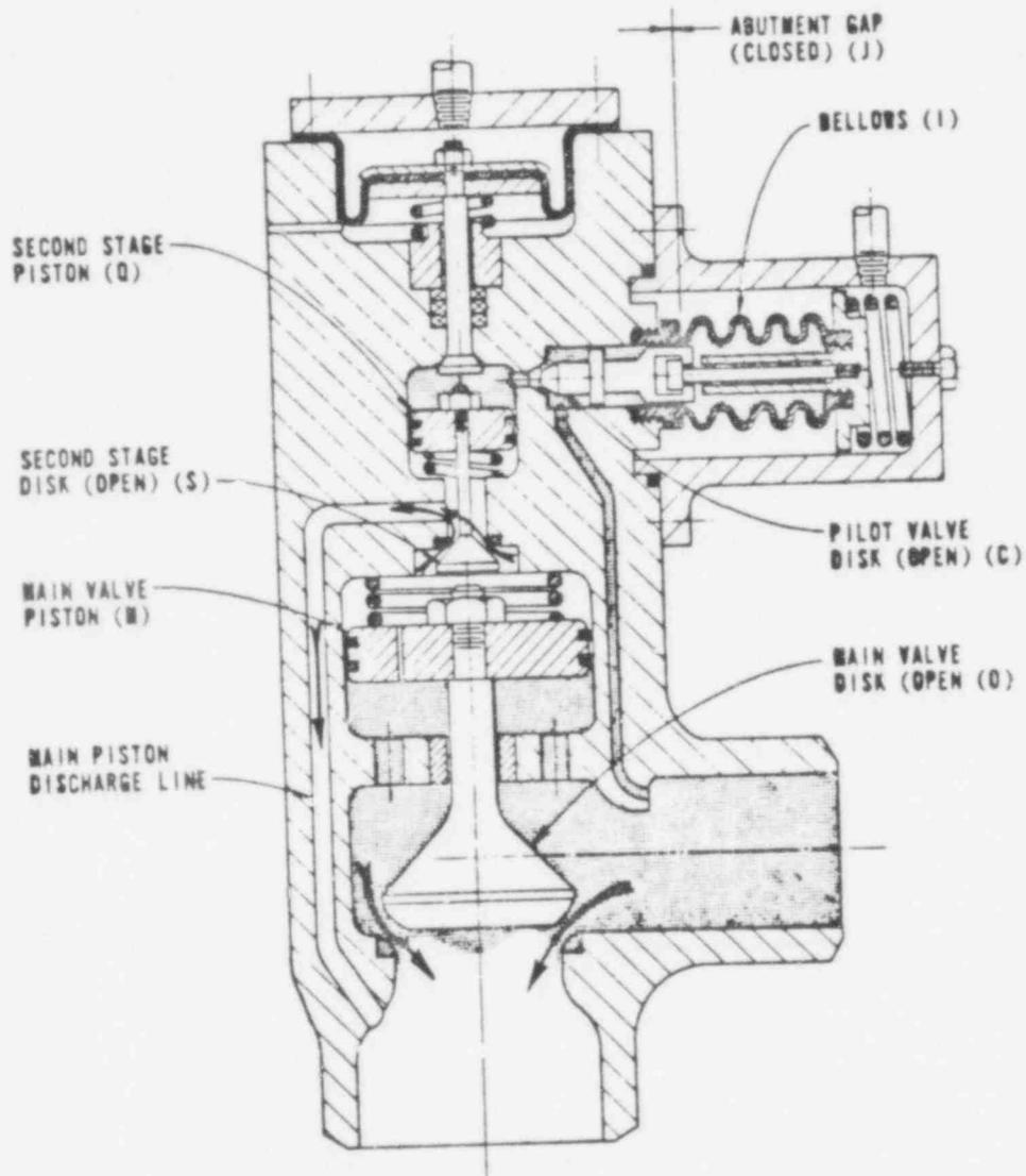
FIGURE 6 - Operational Diagram of Three-Stage Pilo.-Operated Pressure Relief Valve in Open Position.
