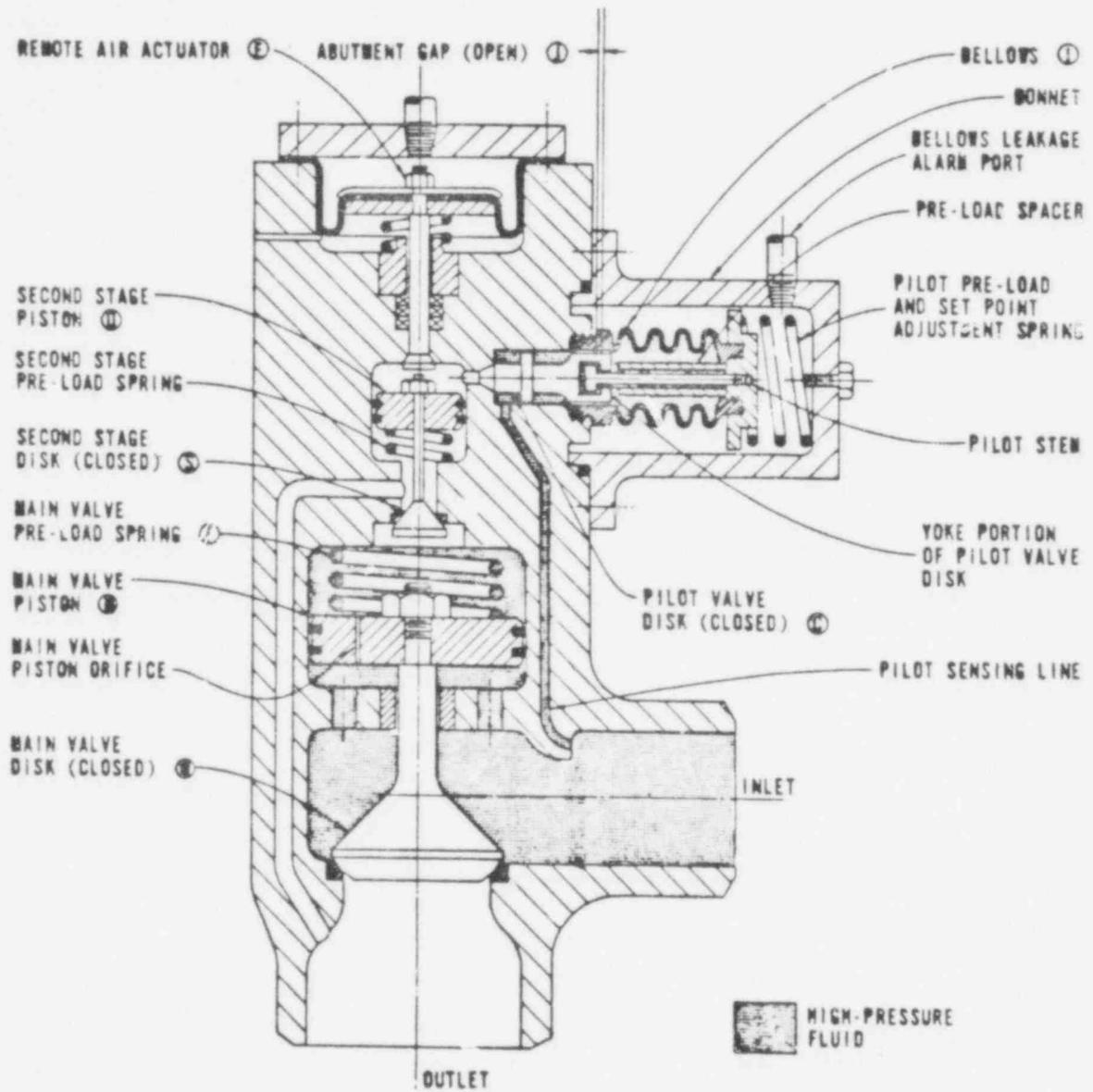
FIGURE 5 - Operational Diagram of Three-Stage Pilot-Operated Pressure Relief Valve in Closed Position.
