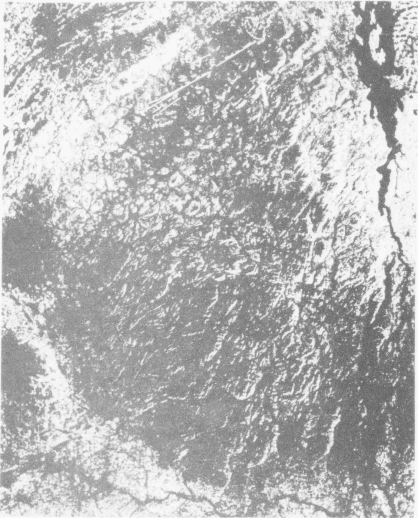
Figure 1 - Landsat - 1 mosaic of the Adirondack Mountains region, made from the imagery of October 10 and 11, 1972, band 7. East-northeast-trending linear features in the northern Adirondacks which are discussed in this report are labeled A-E.
