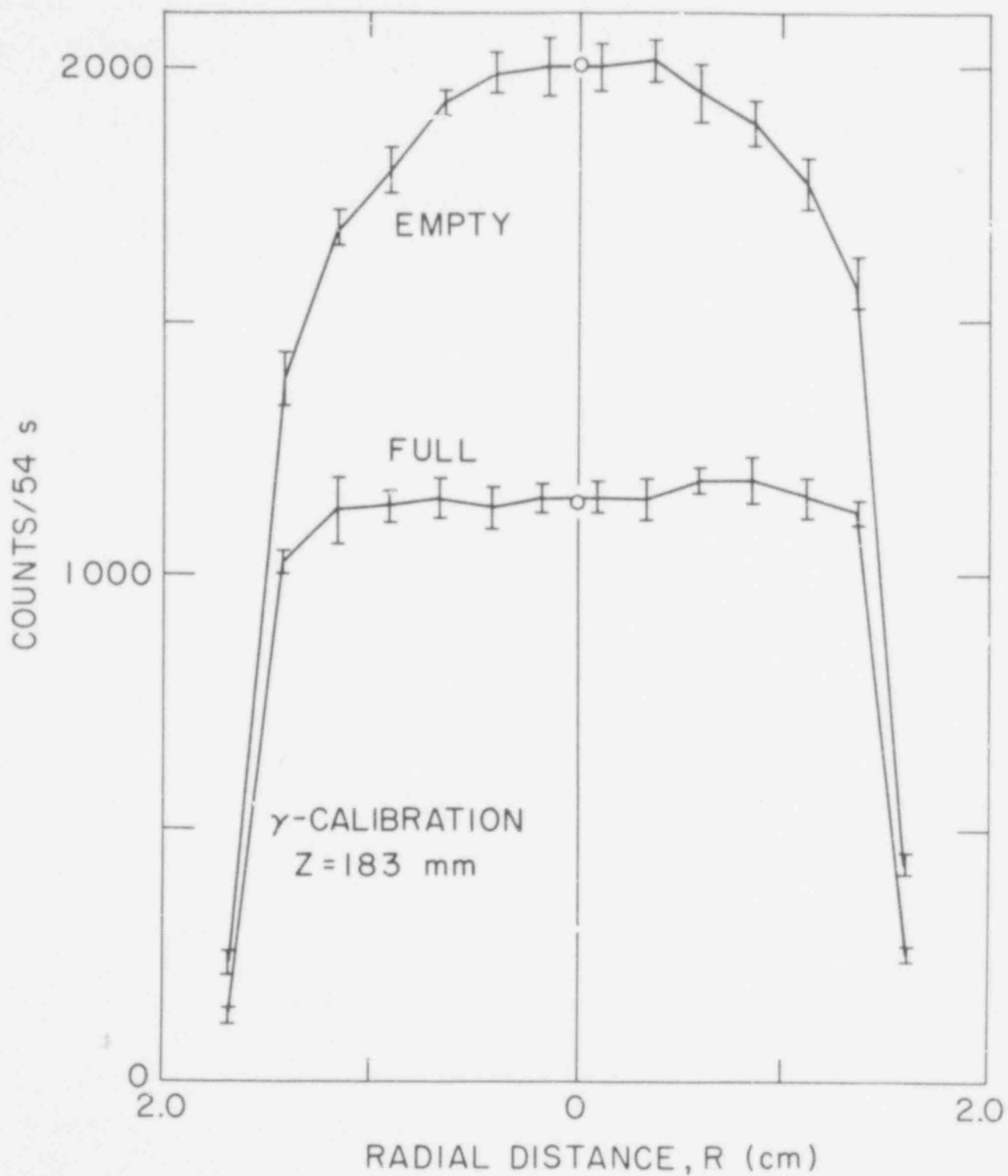
Figure 4.3 Calibration of the Test Section Both Empty (Air) and Full of Water as a Function of Radial Distance at a Fixed Axial Position (BNL Neg. No. 3-1020-79)
