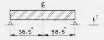
Given the foundation acceleration,  $\ddot{\mu}$ , the acceleration response amplitude,  $\ddot{x}$ , of the lid is found as:
