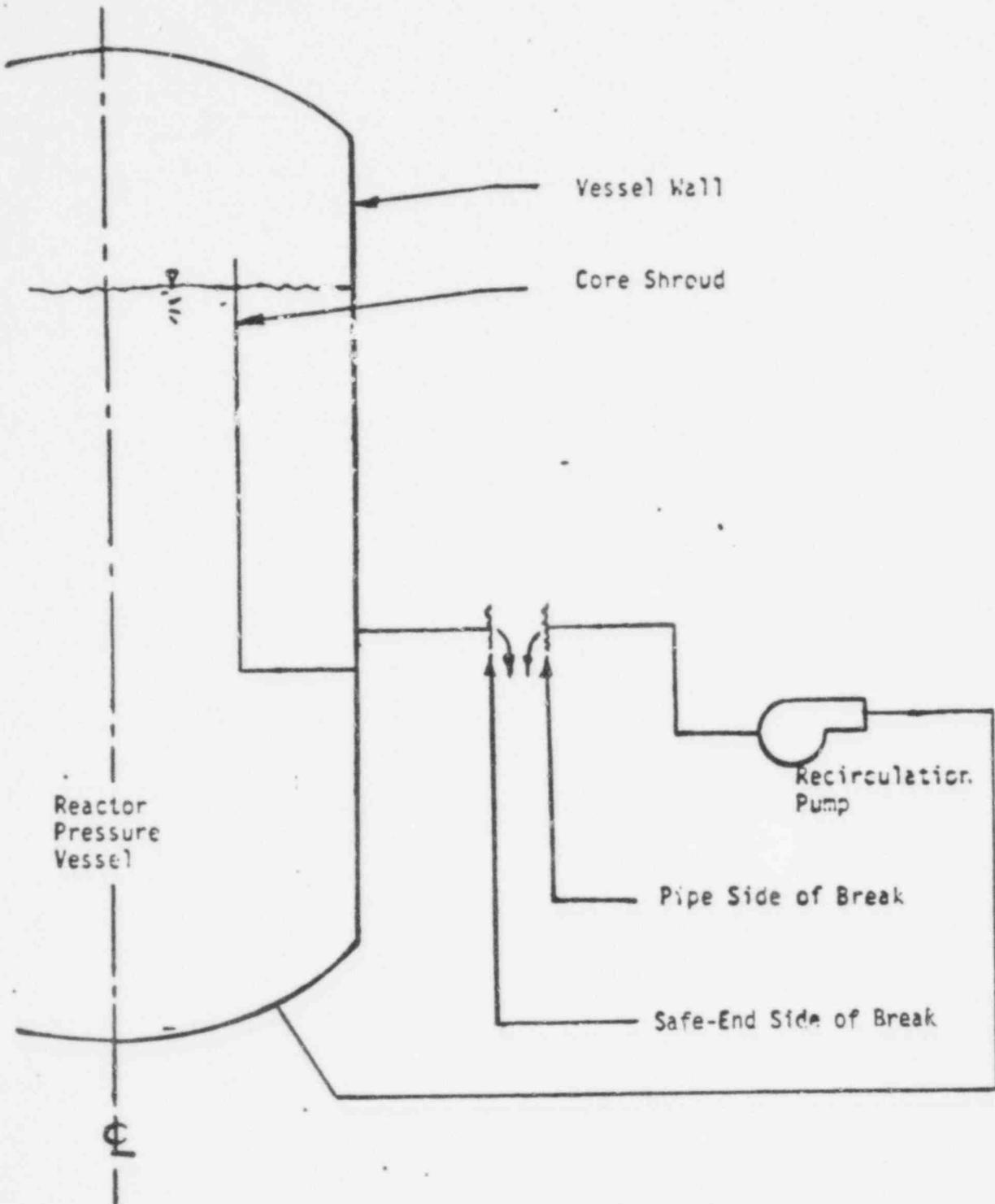
Figure - 10 Recirculation Line Break Location (BWR 2)
