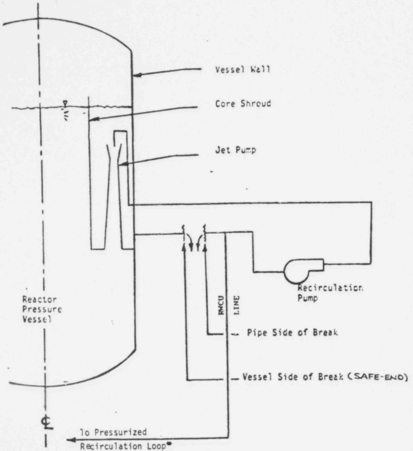
Figure - 11 Recirculation Line Break Location (BWR's 3,4 & 5)
