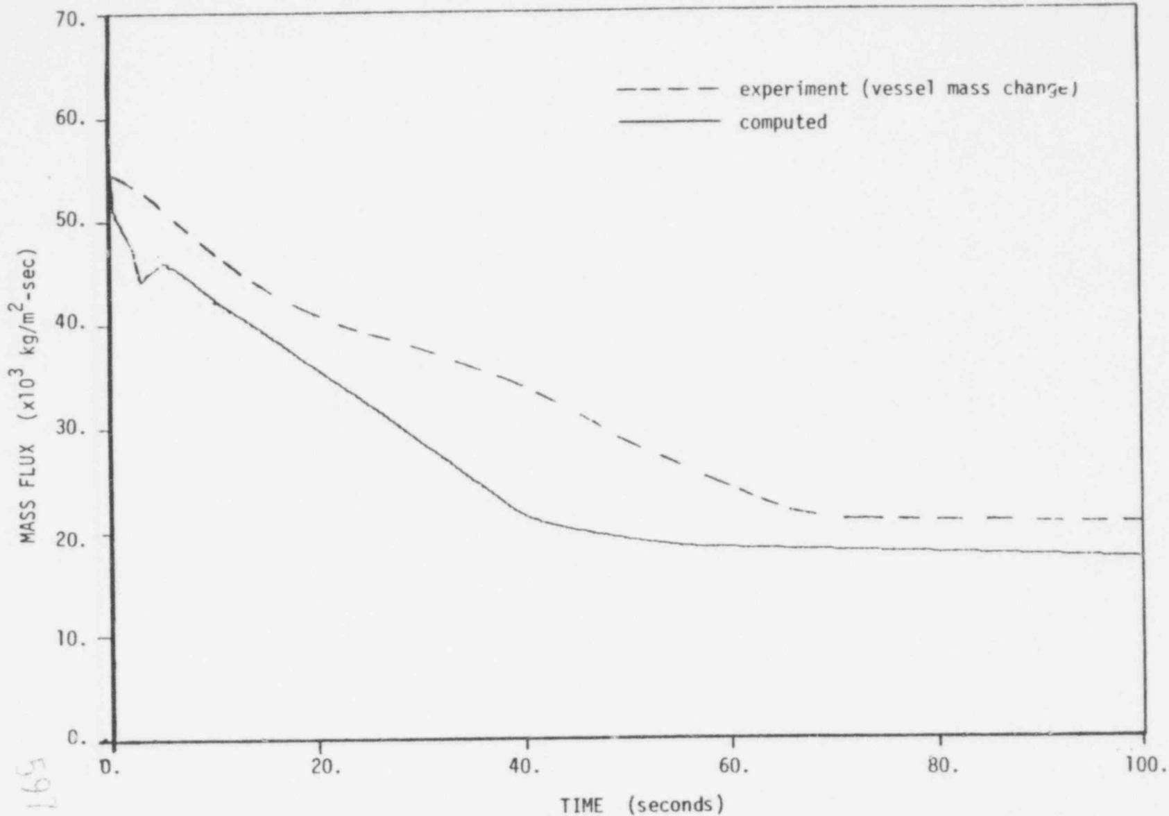
Figure 3 COMPARISON OF COMPUTED AND MEASURED MASS FLUX HISTORIES FOR MARVIKEN TEST NO. 1 (15 C SUBCOOLING), USING A QUASI-STATIONARY ISENTROPIC (IHE) DISCHARGE FLOW MODEL
