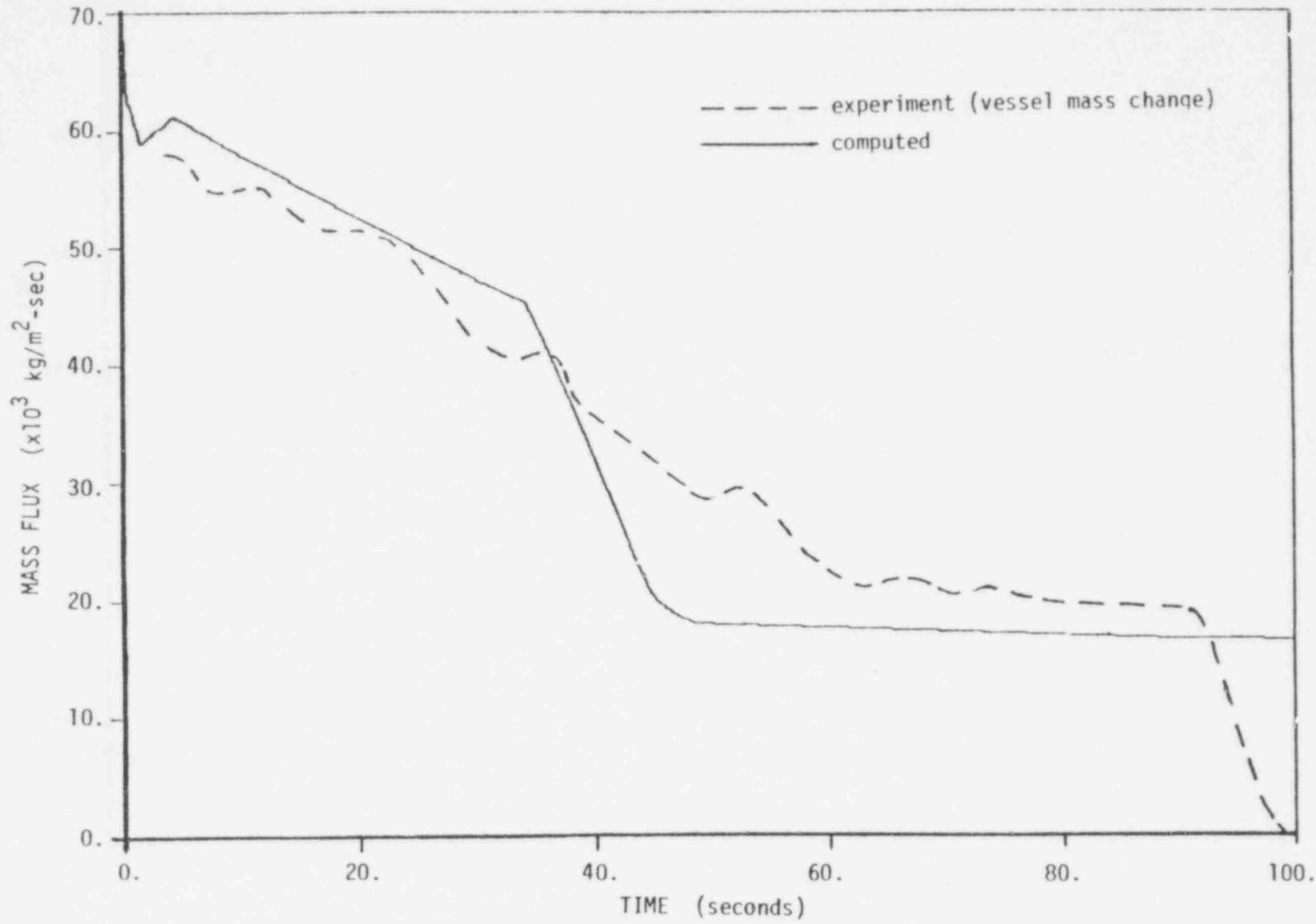
Figure 4 COMPARISON OF COMPUTED AND MEASURED MASS FLUX HISTORIES FOR MARVIKEN TEST NO. 2 (30 C SUBCOOLING), USING A QUASI-STATIONARY ISENTROPIC (IHE) DISCHARGE FLOW MODEL
