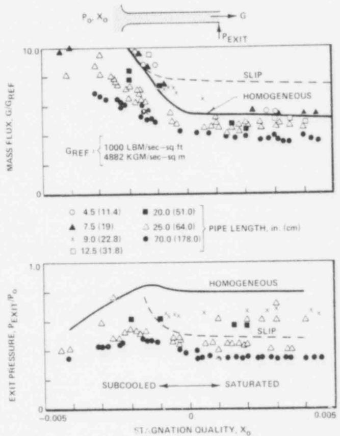
Fig.4 Blowdown rates and exit pressures of Sozzi and Sutherland (7) at 70 atmospheres
