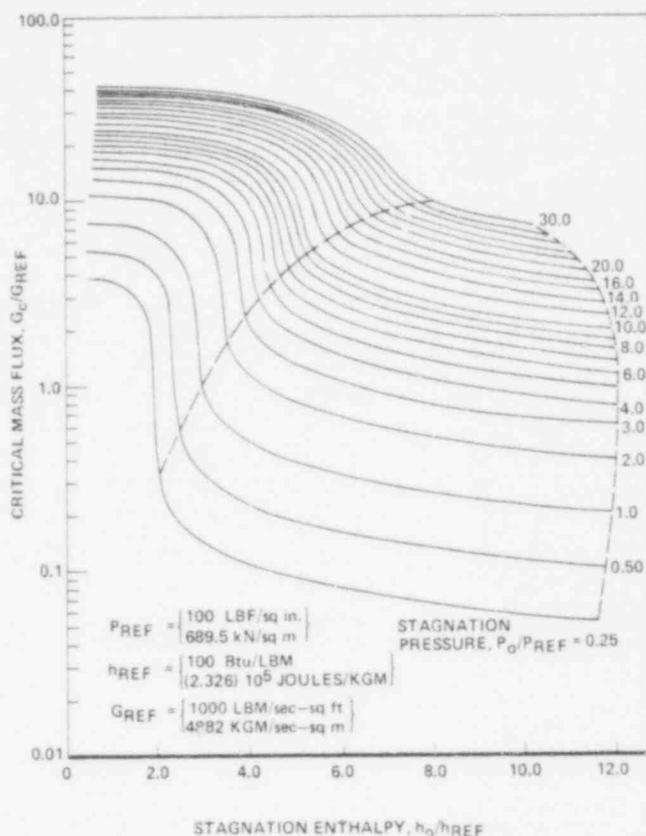
Fig.1 Critical mass flux - homogeneous, equilibrium steam-water
