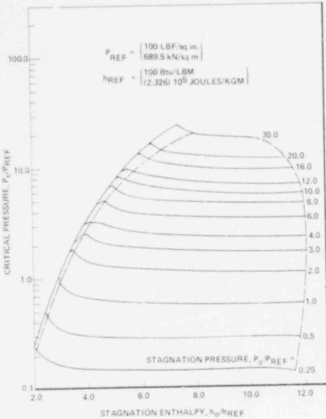
Fig.2 Critical pressure - homogeneous, equilibrium steam-water
