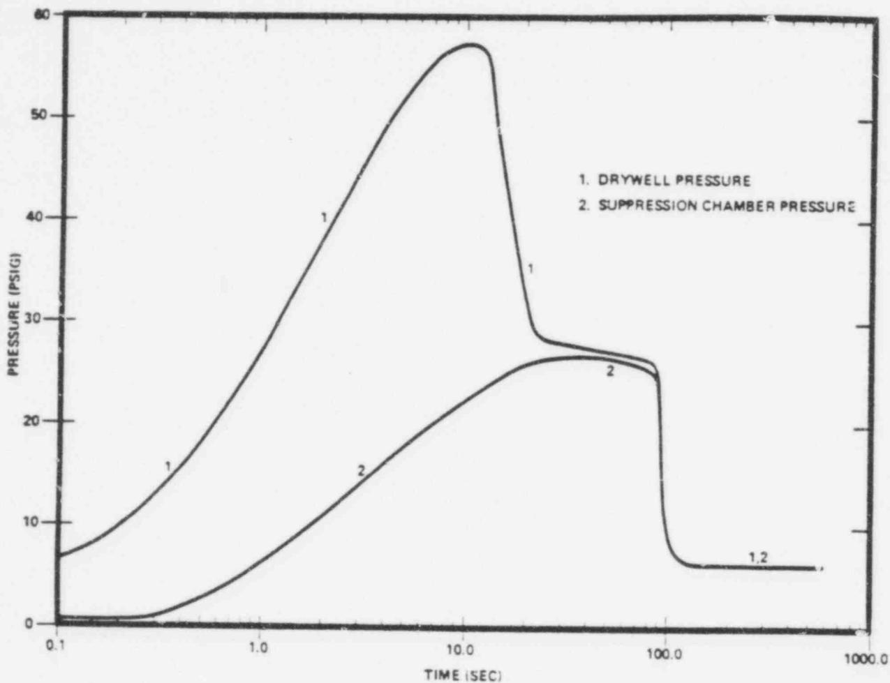
Figure 1 TYPICAL MARK I CONTAINMENT RESPONSE TO A RECIRCULATION LINE BREAK
