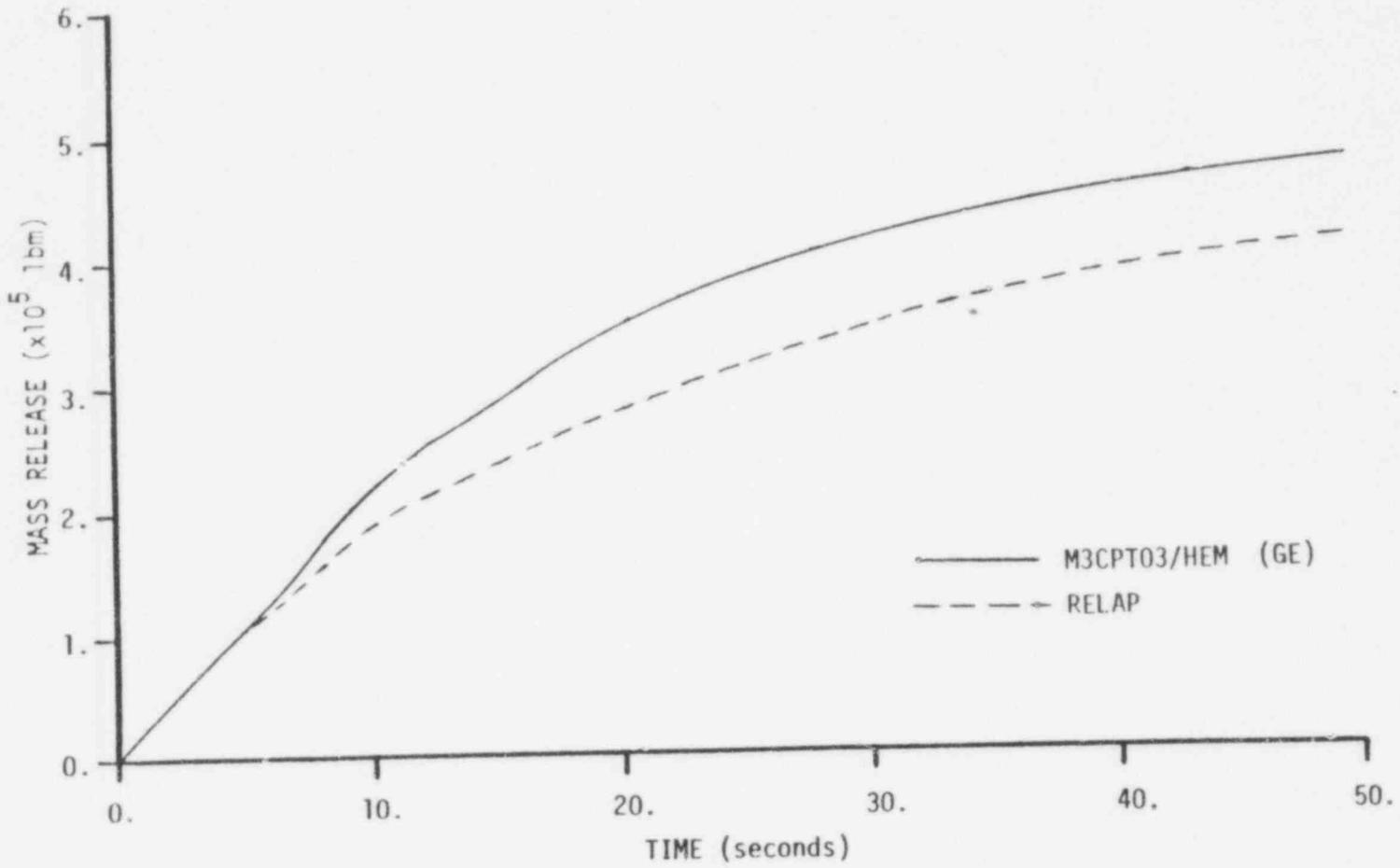
Figure 5 INTEGRATED MASS RELEASE
