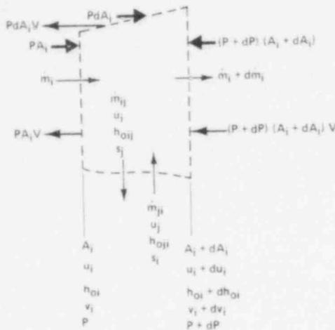
Fig.A-1 Control volume moving with disturbance
