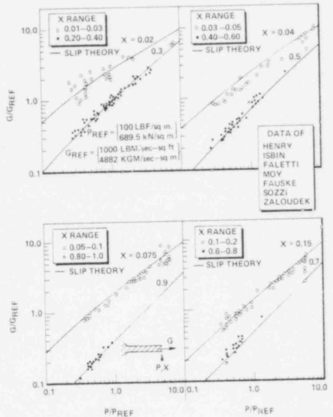
Fig.8 Critical flow properties at pipe exit
