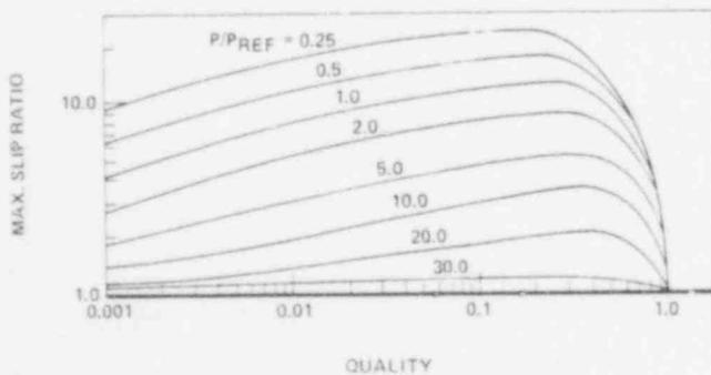
Fig.3 Critical flow states - slip model
