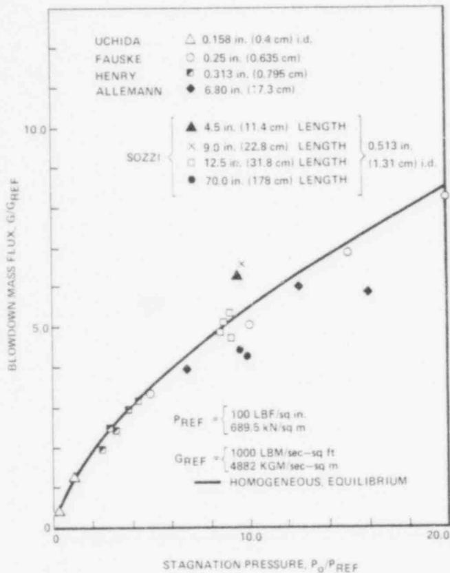
Fig.5 Blowdown rate of saturated water
