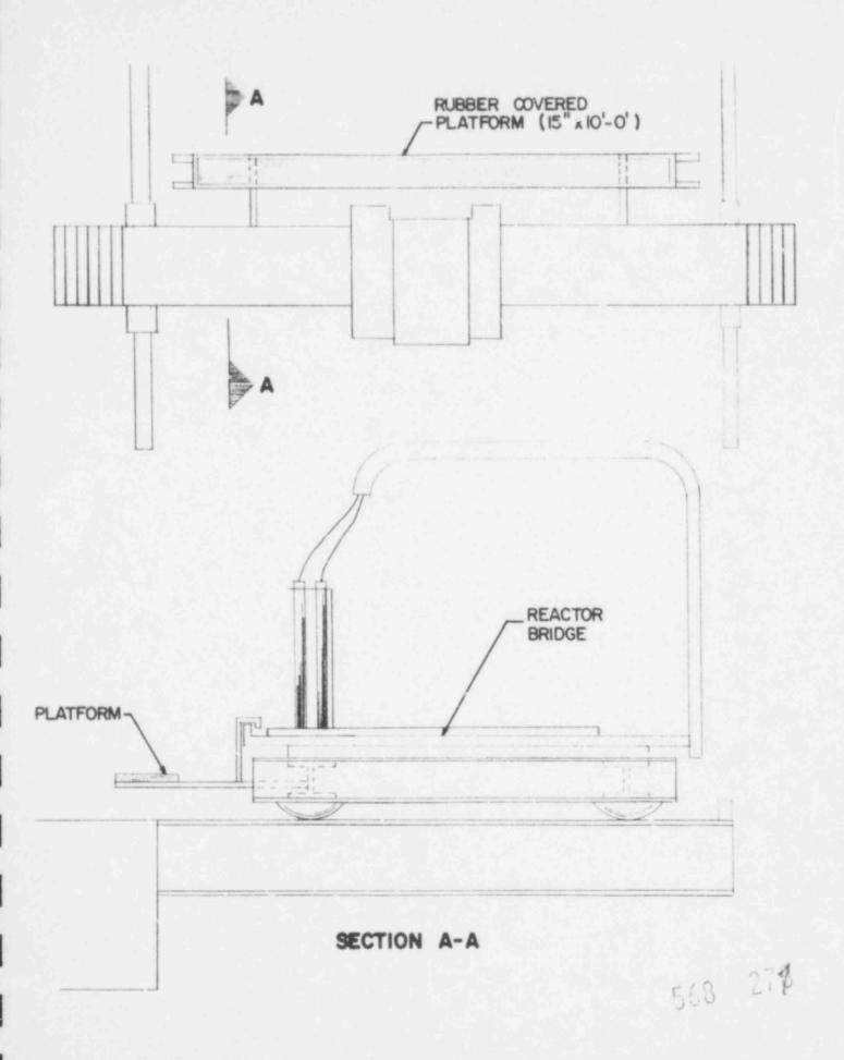
FIGURE 2. REACTOR BRIDGE WORK PLATFORM
