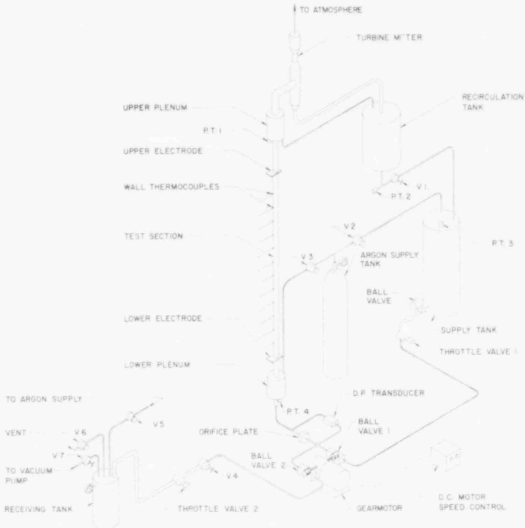
Fig. I.14. Schematic of Reflood Test Facility with Ball-valve System. ANL Neg. No. 900-78-909 Rev. 1.
