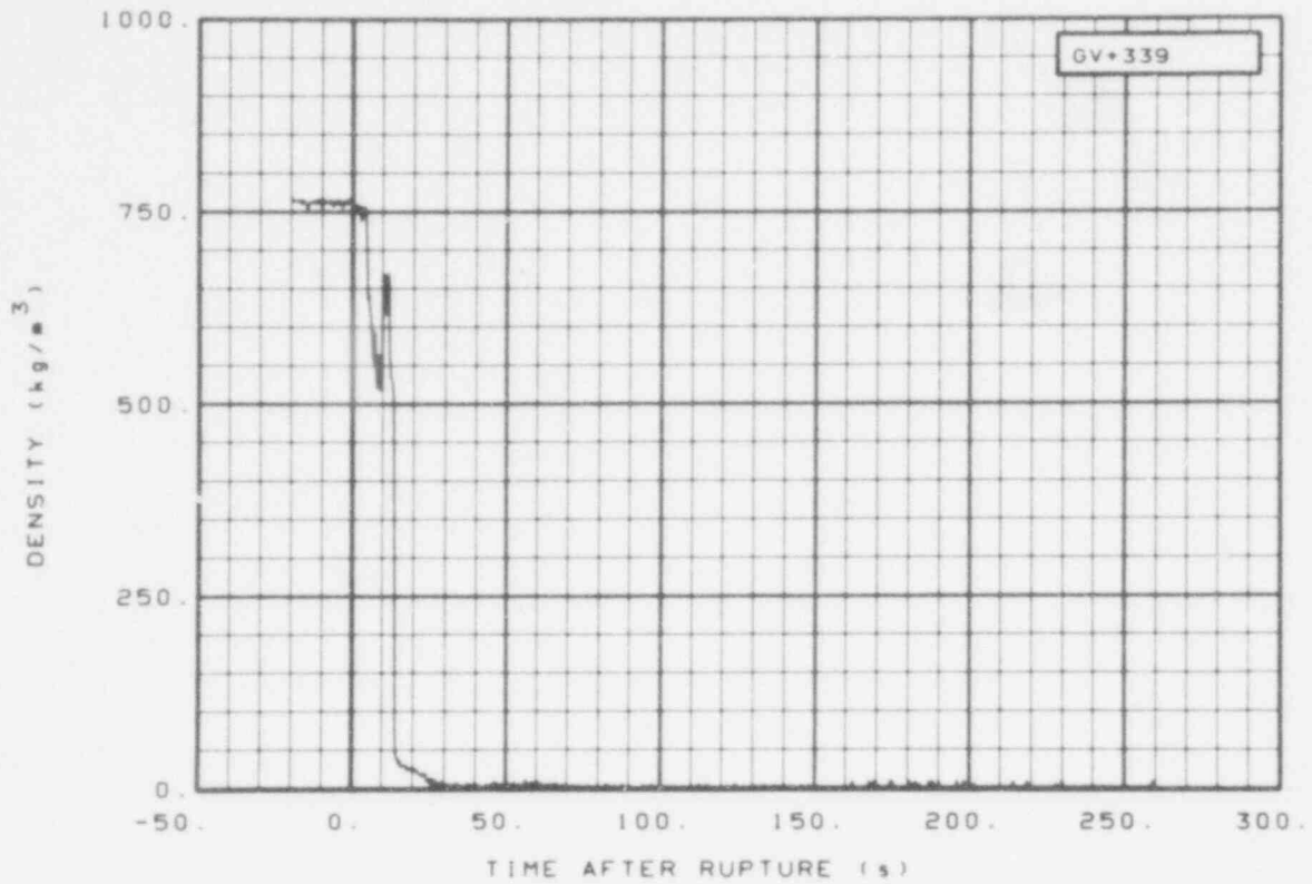
Fig. 261 Density in vessel (GV +339), from -20 to 260 s.
