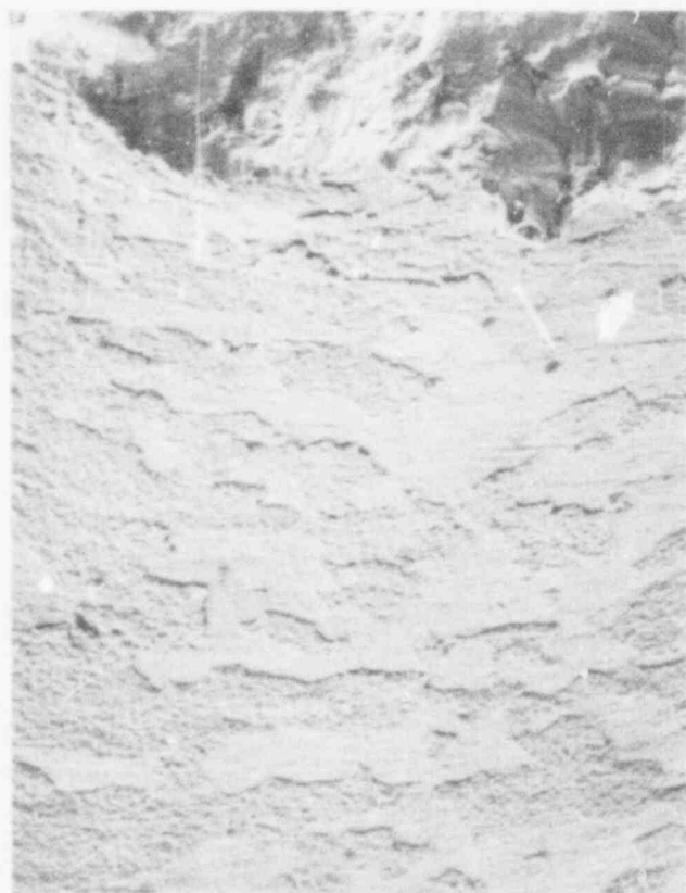
Figure 2.12. Scale spallation on surface of an Incoloy-800H specimen (MNF-194) thermally aged in HTGR helium for 3000 hours at 760^{\circ}\text{C} ( 1400^{\circ}\text{F} ) and tested in HTGR helium at an alternating stress of 158.6\text{ MPa} ( 23.0\text{ ksi} ) at 760^{\circ}\text{C} ( 1400^{\circ}\text{F} ); N_f is 5.5 \times 10^5 . Magnification 100X.
