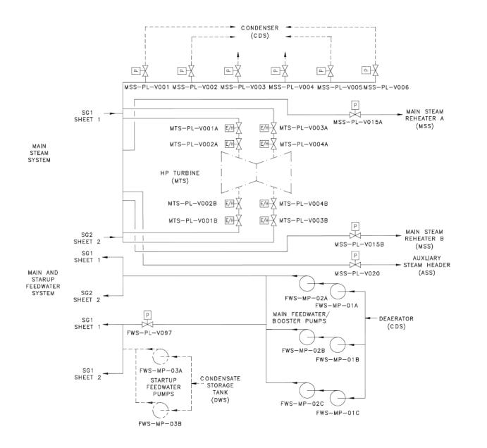
Figure 2.2.4-1 (Sheet 3 of 3) Steam Generator System
