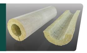
MinWool-1200 Preformed (PF) Pipe insulation is made of inorganic fibers derived from basalt, a volcanic rock. It is made with a thermosetting resin binder. PF Pipe insulation is a factory "V-grooved" mineral wool board that is formed to specific pipe sizes and provided in half cylinder sections with a variety of facing options.
