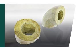
MinWool-1200 Mitered Fittings are made of inorganic fibers derived from basalt, a volcanic rock. It is made with thermosetting resin binder. These mitered and bonded fittings are for standard short and long radius and non-standard radius sweep elbows found in normal piping schemes. Fittings are manufactured from MinWool-1200 Preformed Pipe Insulation and mitered into precision segments.
