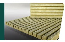
MinWool-1200 Precision Cut (PC) Pipe insulation is made of inorganic fibers derived from basalt, a volcanic rock. It is made with thermosetting resin binder. PC Pipe insulation (without adhesive) is a factory "V-grooved" mineral wool board manufactured to specific pipe or vessel sizes with a variety of facing options. It ships flat in 4 mil plastic and allows easy forming at the job site.
