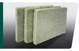
MinWool-1200 Flexible Batt insulation is made of inorganic fibers derived from basalt, a volcanic rock. It is made with a thermosetting resin binder. Advanced manufacturing technology ensures consistent product quality, with high fiber density and low shot content, for excellent performance in high-temperature, thermal control and fire-resistant applications.
