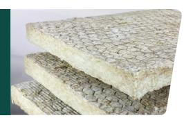
MinWool-1200 Metal Mesh Blanket (MMB) insulation is made of inorganic fibers derived from basalt, a volcanic rock, with a thermosetting resin binder. MMB is a mineral wool blanket available with a variety of metal mesh options mechanically applied to one or both surfaces.
