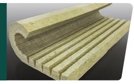
MinWool-1200 Field-Formed Pipe insulation is made of inorganic fibers derived from basalt, a volcanic rock. It is made with a thermosetting resin binder. Field-Formed Pipe insulation is a factory "V-grooved" mineral wool board with a unique contact adhesive in the grooves. It is manufactured to specific pipe sizes with a variety of facing options. It ships flat and allows for easy forming at the job site. Operating Temperature Limit: 1200°F (650°C)
