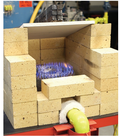
Figure 3: 13" x 13" sample of USG Sheetrock® Brand Firecode® C Gypsum Panel with a 16 lb. 13 oz. weight located in the center to dramatize the failure point.
