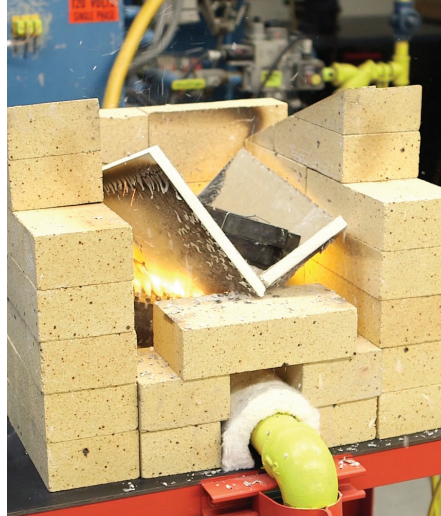
Figure 4: After 57 minutes, the USG Sheetrock® Brand Firecode® X Gypsum Panel collapsed due to the thermal exposure and the superimposed load.
