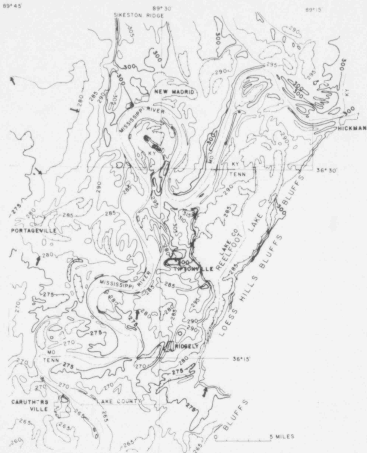
Figure 7- Detailed Configuration of the alluvial plain of the Mississippi River in the Study Area (in the east part of the Eastern Lowlands). This is an envelope over the surface that touches every 2000 feet of closer. Arrows are put on the 280 foot contour line to show its "Z" shaped trend.
