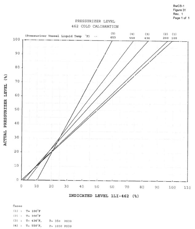
BwCB-1 Figure 31, Pressurizer Level 462 Cold Calibration, Revision 1
