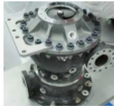
MSFC rocket engine fuel turbopump
