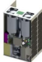
NASA Space Technology Mission Directorate-sponsored Cube Quest challenge for a flight-qualified cubesat (shown: cubesat with an Inconel 718 additively manufactured diffuser section, reaction chamber, and nozzle)
