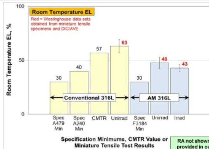
RA not shown here but is provided in our paper, AM values are in the range of 75-77% (measured via SEM fractographic images)
