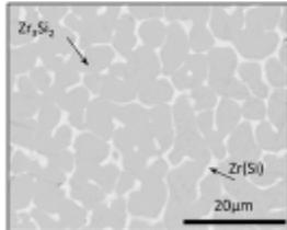
Back-scatter electron micrograph displaying the formation of  $Zr_3Si_2$ . Data validated by X-ray diffraction.
