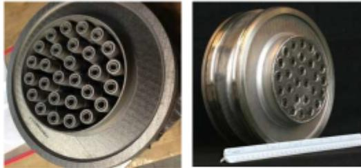
Using traditional manufacturing methods, 163 individual parts would be made and then assembled. But with 3D printing technology, **fewer parts (2)** were required, saving time and money and allowing engineers to build parts with **enhanced performance** and are **less prone to failure**.
