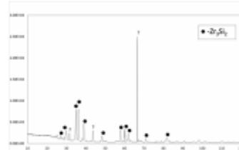
XRD analysis displaying the formation of  $Zr_3Si_2$  (includes resin mount)
