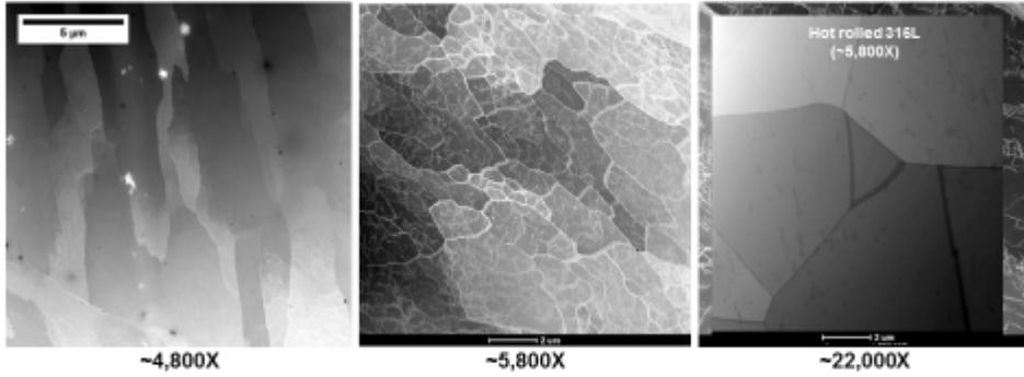
HAADF STEM of columnar grains containing subgrains
