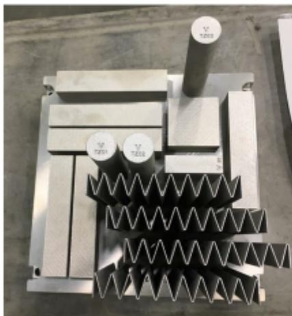
Small-scale production run, with additional materials testing samples:
