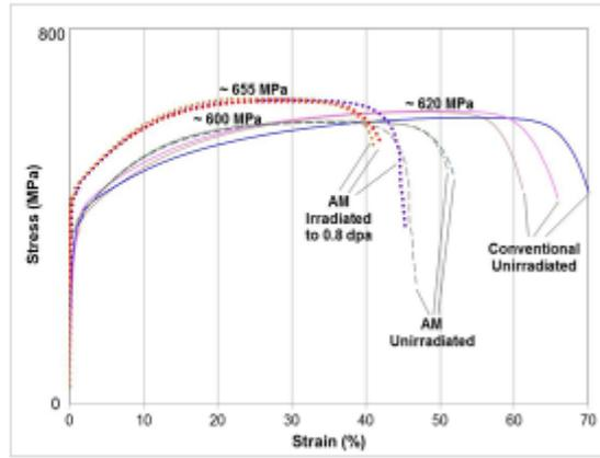
Stress strain curves for nine miniature specimens tested at room temperature
