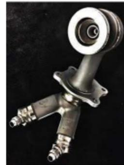
GE Leap Engine fuel nozzle. CoCr material fabricated by direct metal laser melting (DMLM), GE's acronym for DMLS, SLM, etc.
