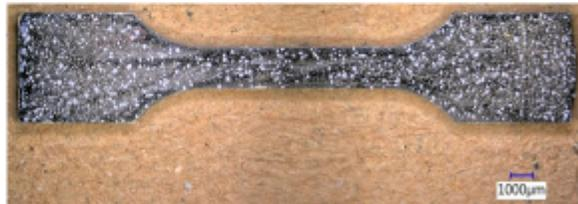
Placement of individual irradiated miniature tensile specimen onto small raised platform and example of good speckle pattern
