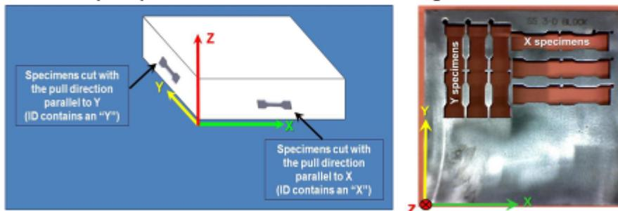
Wire EDM cutting of quads from AM 316L test block
