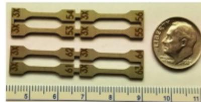
Miniature tensile specimen quads.
