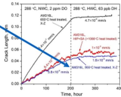
After high temperature annealing (above stress relief), retained unrecrystallized grains in the material may not significantly affect SCC behavior.
