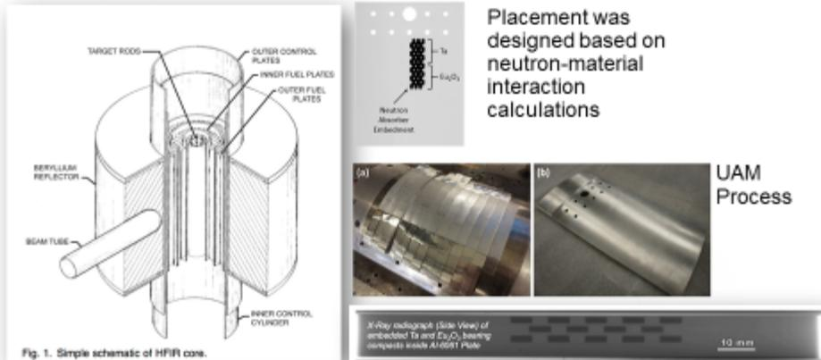
Placement was designed based on neutron-material interaction calculations
