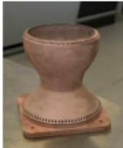
MSFC copper combustion chamber liner for extreme temperature and pressure applications
