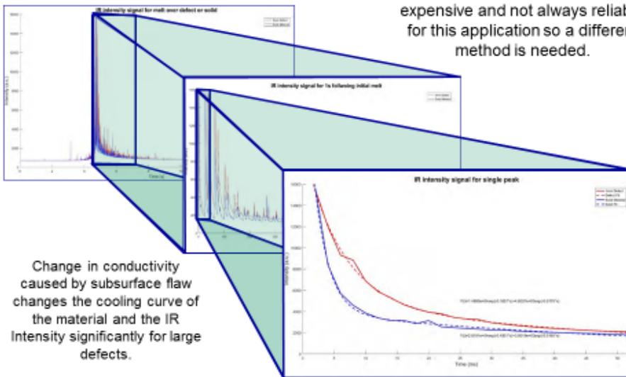
Change in conductivity caused by subsurface flaw changes the cooling curve of the material and the IR Intensity significantly for large defects.
