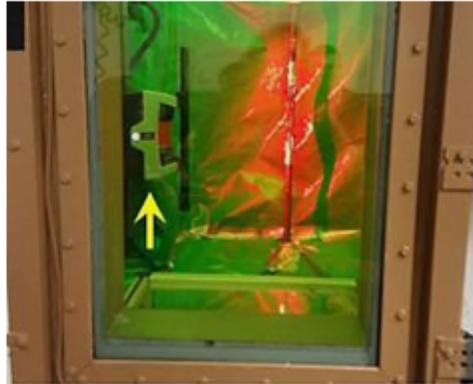
DIC system inside Low Level Hot Cell (marked with yellow arrow)
