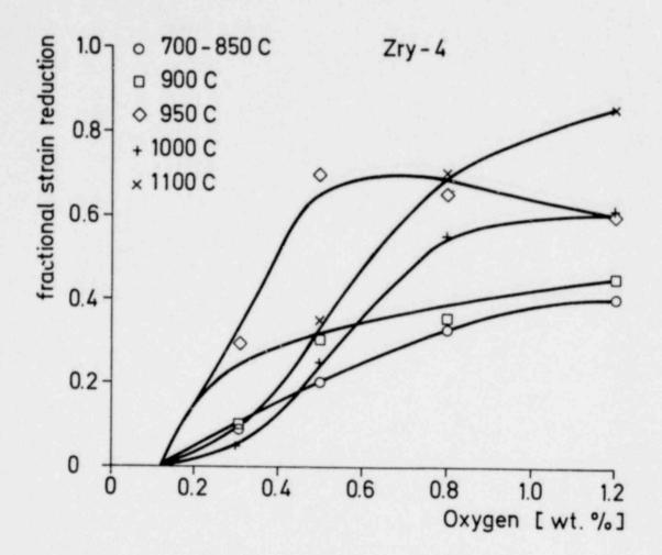
relative strain reduction due to steam oxidation for composite material
