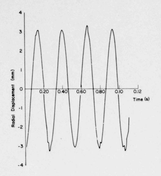
Fig. 7. Calculated radial displacement history of the core barrel bottom without the mass ring. The motion is initiated by prescribing the three components of the displacement field from solution of the Timoshenko beam equation. The frequency is 38.6 Hz.
