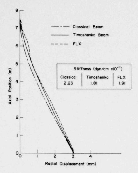
Fig. 9. Fundamental mode shape calculated with FLX compared with analytic results for solutions of the classical and Timoshenko beam equations.
