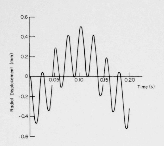
Fig. 8. Calculated radial displacement history of the core barrel bottom without the mass ring in response to a horizontal harmonic vessel acceleration  $\ddot{x} = 980 \cos 10 \pi t$ . The frequency is 37.9 Hz.
