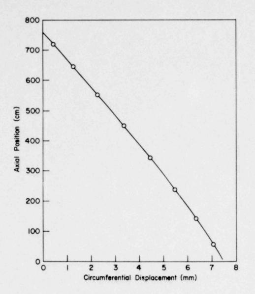
Fig. 10. Fundamental torsional mode shape calculated with FLX compared with the analytic result. The calculated torsional frequency is 22.0 Hz, which agrees precisely with the analytic solution.
