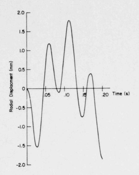
Fig. 6. Calculated radial displacement history of the core barrel bottom in response to a horizontal harmonic vessel acceleration  $\bar{x} = 980$  cos 10  $\pi t$ . The frequency is 17.6 Hz.
