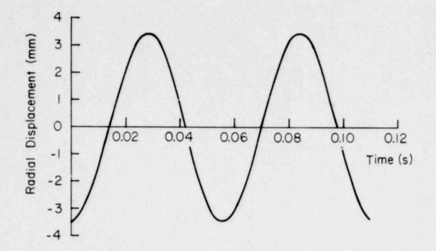
Fig. 5. Calculated radial displacement history of the core barrel bottom after release from a static configuration in which the core barrel bottom is deflected 3.5 mm. The frequency is 17.9 Hz.
