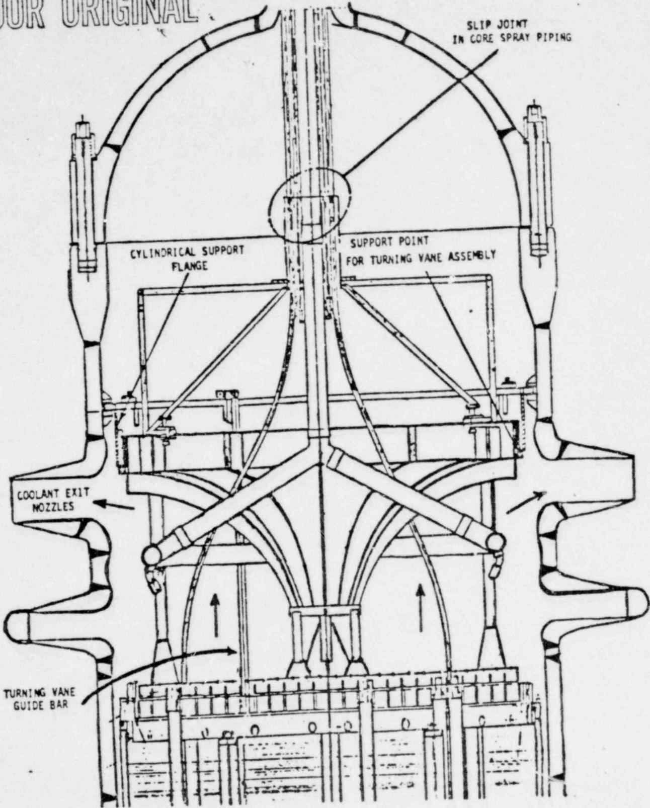
FIGURE 2 TURNING VANE ASSEMBLY INSTALLED IN THE PRESSURE VESSEL.
