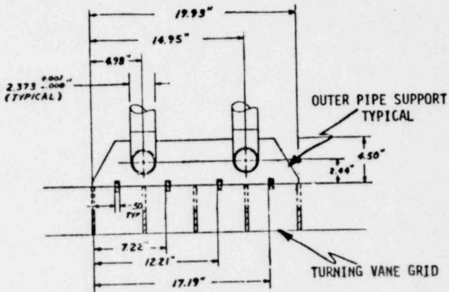
FIGURE 5 TYPICAL PERIPHERAL SUPPORT FOR GRID HEADER PIPE.
