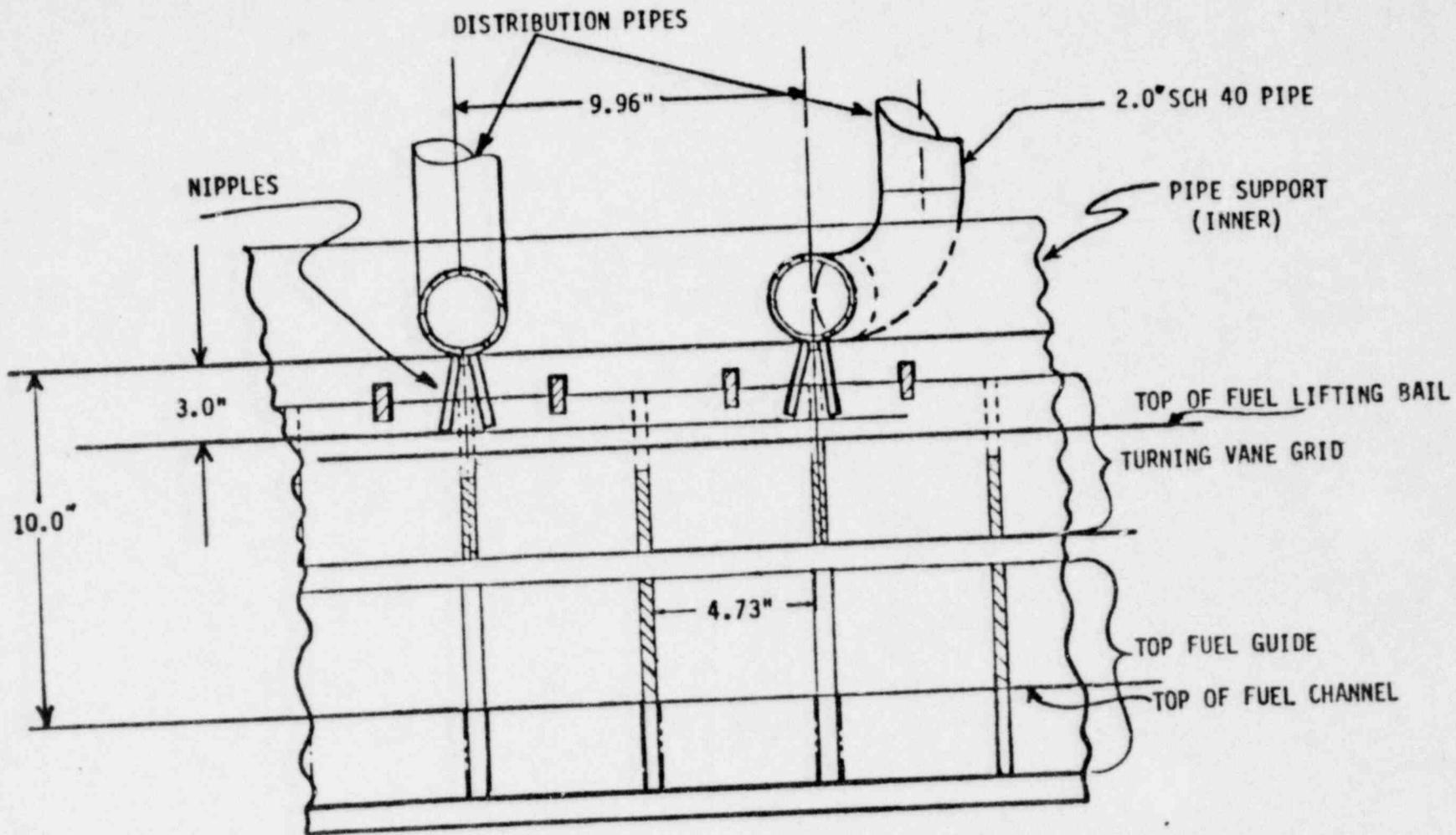
FIGURE 8 DETAIL SHOWING RELATIONSHIP OF HEADER PIPES AND NIPPLES TO THE TURNING VANE GRID, TOP FUEL GUIDE AND THE TOP OF THE FUEL CHANNELS.
