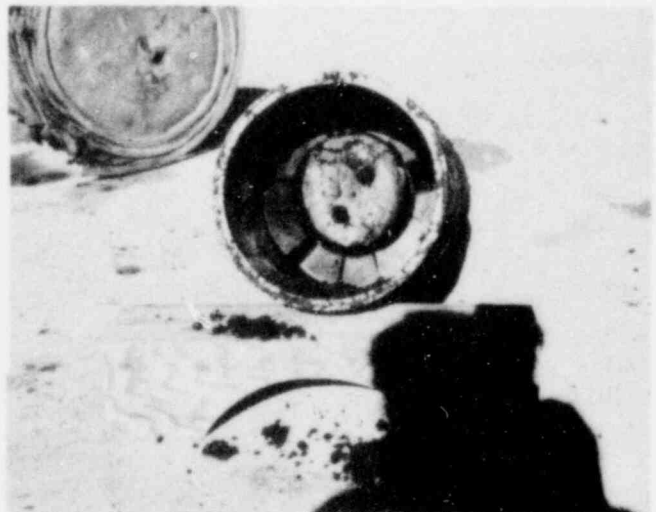
Figure 2.5.1.7-4. Load Spreader Showing Redwood and Internal Plug (Circular Plate Load Spreader Removed)
