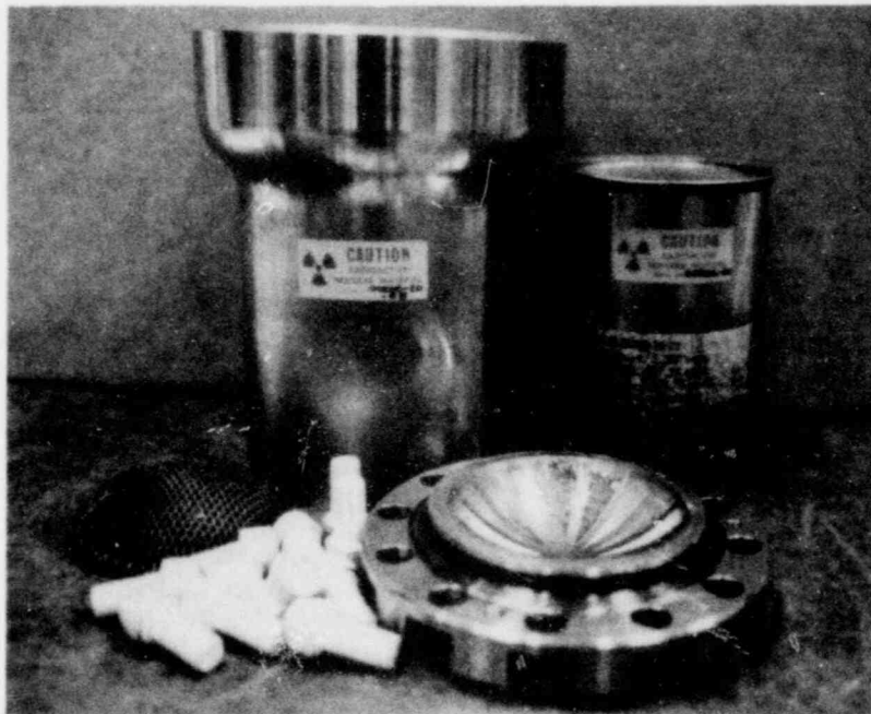
Figure 2.5.4.11-1. Disassembled TB-1 Following 10 CFR 71.A Tests
