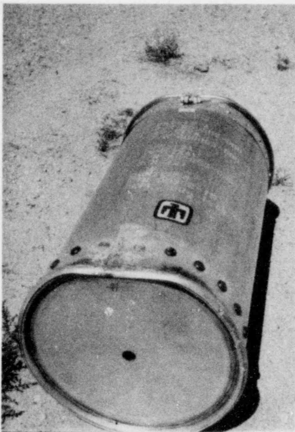
Figure 2.5.5.2-1. Damage From 30-ft Side Drop
