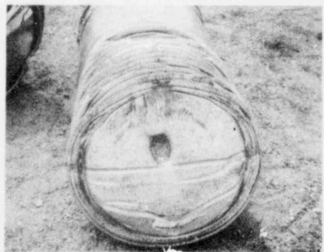
Figure 2.5.1.3-4. Puncture Test on Bottom-Corner-Impacted PAT-1
