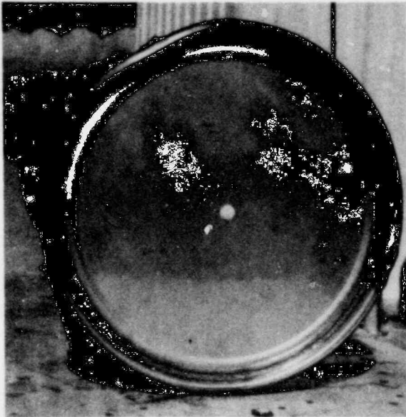
Figure 2.5.4.7-1. Damage From 4-ft Drop Test
