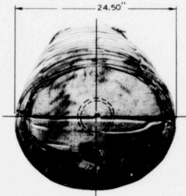
Figure 2.5.1. 1-15. Postimpact Measurements -- Bottom Corner (150°) Impact
