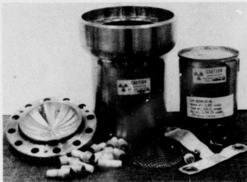
Figure 2.5.5.6-3. Disassembled TB-1, Post 10 CFR 71 Test, Showing Roll Crimp Closure and Epoxy Overbonding Intact
