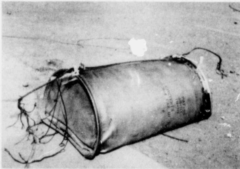
Figure 2.5.2.2-1. Cold (-40°F) Impact of Prototype PAT Package
