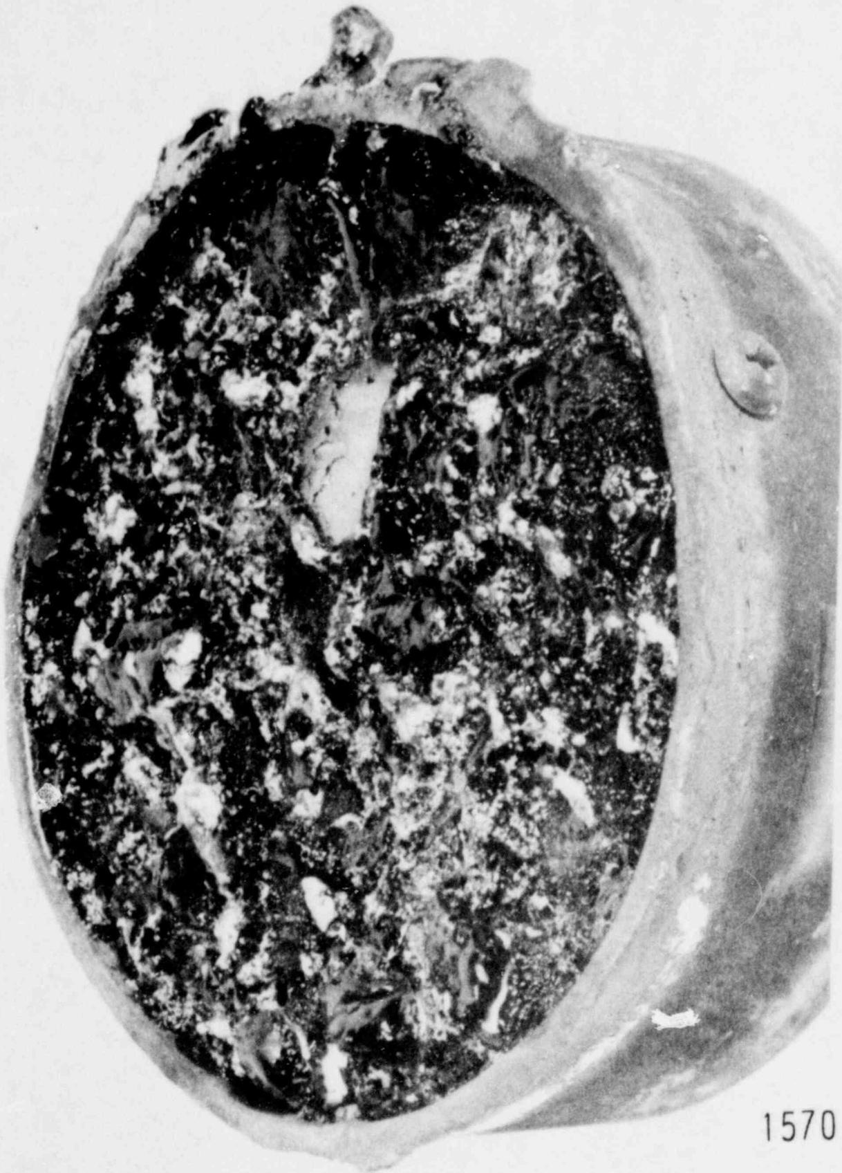
Figure D-6. Eroded Surface of Radiant Heat Test Sample RH7-4;
