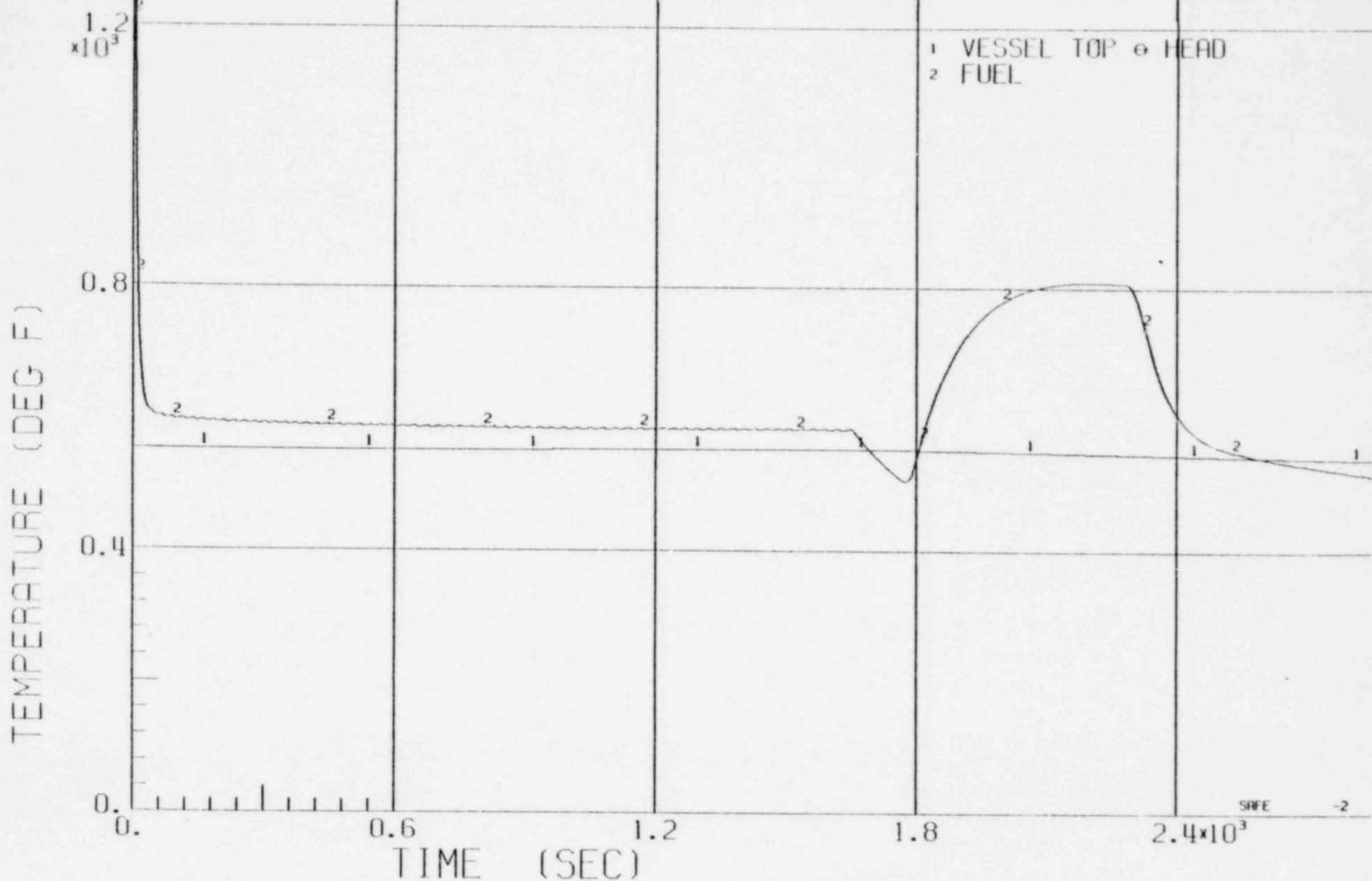
FIGURE 3.5.2.1-31.6 TEMPERATURE VS TIME FOR AN ISOLATION WITH ONE LPCI AVAILABLE, THREE RELIEF VALVES OPEN AT 600 SECONDS AFTER LI.
