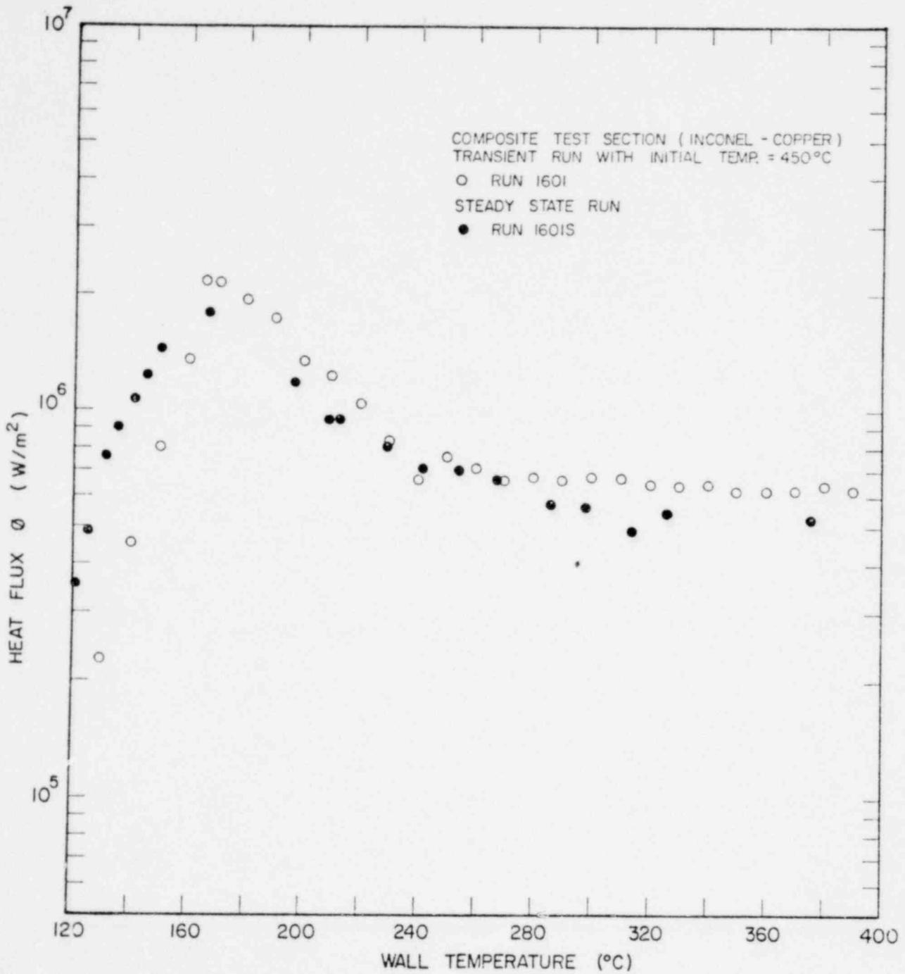
Fig. 2. Boiling Curves of Distilled Water for  $G = 136 \text{ kg/m}^2\text{s}$  and  $\Delta T_{\text{sub}} = 13.9^\circ\text{C}$
