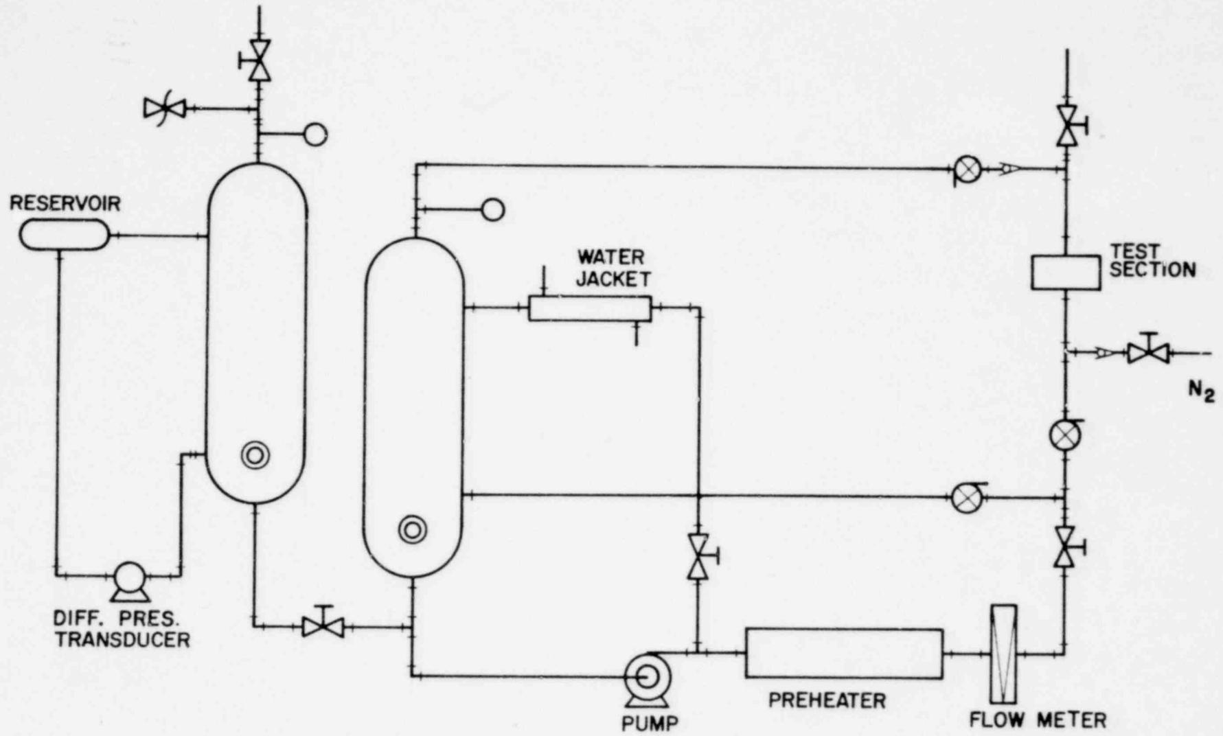
Fig. 26. Preliminary Design for Pressurized Loop
