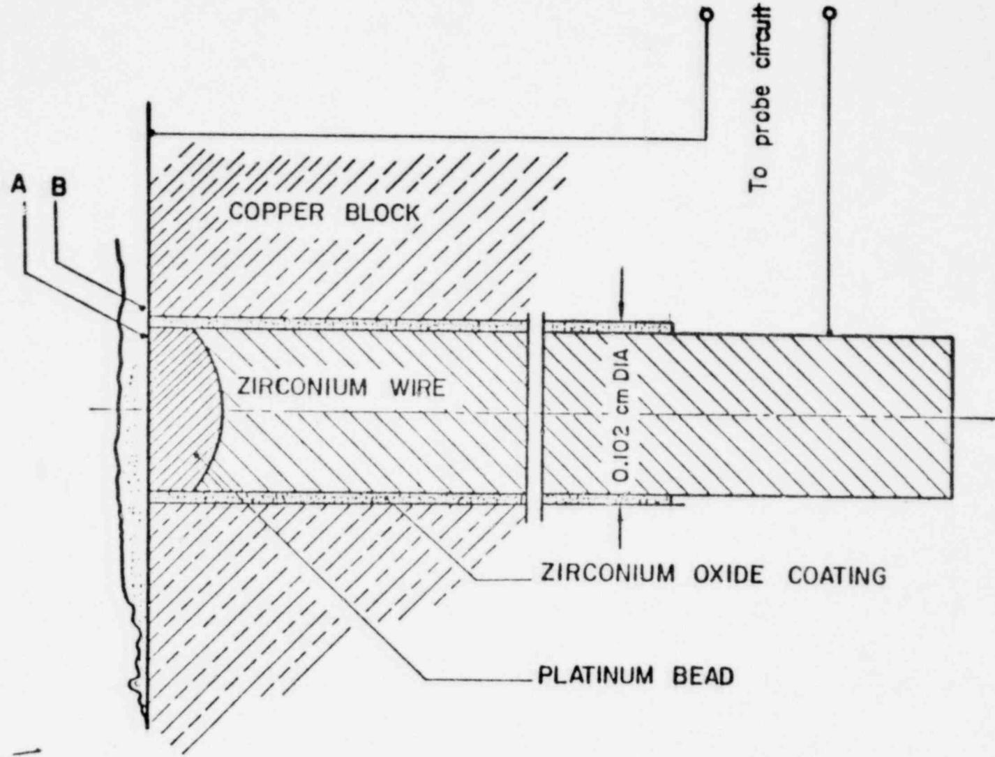
Fig. 1. Probe Configuration
