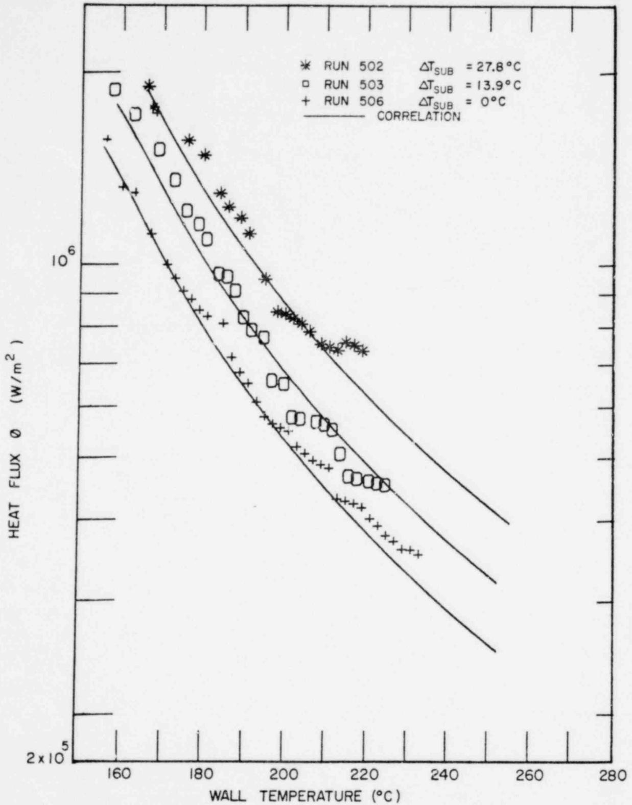
Fig. 19. Comparison of Copper Correlation with Transition Boiling Data for  $G = 136 \text{ kg/m}^2\text{s}$
