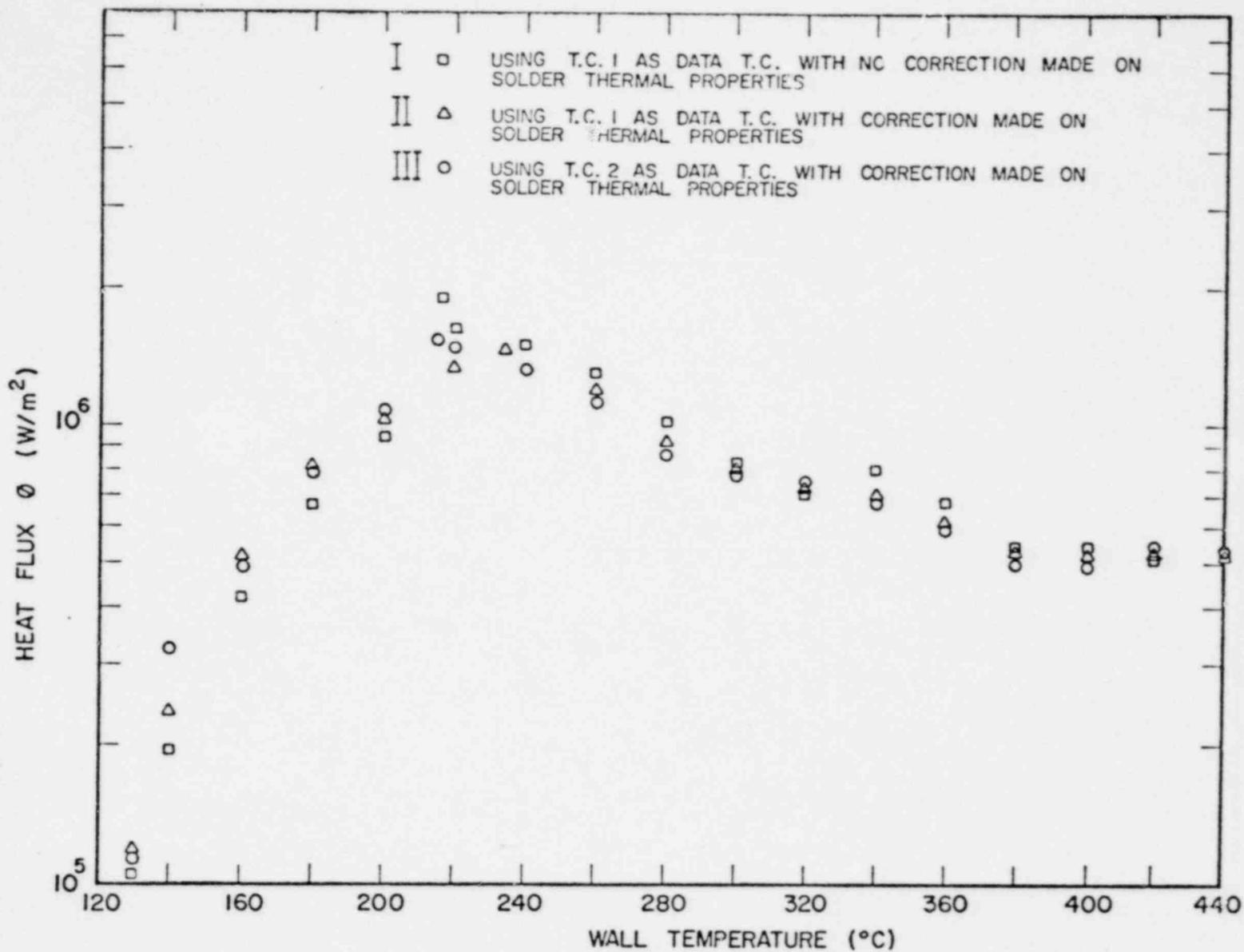
Fig. 8. Boiling Curve for Distilled Water, 1700 Run
