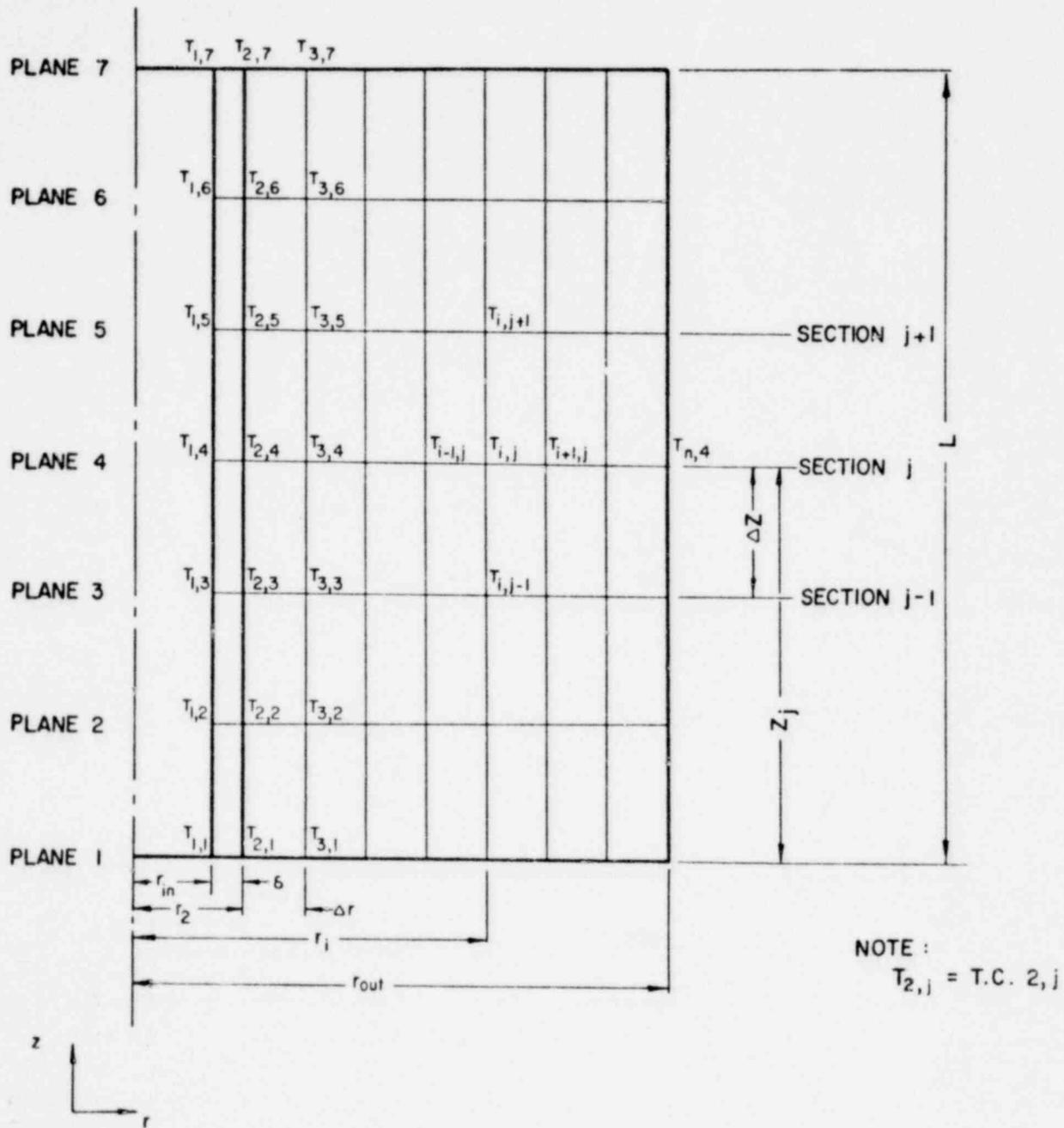
Fig. 2. Nodal Network for Two Dimensional Model in Composite Test Section
