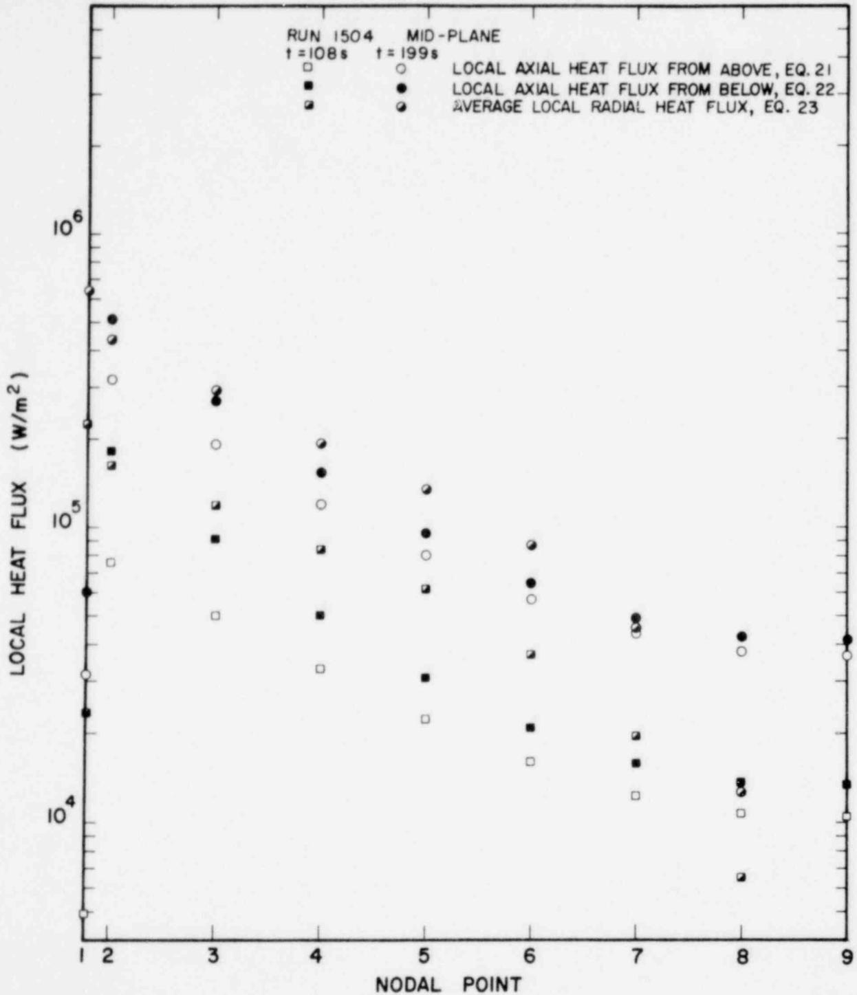
Fig. 5. Local Axial Heat Flux Distribution at Mid-Section for Inconel-Copper Composite Test Section for  $G = 136 \text{ kg/m}^2\text{s}$  and  $\Delta T_{\text{sub}} = 13.9^\circ\text{C}$  (Part II)
