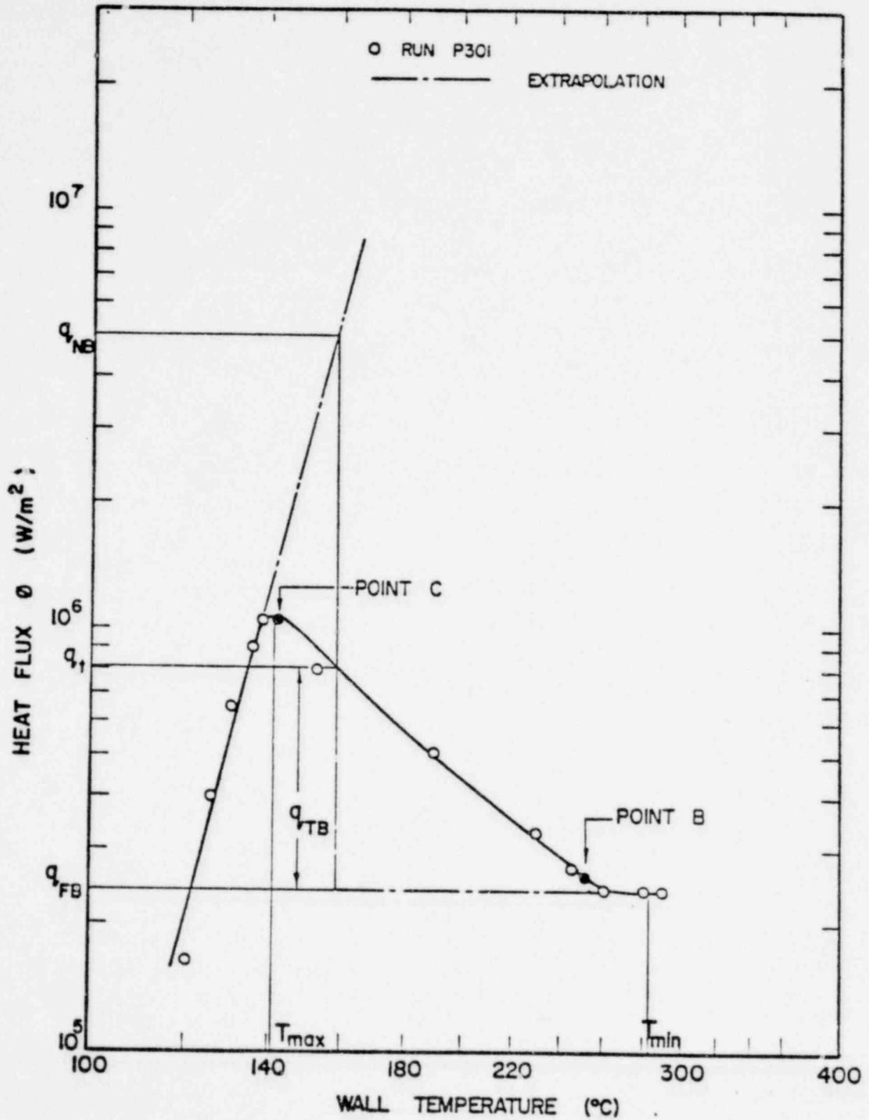
Fig. 4. Boiling Curve of Water for  $G = 68 \text{ kg/m}^2\text{s}$  and  $\Delta T_{\text{sub}} = 27.8^\circ\text{C}$
