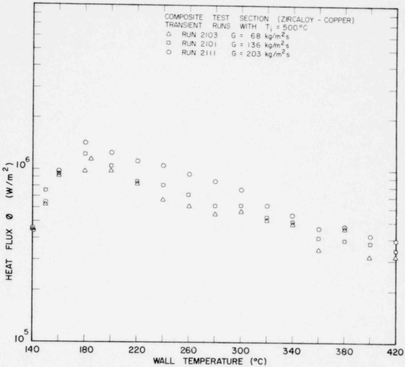
Fig. 13. Boiling Curves of Distilled Water, 2100 Run Series for  $\Delta T_{\text{sub}} = 13.9^\circ\text{C}$ , Using 1-D Model
