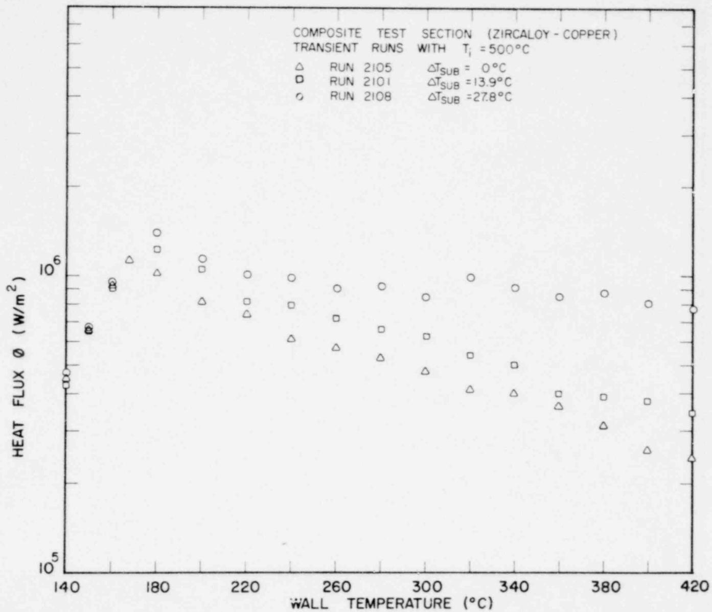
Fig. 12. Boiling Curves of Distilled Water, 2100 Run Series for  $G = 136 \text{ kg}/\text{m}^2\text{s}$ , Using 1-D Model
