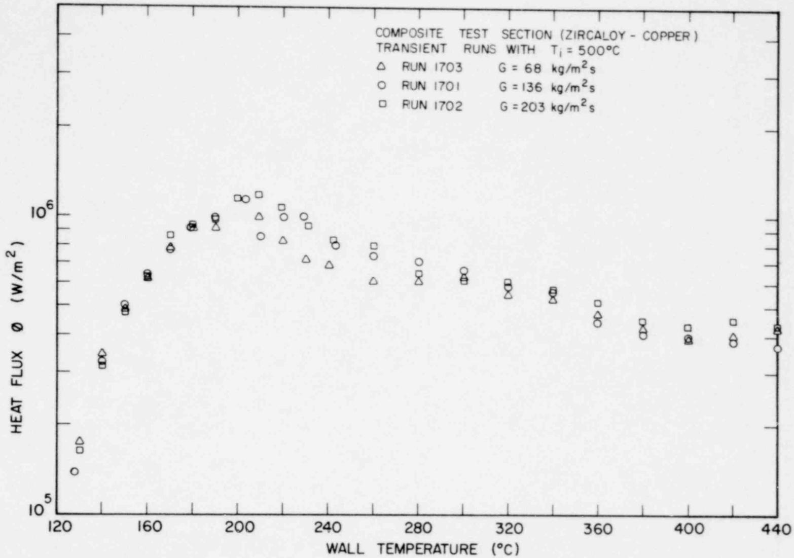
Fig. 9. Boiling Curves for Distilled Water, 1700 Run Series for  $\Delta T_{\text{sub}} = 13.9^\circ\text{C}$
