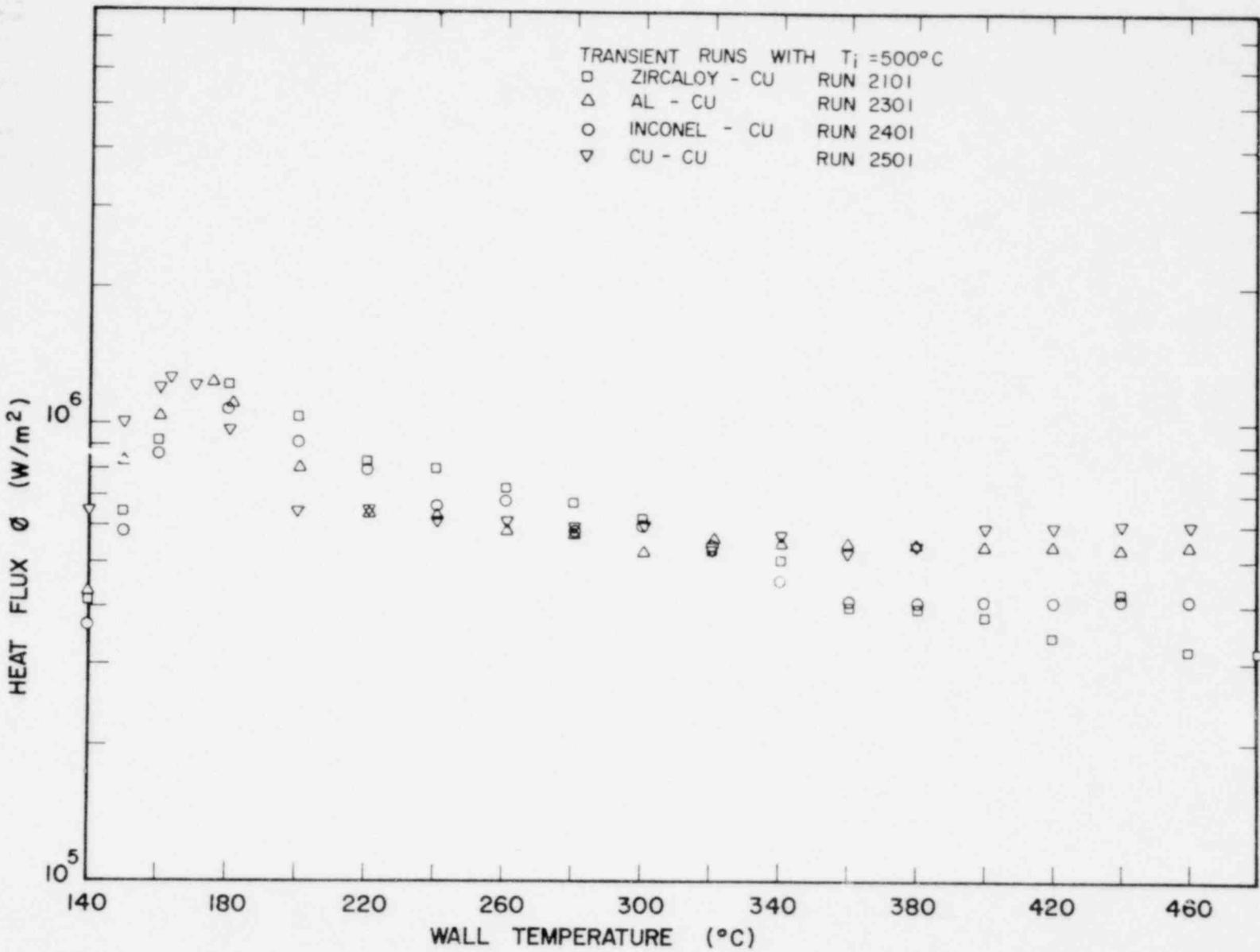
Fig. 14. Comparison of Boiling Curves for Various Heated Surfaces at  $G = 136 \text{ kg/m}^2\text{s}$  and  $\Delta T_{\text{sub}} = 13.9^\circ\text{C}$ , Using 1-D Model
