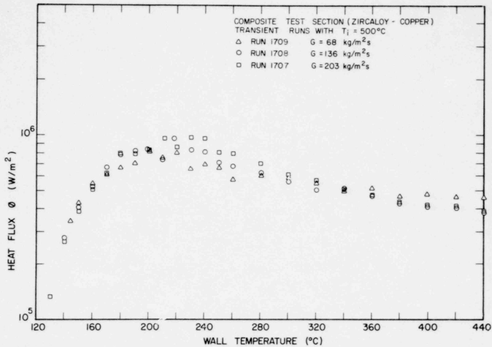
Fig. 10. Boiling Curves for Distilled Water, 1700 Run Series for  $\Delta T_{\text{sub}} = 0^\circ\text{C}$
