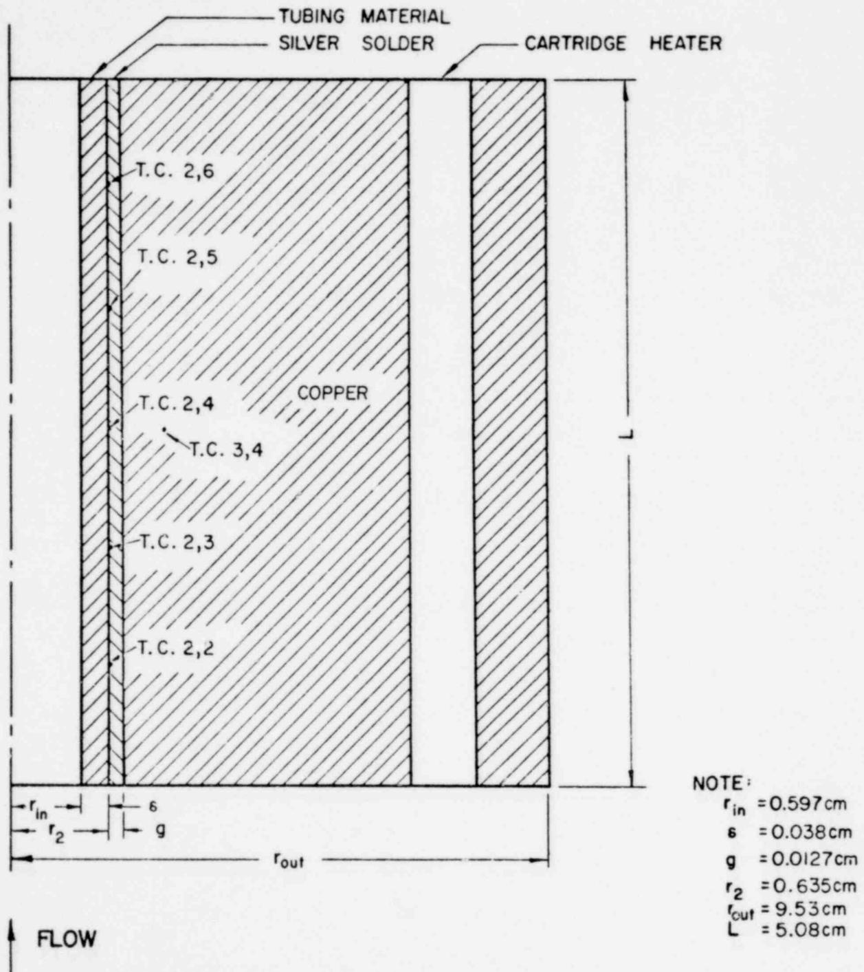
Fig. 1. Location of Thermocouples in Inconel-Copper Composite Test Section
