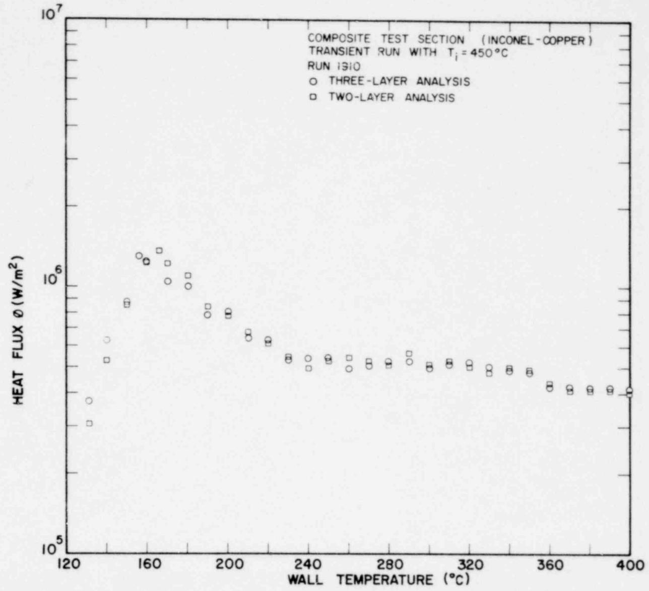
Fig. 11. Comparison of Boiling Curves for Three-layer and Two-layer Analyses, 1900 Run Series for  $G = 136 \text{ kg/m}^2\text{s}$  and  $\Delta T_{\text{sub}} = 13.9^\circ\text{C}$
