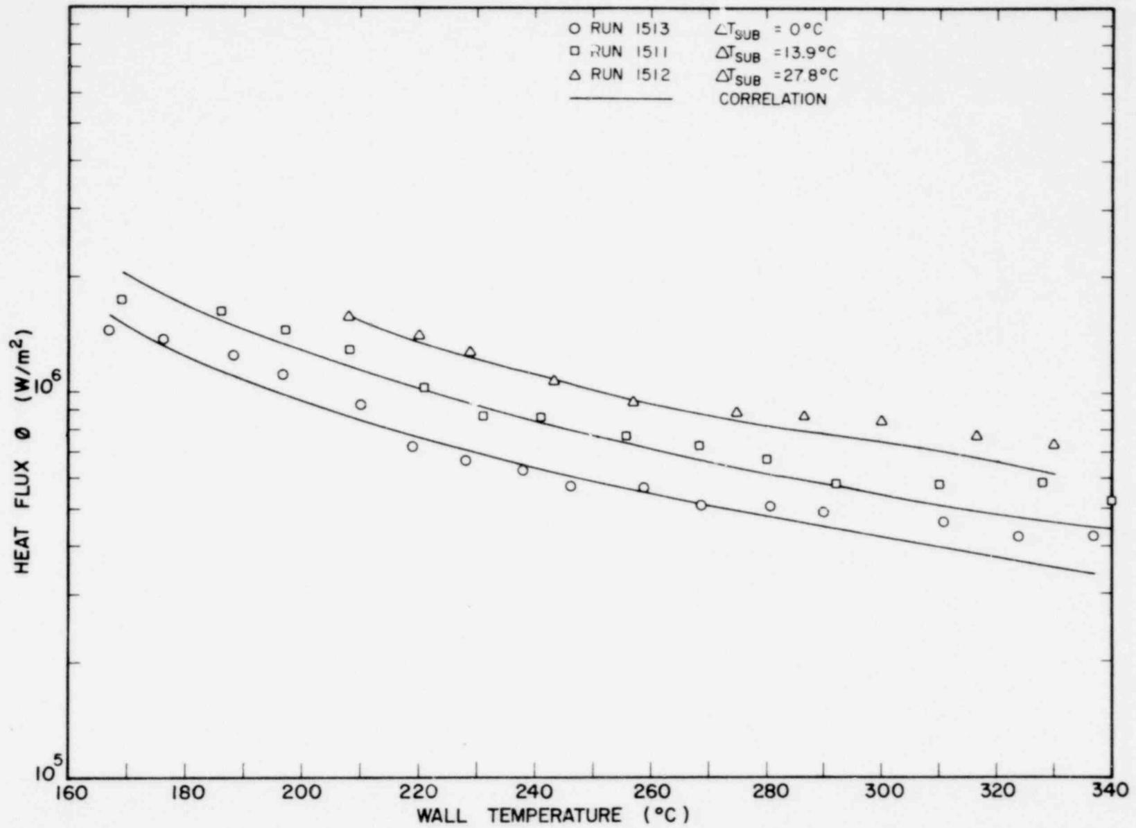
Fig. 24. Comparison of General Empirical Correlation with Inconel Data for  $G = 68 \text{ kg/m}^2\text{s}$
