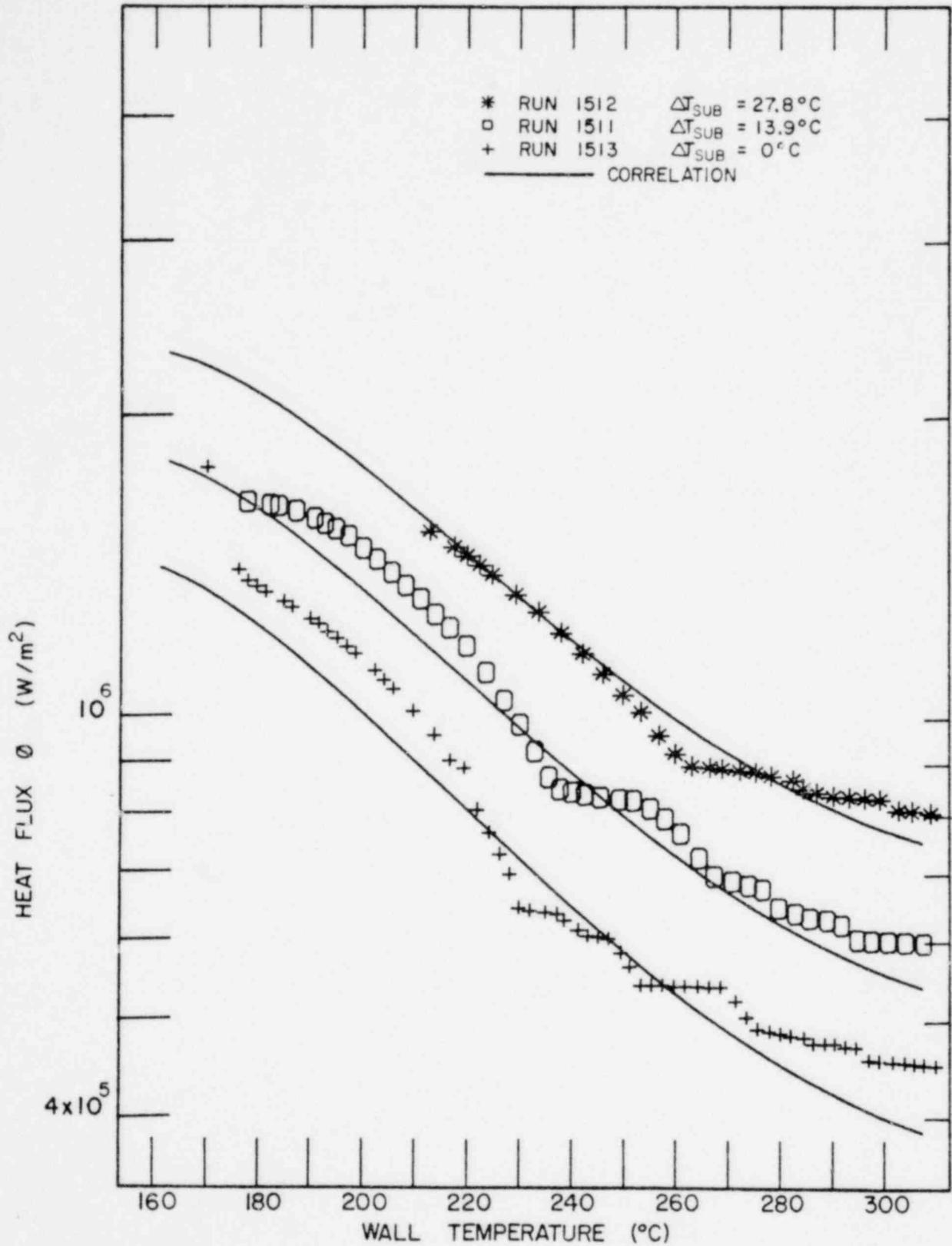
Fig. 20. Comparison of Inconel Correlation with Transition Boiling Data for  $G = 68 \text{ kg}/\text{m}^2\text{s}$
