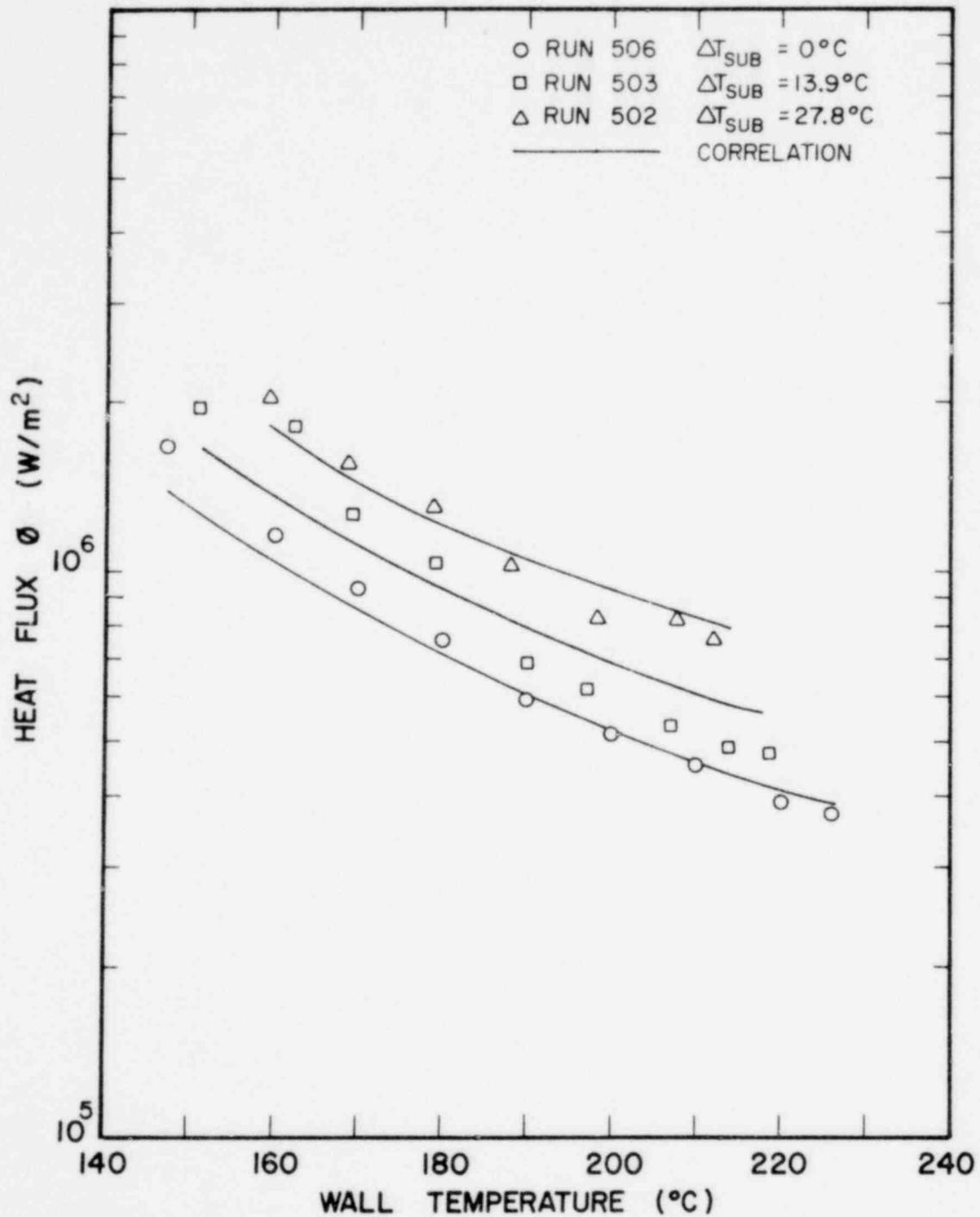
Fig. 23. Comparison of General Empirical Correlation with Copper Data for  $G = 136 \text{ kg/m}^2\text{s}$
