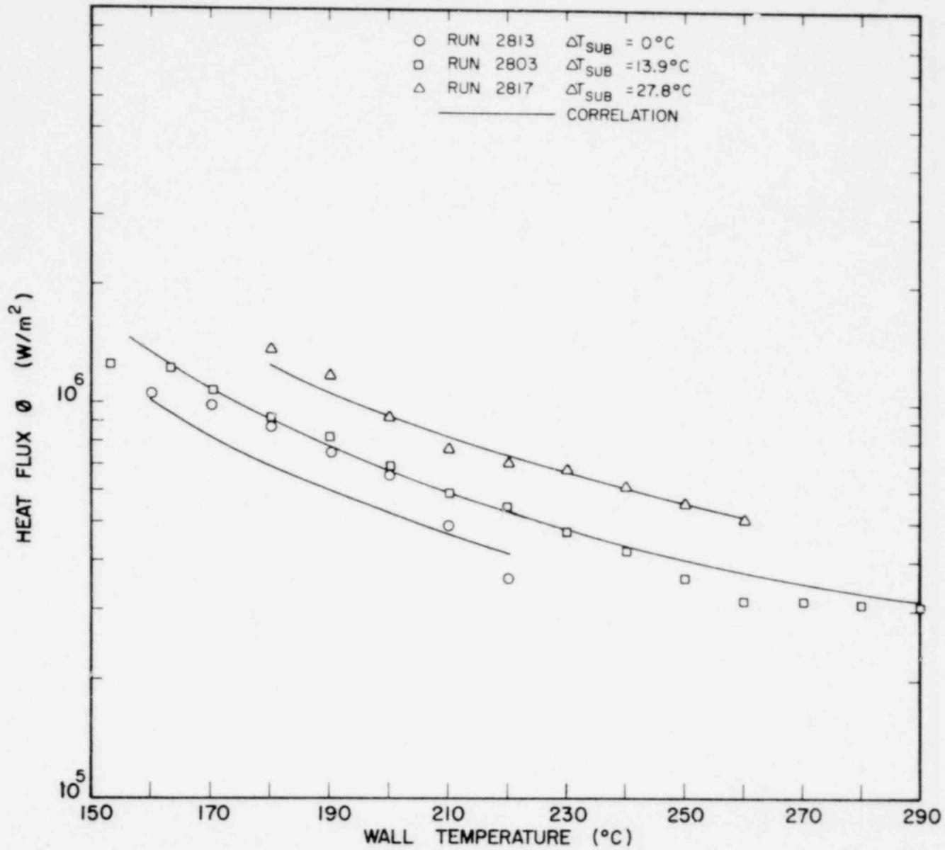
Fig. 25. Comparison of General Empirical Correlation with Brass Data for  $G = 68 \text{ kg/m}^2\text{s}$
