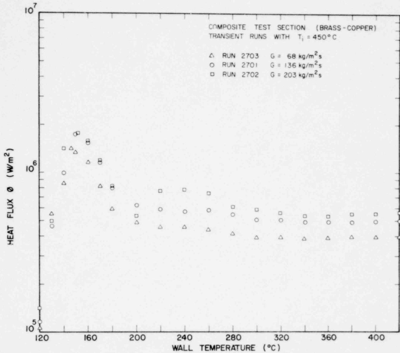
Fig. 15. Boiling Curves of Distilled Water, 2700 Run Series for  $\Delta T_{\text{sub}} = 13.9^\circ\text{C}$
