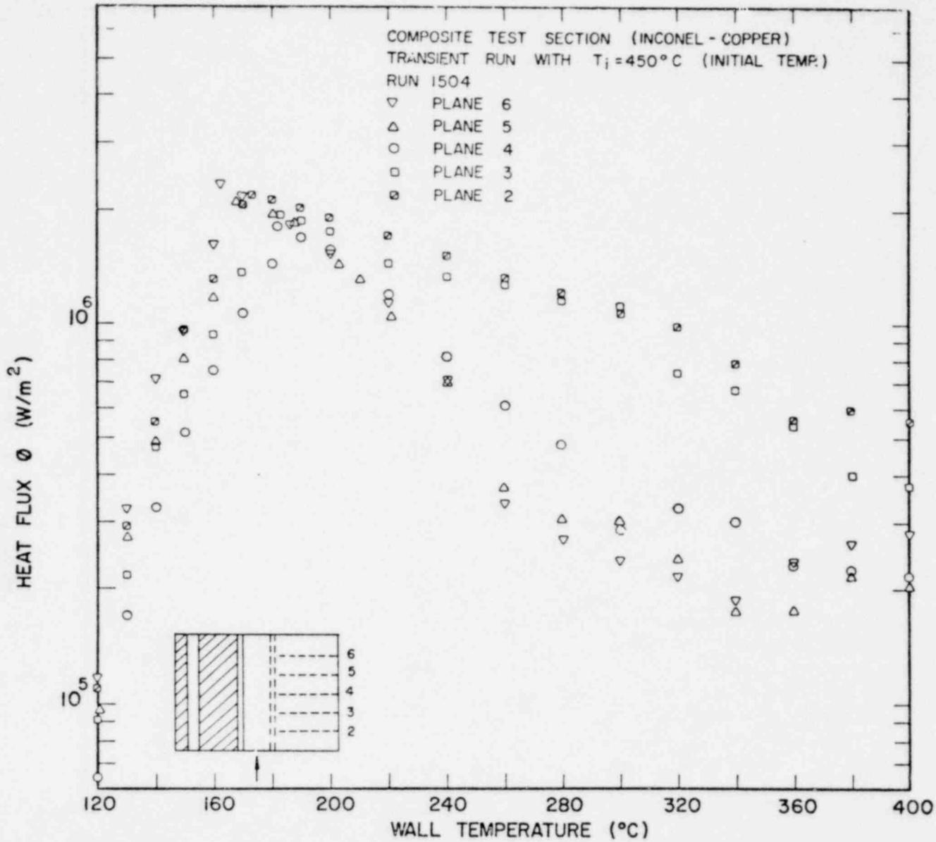
Fig. 3. Boiling Curves of Distilled Water, 1500 Run Series for  $G = 136 \text{ kg}/\text{m}^2\text{s}$  and  $T_{\text{sub}} = 13.9^\circ\text{C}$ , Using 2-D Model
