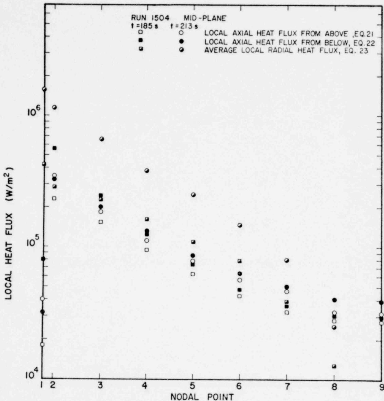
Fig. 4. Local Axial Heat Flux Distribution at Mid-Section for Inconel-Copper Composite Test Section for  $G = 136 \text{ kg/m}^2\text{s}$  and  $\Delta T_{\text{sub}} = 13.9^\circ\text{C}$  (Part I)
