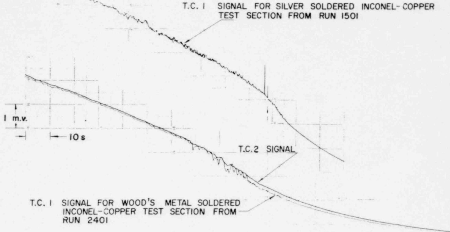
Fig. 16. Thermocouple Recordings from Silver Soldered Inconel-Copper Test Section and Wood's Metal Soldered Inconel-Copper Test Section
