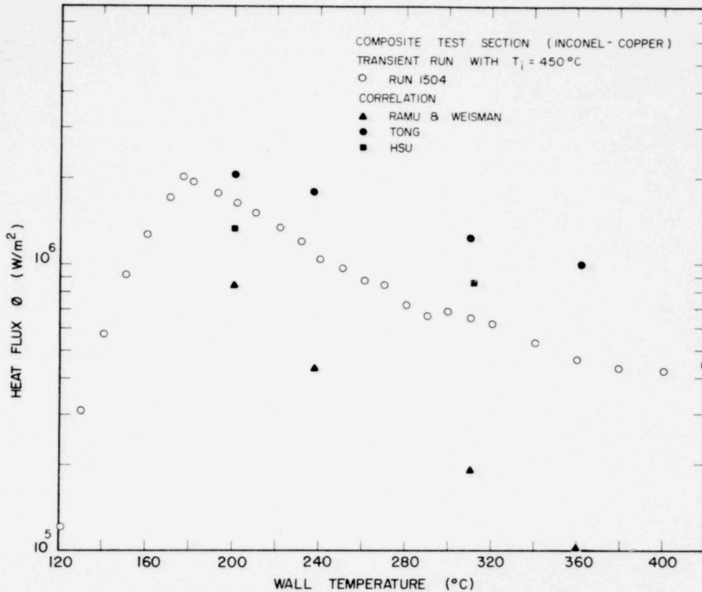
Fig. 18. Comparison of Data for 1500 Run Series with  $G = 136 \text{ kg/m}^2\text{s}$  and  $\Delta T_{\text{sub}} = 13.9^\circ\text{C}$
