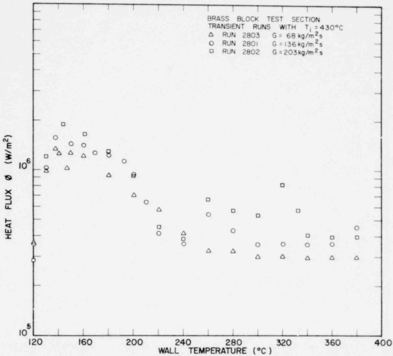
Fig. 21. Boiling Curves of Distilled Water, 2800 Run Series for  $\Delta T_{\text{sub}} = 13.9^\circ\text{C}$
