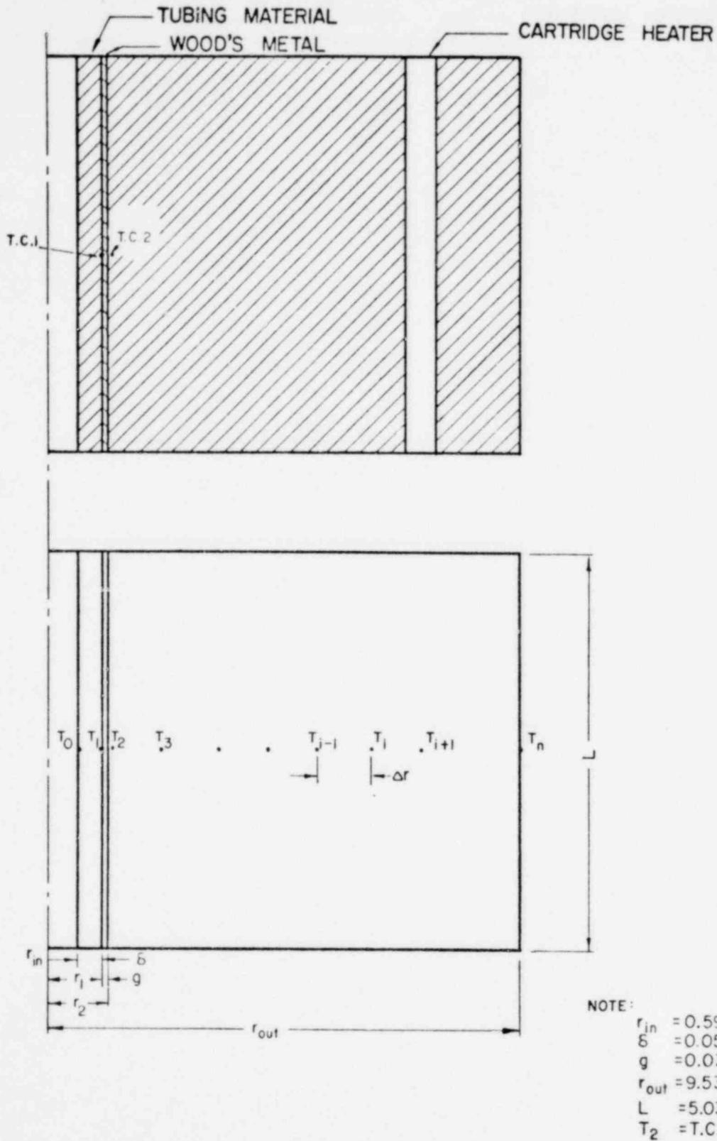
Fig. 6. Zircaloy-Copper Composite Test Section and Its Model Point Distribution
