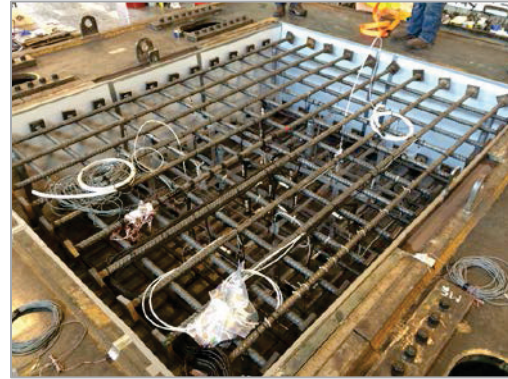
FIGURE 3. (a) Confined thick concrete specimen design. (b) Picture of rebar frame and steel frame for confined concrete specimen.
