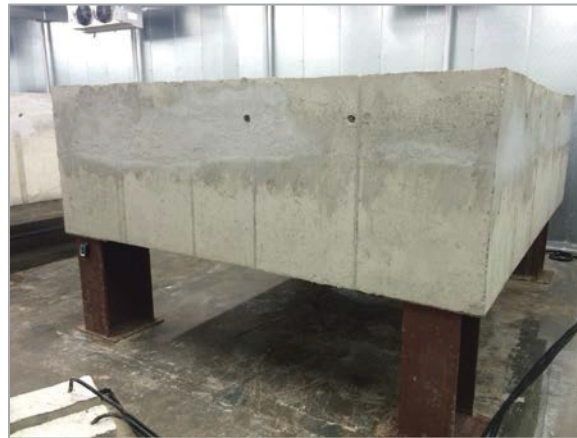
FIGURE 2. Picture of one of the unconfined concrete specimen inside the environmental chamber.
