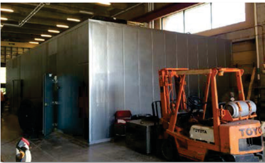
FIGURE 5. (a) Picture of the environmental chamber built around the concrete specimen. (b) Drawing of environmental chamber design.
