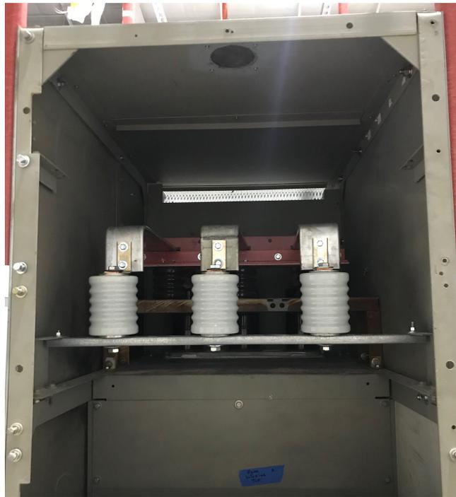
KEMA HEAF test switchgear
