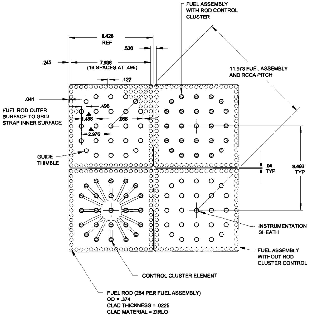
NOTE: THIS SECTION VIEW IS TAKEN AT THE TOP GRID ELEVATION
