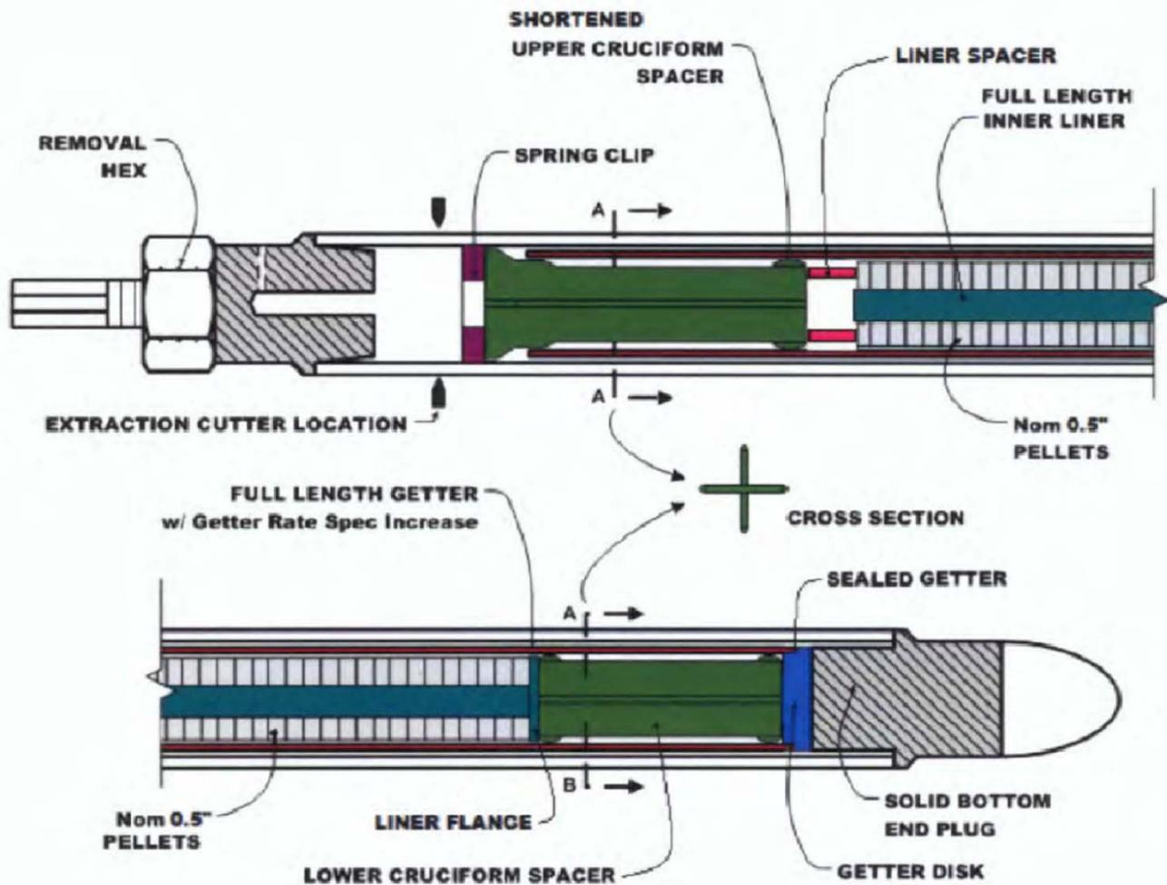
LU TPBAR Design: Full length inner liner with 1/2 inch pellets and sealed getter
